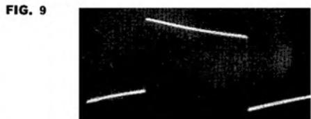
sloping top and bottom indicates a falling response at the lower frequencies.
