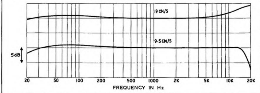
FIG. 4 REVOX A77 ACOUSTIC RESPONSE (WHITE NOISE TAPE TO SOUND OUTPUT)
