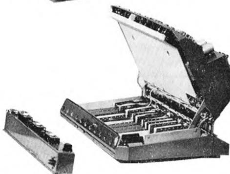
Fig. 5—Preamp circuits are accessible behind the screen and are built on hinged *Formica* cards. Similar cards in the plinth section plug in via *Bulgin* connectors.
