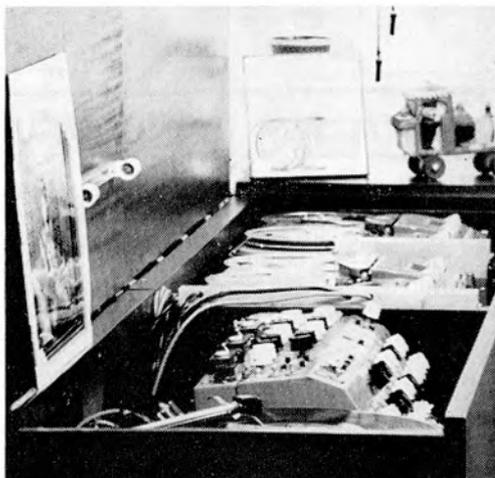
Fig. 2—Potentiometers for mixed feeds A and B are on top, C and D being to the right of the bass and treble controls.
