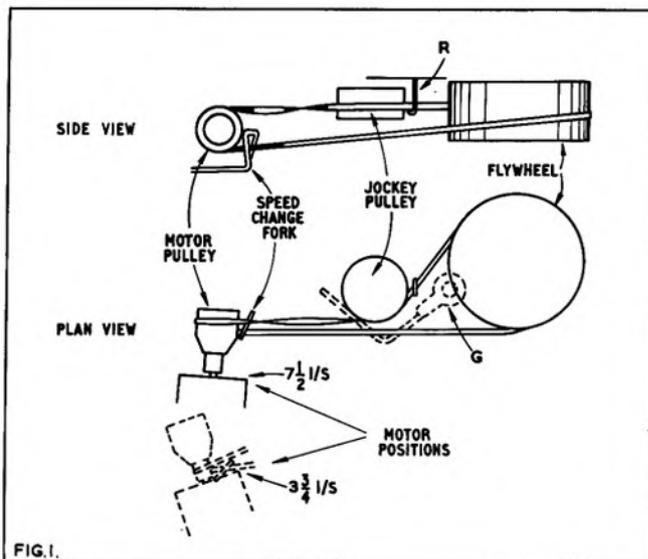
which should be slack when disengaged. A screw threaded through a spring allows pressure adjustment.
