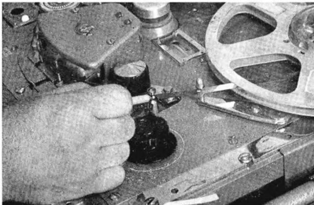
*Above: If the playback head is inaccessible, the chinagraph mark can be made alongside a convenient guide; the distance from head to guide enables calculation of the cutting position. Photo on page 397: Daphne Oram, composer of musique concrète, makes full use of splicing techniques to produce the unearthly from everyday sounds. Both illustrations by courtesy of the BBC.*
