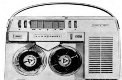
**Manufacturer's Specification. Power supply:** A.C. 40-60 c/s 110-220 v, 6 v car battery, 12 v using series resistance LR412, 5 U2 torch cells, 5 DEAC rechargeable cells type RS3.5. **Recording procedure:** double track international standard. **Tape speed:**  $3\frac{3}{4}$  i/s. **Frequency response at radio output:** 50-10,000 c/s. **Dynamic range:** 46 dB or better. **Maximum reel diameter:**  $4\frac{1}{2}$  in.
