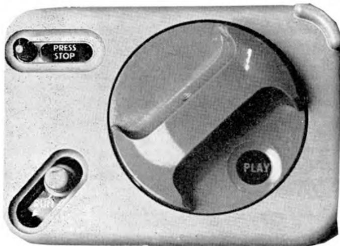
**Fig. 2:** Close-up view of the grouped operating controls. The main function switch has four positions, Record, Wind on, Wind back, and Play. In the Wind positions, the pressure pads are held away from the heads to prevent wear and facilitate tape loading.
