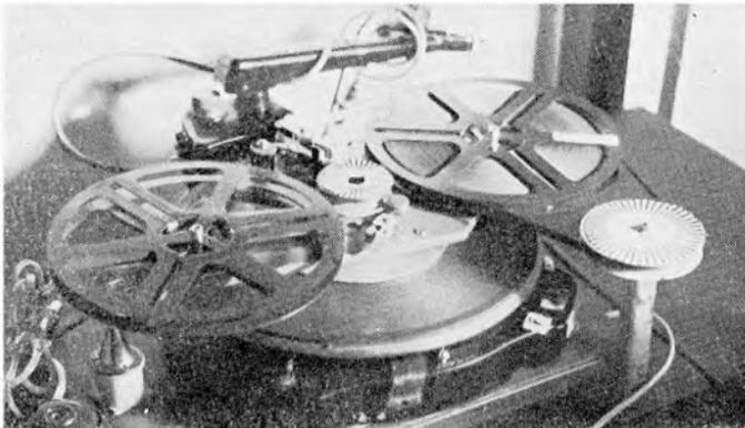
The writer of this letter enclosed the above photograph which illustrates the use of a Gramdeck unit and an old-fashioned gramophone. The sound track can be set to keep in sync. with a fixed speed projector. The stroboscope is driven by the tape and lit by the projector flicker.
