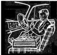
Valradio converters step up the DC voltage from your car battery enabling you to make your tape recorder really mobile.
