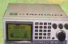
The only base scanner on the market with panoramic display at a realistic price, enabling the user to view a whole 1MHz on the built in brightly lit LCD TV type screen.
