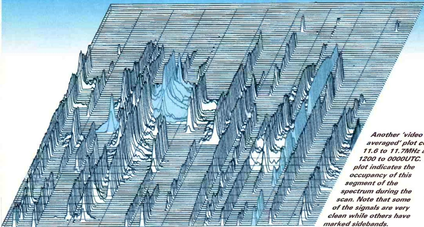
*Another 'video averaged' plot covering 11.6 to 11.7MHz and 1200 to 0000UTC. This plot indicates the occupancy of this segment of the spectrum during the scan. Note that some of the signals are very clean while others have marked sidebands.*
