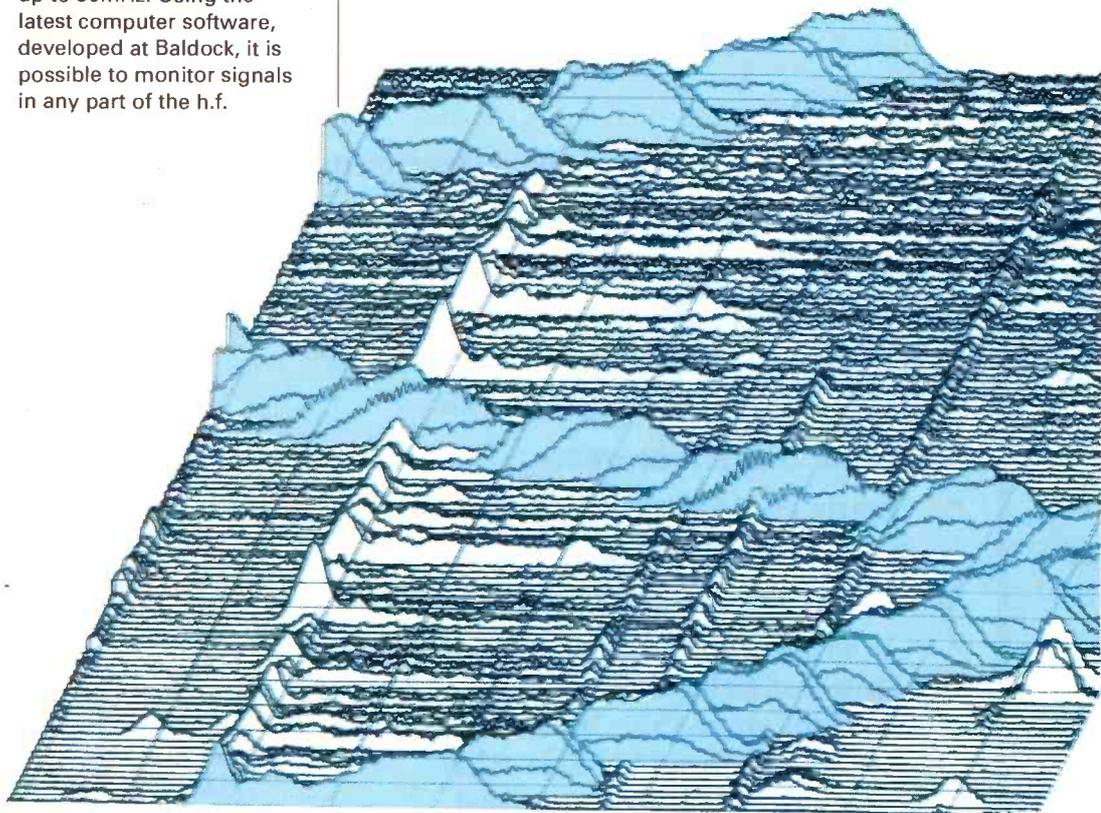
*This very striking plot shows a transmitter drifting across the portion of the spectrum being monitored. This information can be used by the Radiocommunications Authority to identify rogue stations and get something done about them. This is a 'video averaged' plot. The drifting signal has been coloured by SWM to make it stand out better. The time scale of the complete plot is six hours, while the frequency span is 2.18 to 2.19MHz.*
