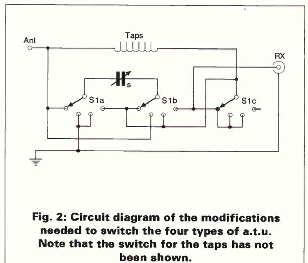
the a.t.u. and wire it so that all four options shown in **Fig. 1** would be available at the twist of a knob. A suitable switch would be Maplin
