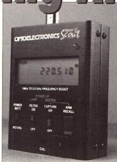
indication, a red 'gate' l.e.d., three small slide switches for power, filter and capture functions and a square push-button to select the 'gate' time. The top panel has a d.c. power socket, red
