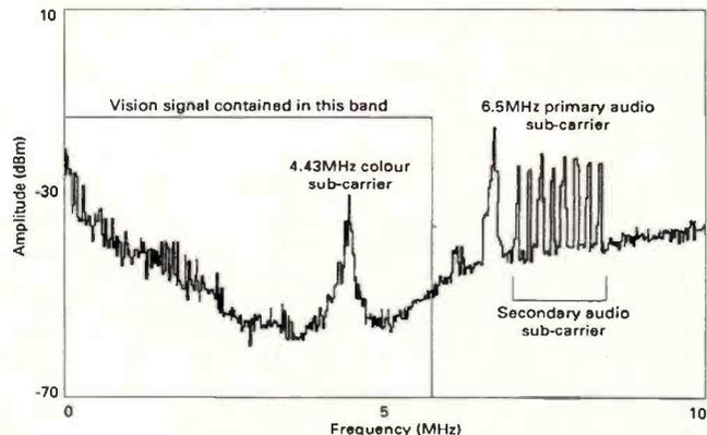
Fig.1: Typical spectrum of satellite TV baselband signal.
