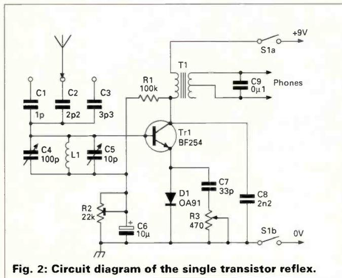
Fig. 2: Circuit diagram of the single transistor reflex.
