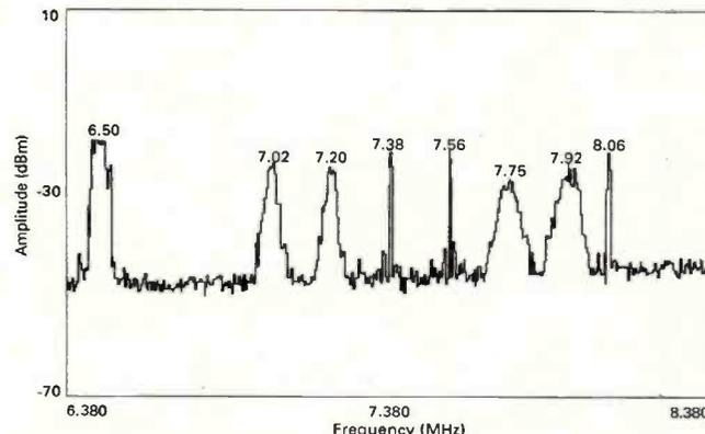
Fig.2: Magnified portion of spectrum showing individual audio subcarriers.
