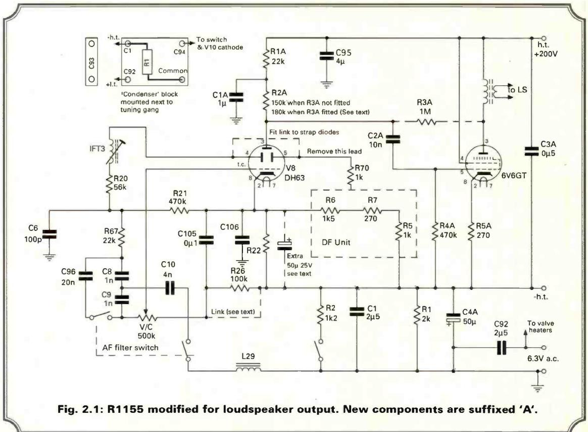
Fig. 2.1: R1155 modified for loudspeaker output. New components are suffixed 'A'.
