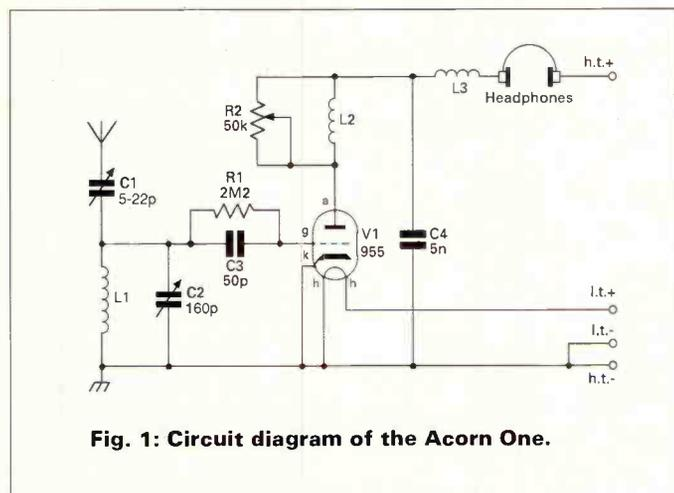
**Fig. 1: Circuit diagram of the Acorn One.**
