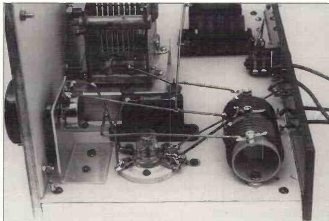
the lower glass 'pip' of the acorn valve projects below the level of the holder base, so a hole must be drilled in the baseboard to accommodate this 'pip'.
