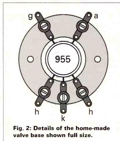
**Fig. 2: Details of the home-made valve base shown full size.**
