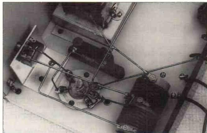
**Fig. 5: Details of the valve and coil wiring.**
