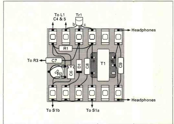
**Fig. 4: The main component tag board sub-assembly. Shown full size.**
