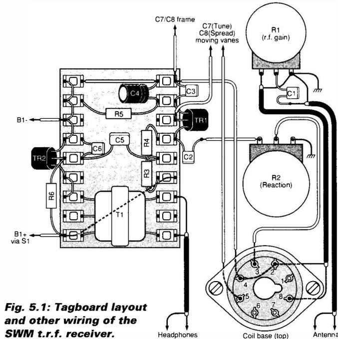
**Fig. 5.1: Tagboard layout and other wiring of the SWM t.r.f. receiver.**
