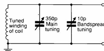
(b): Adding bandspreading by electrical means.
