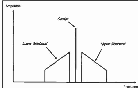
Fig. 1: An a.m. signal.
