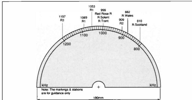
Fig. 1: How to mark out the dial.
