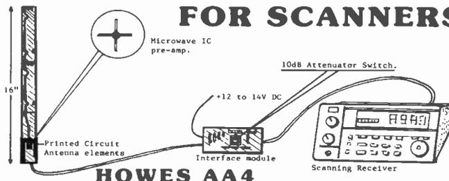
The **HOWES AA4** Active Antenna gives full coverage from 25 to 1300MHz. It is designed to be the ideal solution for those requiring a compact, broadband antenna for use with scanning receivers. The AA4 features advanced technology with a low noise microwave IC amplifier.
