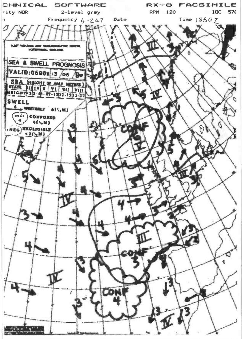
Fig. 2: Weather map from Northwood on 4.247MHz at 1850Z.
