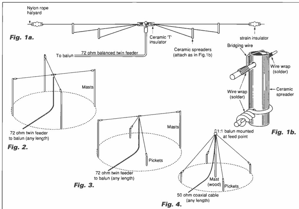
last month's article. If space permits, additional masts can be used to support the ends of the dipoles added to the feed-point. Two dipoles erected in that manner are depicted in **Fig. 2**. This method offers the advantage that each dipole can be erected in a direction best suited for optimum reception from a particular area.
