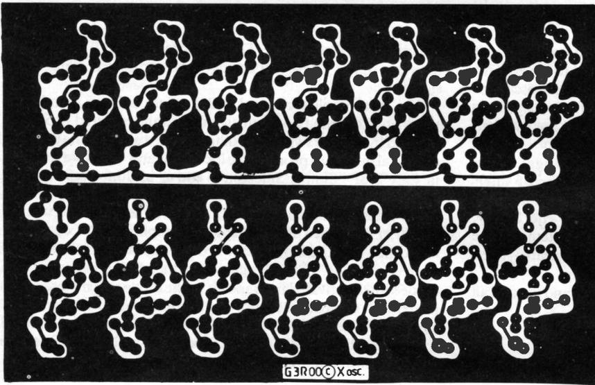
Fig. 4. Oscillator PCB foil
