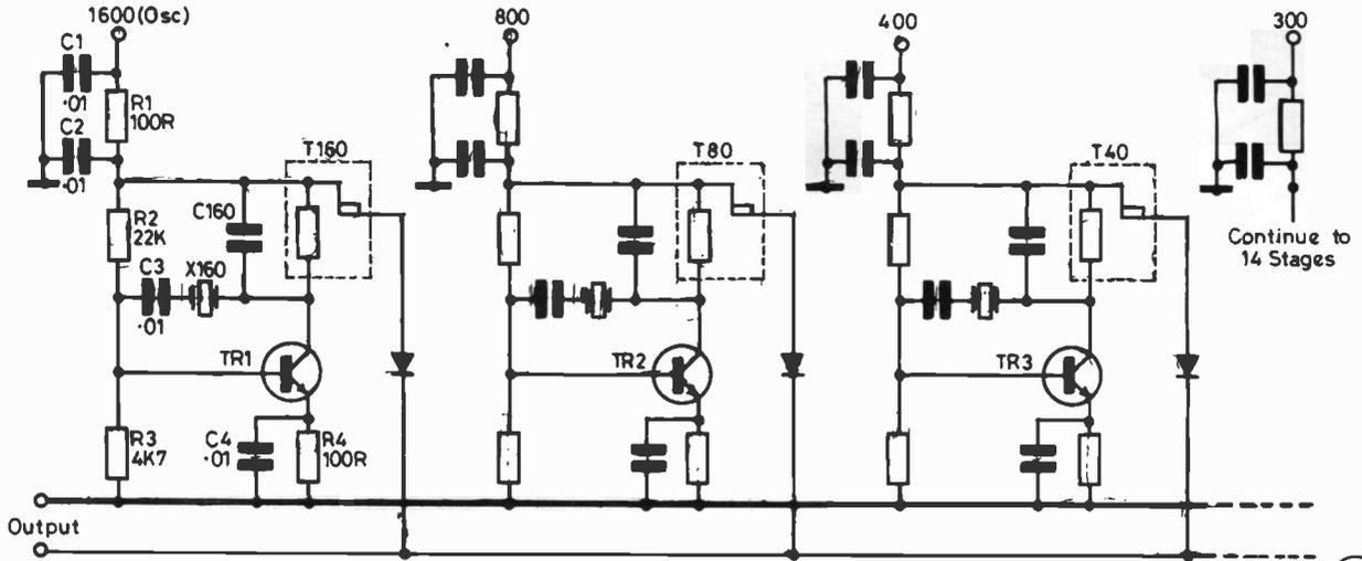
Fig. 3 MODULAR SSB TRX 14 CHANNEL OSCILLATOR CIRCUIT DIAGRAM
