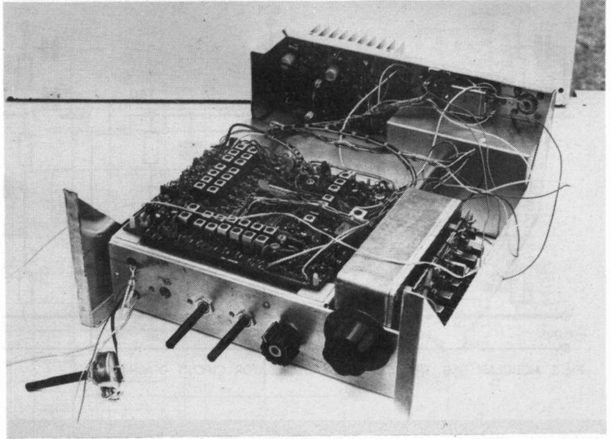
board that we have to build before we start is an oscillator unit that can provide a signal for each band we intend to cover. This will mix with the VFO to produce the required local oscillator signal for the transceiver mixer; this mixing of the two signals is done on the '707 RF board and the necessary filters are switched with the signal frequency circuits.
