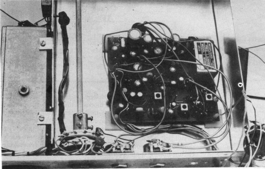
The MLX PCB. Note the bandswitch (bottom left) with extension spindle to the LPF box. The VFO box is on the left
