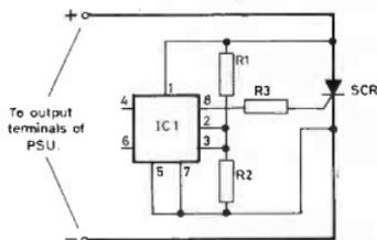
Note: Heavy wires to SCR should be at least 2.5mm<sup>2</sup> and be as short as possible.
