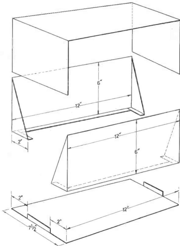
Fig 22 WHITFIELD CASE DETAILS (16 swg Aluminium)
