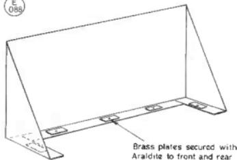
Fig 23 "WHITFIELD" BRASS PLATE POSITIONING
