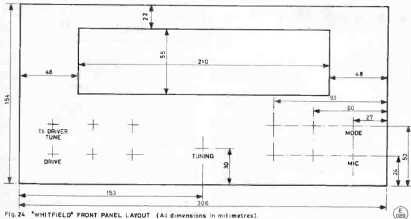
Fig. 24 'WHITFIELD' FRONT PANEL LAYOUT (All dimensions in millimetres).
