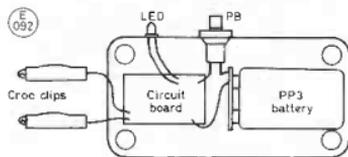
Fig 3 CRYSTAL CHECKER LAYOUT IN PLASTIC BOX
