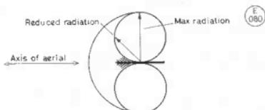
Fig 1(a) '3D' Polar diagram of horizontal dipole in free space. The actual 'doughnut' pattern is cut in half to show how the line from the centre to the surface of the pattern varies.
