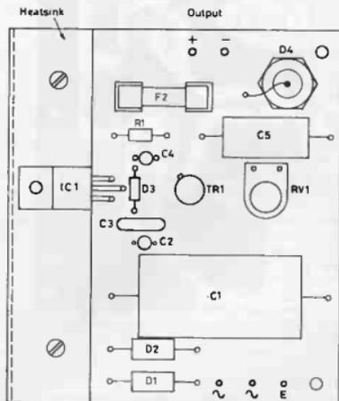
Fig. 3 PCB LOCATION OF COMPONENTS (Full size).
