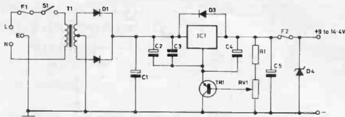
Fig. 1 LOW CURRENT POWER SUPPLY CIRCUIT DIAGRAM
