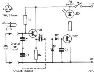
Fig 1 CRYSTAL CHECKER CIRCUIT DIAGRAM
