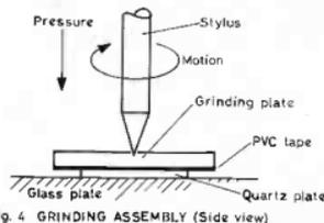
Fig 4 GRINDING ASSEMBLY (Side view)
