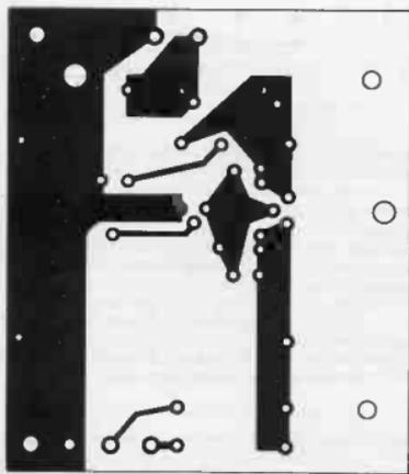
Fig. 2 PCB TRACK LAYOUT (Full size).
