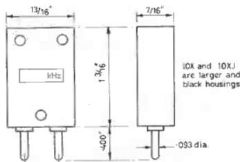
Fig. 6 FT 243 PRESSURE MOUNTING
