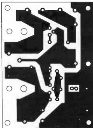
Fig. 5 PCB TRACK LAYOUT (Full size)
