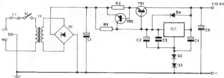
Fig. 4 5AMP POWER SUPPLY CIRCUIT DIAGRAM
