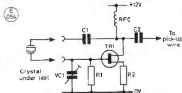
Fig. 5 CRYSTAL TEST CIRCUIT (For 2-20MHz fundamental pressure mounted crystals - recommended by 'JAN Crystals')
