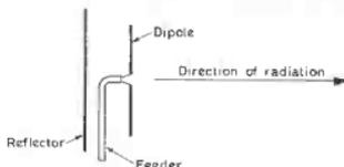
Fig. 3(a) DIPOLE PLUS REFLECTOR
