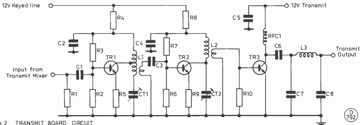
Fig. 2 TRANSMIT BOARD CIRCUIT
