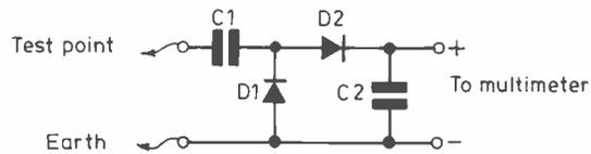
Fig. 8 DIODE RF PROBE
