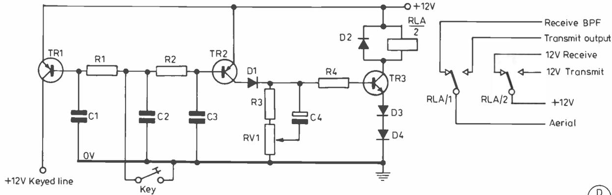
Fig.3 CHANGEOVER CIRCUIT
