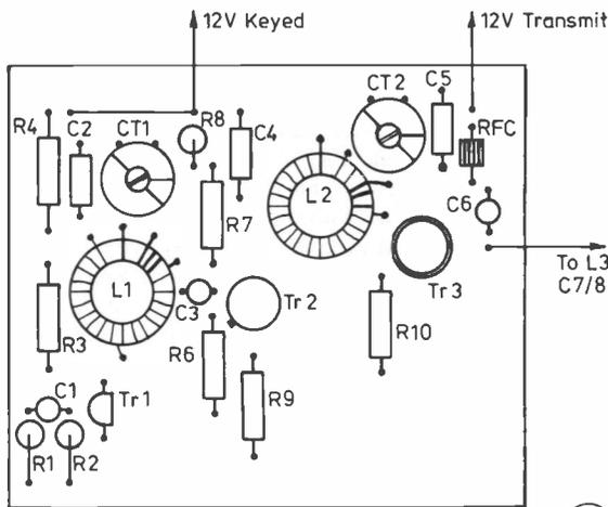
Fig. 5 TRANSMIT BOARD LAYOUT (actual size).
