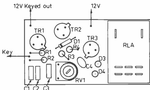
Fig. 6 CHANGEOVER CIRCUIT BOARD (actual size).
