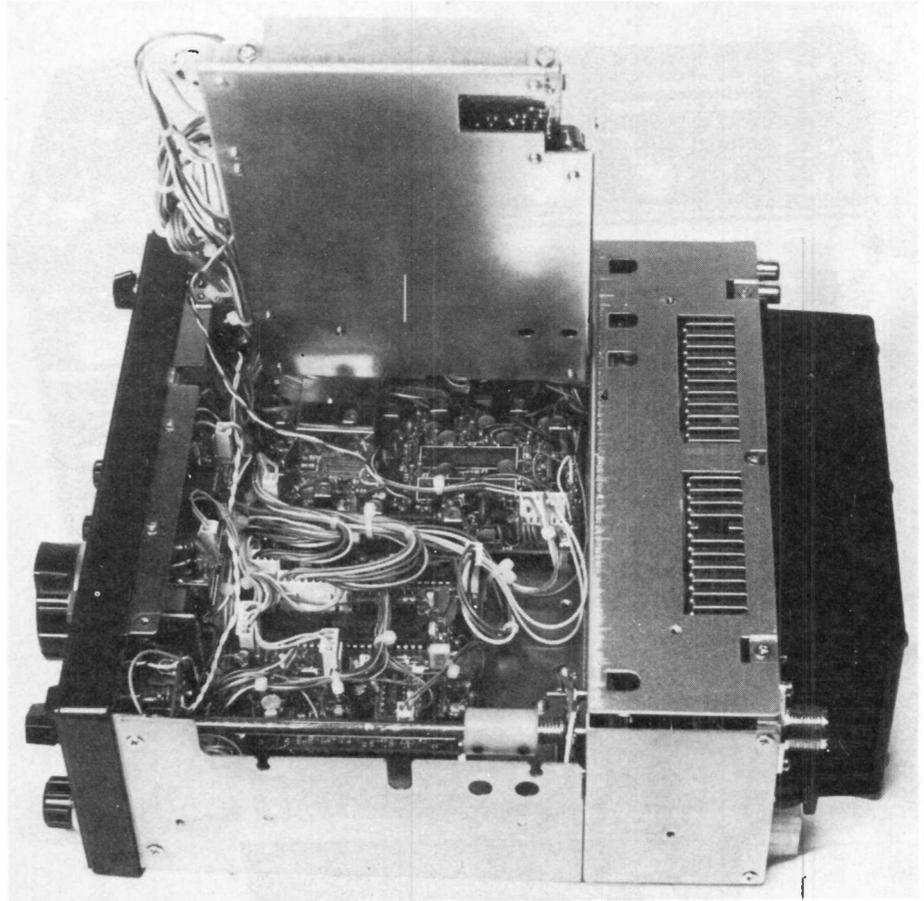
band,  $30\mu\text{V}$  gave an S9 indication,  $180\mu\text{V}$  S9 + 20 dB,  $910\mu\text{V}$  S9 + 40 dB and  $15\text{mV}$  S9 + 60 dB. This corresponds to steps of 15.6, 14.1 and 24.3 dB respectively. The gain of the preamplifier stage averaged out at 9.5 dB.
