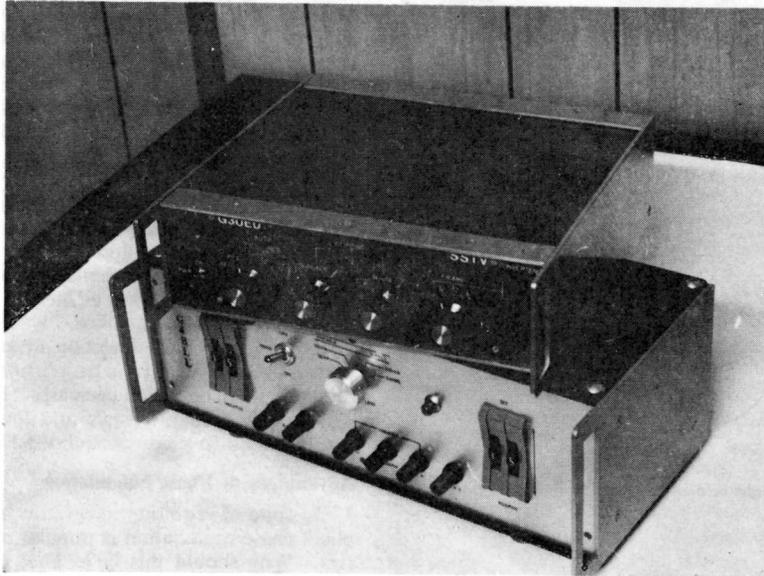
Shows two pieces of home constructed equipment using the described Cabinet System. The top one is a SSTV fast/slow converter and shows how front and rear trims may be fitted to enhance the appearance. The bottom piece of equipment is a fully variable "digital readout" power supply with current limiting and short-circuit protection.
