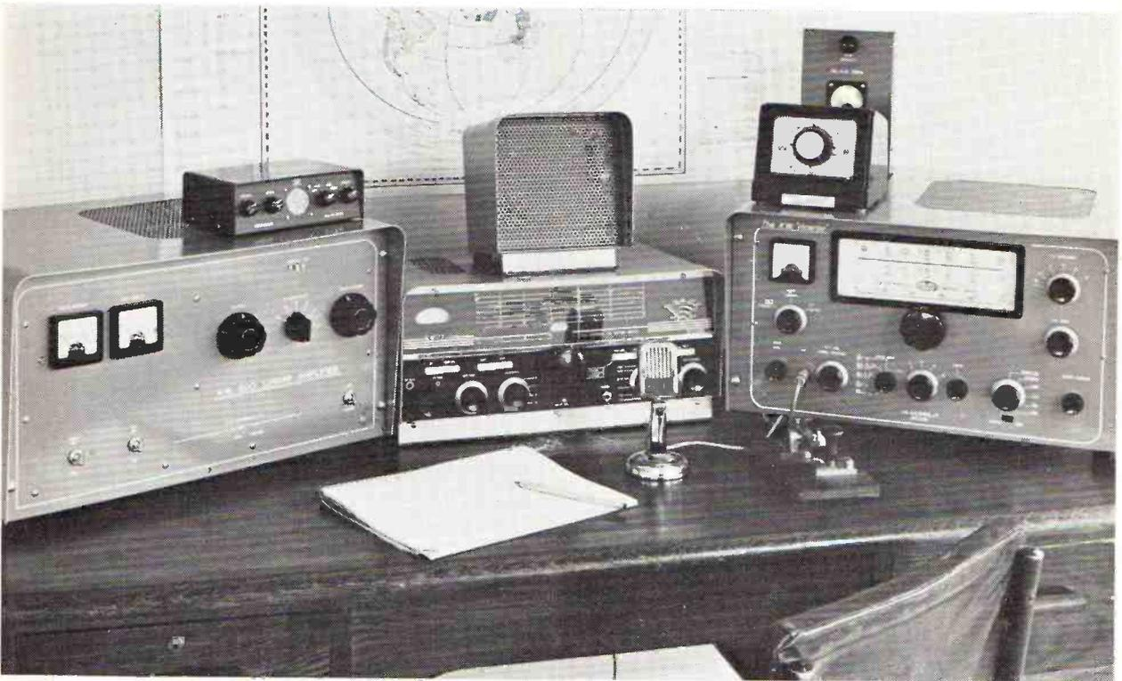
The KW Station comprising (left to right) KW 500 Linear Amplifier, Hammarlund HK1B Electronic Keyer, KW 77 Triple-Conversion Receiver and Speaker, Gelo-Table mic., KW Viceroy transmitter, CDR Beam Control Unit, KW Match SWR indicator (Vibroplex bug-key and 'phones in desk drawer).
