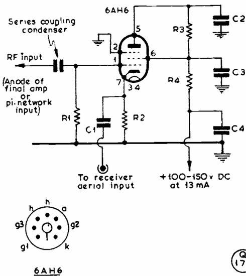
Fig. 5. A transmitter tank T-R switch. Such a unit should be mounted in a screened box, with the valve also screened; all leads to the receiver and external power source must be fully screened, too. Values are: C1, C2, C4, .01  $\mu\text{F}$ ; C3, .001  $\mu\text{F}$ ; R1, 1.2 megohms; R2, 220 ohms; R3, 1000 ohms; and R4, 270 ohms. Resistors can be all 1/2-watt non-inductive, and the condensers the disc ceramic type.
