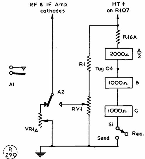
Fig. 3. Suggested muting and control circuit—see text. A/2 is the existing relay in the IF pack; B is external HT control relay; C the external aerial c/o relay; S1 is the send-receive switch; VR1A the existing RF gain control; R1 is 200,000 ohms, 1-w.; R2 is a 50,000-ohm potentiometer; and R16A is the existing 15,000-ohm 3-watt resistor.
