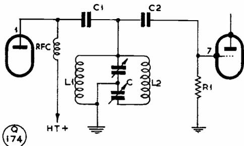
Fig. 4. A modification of the twin-triode T-R switch which will improve the gain and add selectivity to the original circuit. Condenser C is approximately 400  $\mu\mu\text{F}$  per section, and can be a split-stator receiving type. C1 is 150  $\mu\mu\text{F}$ ; C2, .001  $\mu\text{F}$ ; R1, 50,000 ohms; RFC, 21  $\mu\text{H}$ , as in Fig. 3; L1, 19 turns 18g. on 1-in. diam. former, spaced to 5/8-in.; L2, 23 turns 18g. on 1/2-in. diam. former spaced out to 1 1/2-ins. length.
