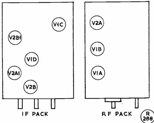
Fig. 1. Positioning of the valves on the IF and RF packs of the R.107 ex-Army receiver. These packs are obtainable separately as "surplus" items.
