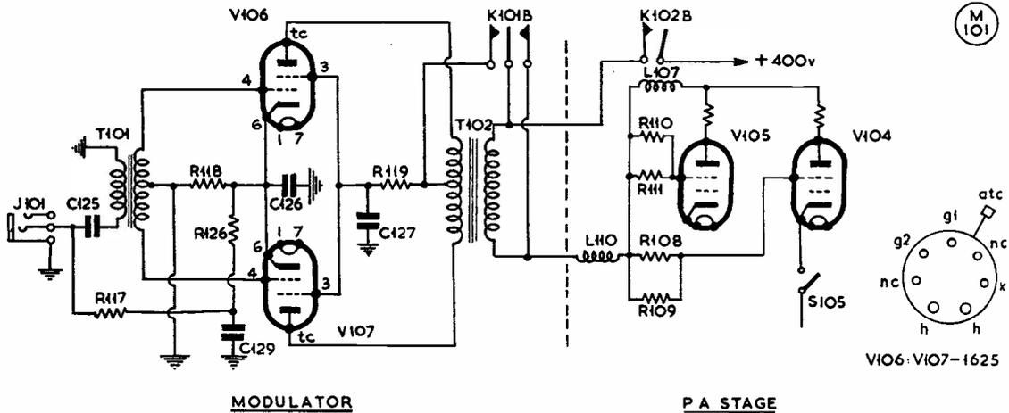
Fig. 3. Modulator arrangement in the TCS transmitter, using a pair of 1625's, V106/V107. As explained in the article, the speech output with a carbon microphone and the circuit as shown here leaves something to be desired, and it is better to drive the 1625's with a separate high-gain speech amplifier suitable for a crystal microphone.
