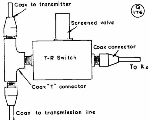
Fig. 6. Suggested constructional layout for the T-R switch shown in Fig. 5. The unit is fully screened and all RF lines are run in coaxial cable. The transmitter output is in effect connected through the T-R switch by means of the T-connector, making for short and direct RF leads.
