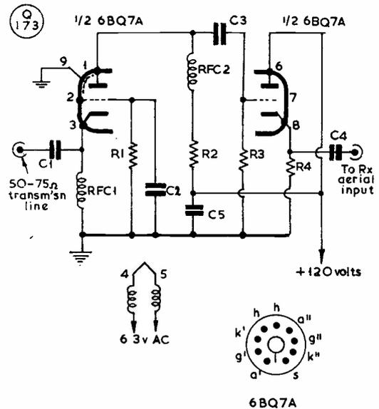
Fig. 3. A much more refined type of T-R switch, using a twin-triode. Values are: C1, 500  $\mu$ F; C2, C4, .01  $\mu$ F; C3, C5, .001  $\mu$ F; R1, 1 megohm; R2, 1000 ohms; R3, 50,000 ohms; R4, 100 ohms; RFC1, 2.5 mH; RFC2, 21  $\mu$ H (10-metre) RF choke; Htr. 4/5, bi-filar wound. All resistors are 1/2-watt non-inductive. RFC2 is a single-layer VHF-type RF choke, and is not critical; the special bi-filar choke, in the heater leads, is explained in the text.
