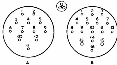
Receiver plug from the front. Transmitter plug from the front
