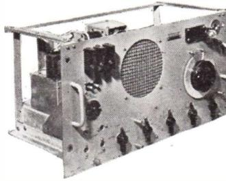
Complete with 6 valves, 2-6K8G, 2-EF39, 6Q7G and 6V6G. Internal mains and 6v. vibrator pack. Built-in 6 1/2" P.M. speaker. Muir-head slow motion drive. B.F.O. and R.F. stage. Provision for 'Phones and Muting and 600 ohms line combined input, 100/250v. A.C. or 6v. D.C. All sets in new condition and air tested.
