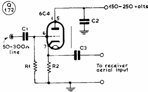
Fig. 2. A cathode-follower T-R switch. Resistors are 1-watt non-inductive, and the input and output circuits should be screened to prevent feed-through coupling. Values are: C1, 50  $\mu$ F, 500v.; C2, .005-.01  $\mu$ F; C3, .01  $\mu$ F; R1, 1 megohm; and R2, 500 ohms.
