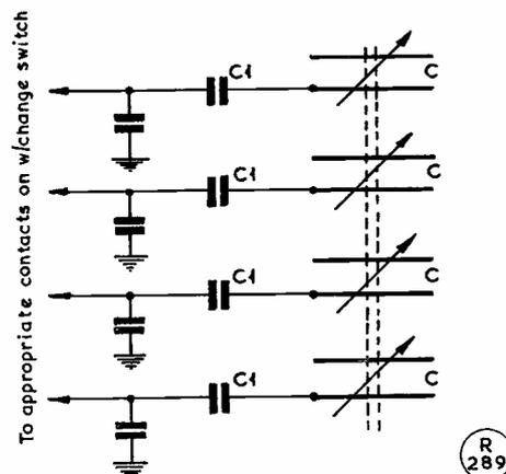
Fig. 2. Method of obtaining improved band-spread when using the R.107 RF/IF packs as part of a double superhet. Capacities marked C are the existing 300  $\mu$ F sections of the 4-gang tuning condenser, and those marked C1 are all 75  $\mu$ F 1% silver mica condensers.
