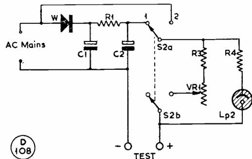
Fig. 1. The experimental layout for the Tester described in the text. This particular arrangement is not recommended for any finalised constructional form, because it is exposed to mains voltage. A better circuit, which is safer and gives the same sort of results, is shown in Fig. 2.
