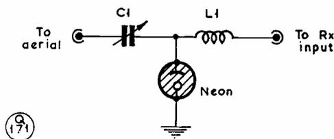
Fig. 1. A basic T-R (automatic send-receive) switch, using a series-resonant circuit and neon bulb. C1 is 50  $\mu$ F, and L1 is of 28g. on a  $\frac{1}{2}$ -in. diameter former, as follows: For 3.8 mc, 90 turns; for 7 mc, 45 turns; for 14 mc, 27 turns. The action of the circuit is explained in the text; it is applicable to any amateur Tx/Rx change-over situation.
