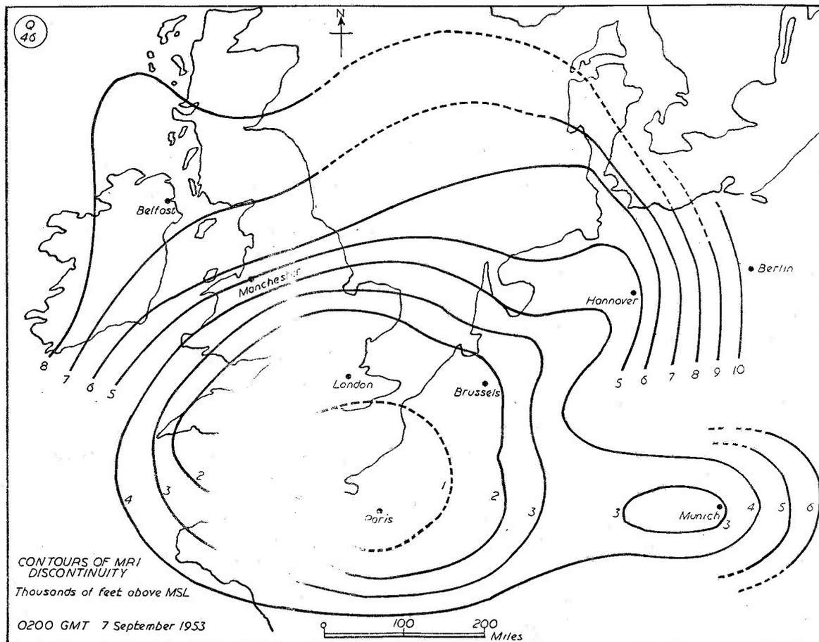
Fig. 2. Showing the contours (heights) of the MRI discontinuity (reflecting layer) that formed over part of Northern Europe early in September. From the heights given, it can be visualised rather as an irregular bowl, with the lip sloping upwards from the earth from a small, low-level central area. With the level central area well spread out, conditions are very much better.
