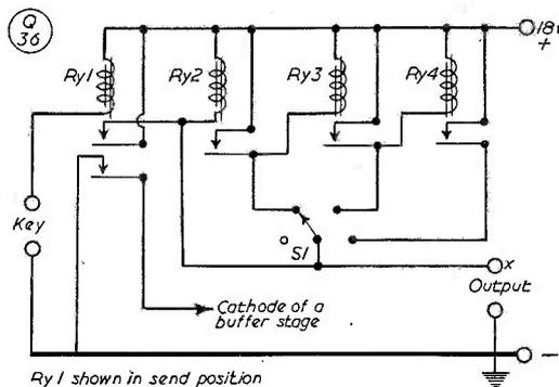
Fig. 1. Electrical layout of the key controlled circuit.
