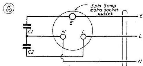
Fig. 7. Additional mains filter to be fitted at plug point. C1, C2 are  $2.0 \mu\text{F}$ , not less than 1000v. wkg. The lettering N, E, L, stands for "neutral, earth, live," and should appear on all plugs and sockets in properly-wired installations.
