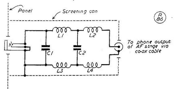
Fig. 3. Circuit of RF filter for phone output leads. L1-L4 are "all-wave" RF chokes, and C1, C2 are .001  $\mu$ F.
