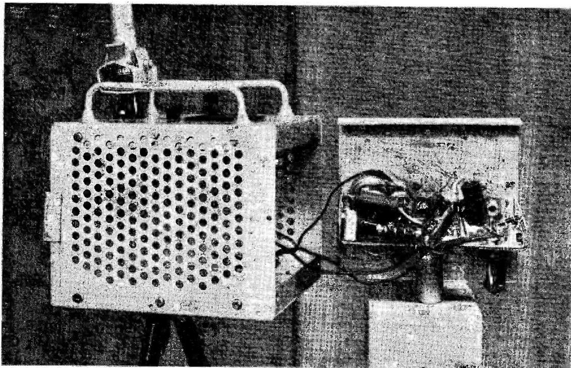
The field strength meter exposed, with its carrying case and tripod on the left. The telescopic mast extends to 7 feet; L1 is from a 1½v. dry cell and HT from 22½v. deaf-aid batteries. A shelf-type chassis is used, with parts fitted above and below. It was with this instrument that G2NS obtained the readings given in his article.
