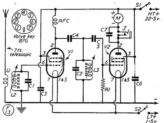
Fig. 1. Circuitry for a modern type of Field Strength Meter, sensitive enough for measurements to be made at some distance from the radiating system. Coils are for the band(s) required and values are given in the table. The built-up version of this circuit is shown in the photograph.
