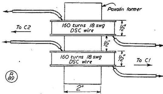
Fig. 6. Detail of the construction of 2.0 mH RF chokes for mains filtering.
