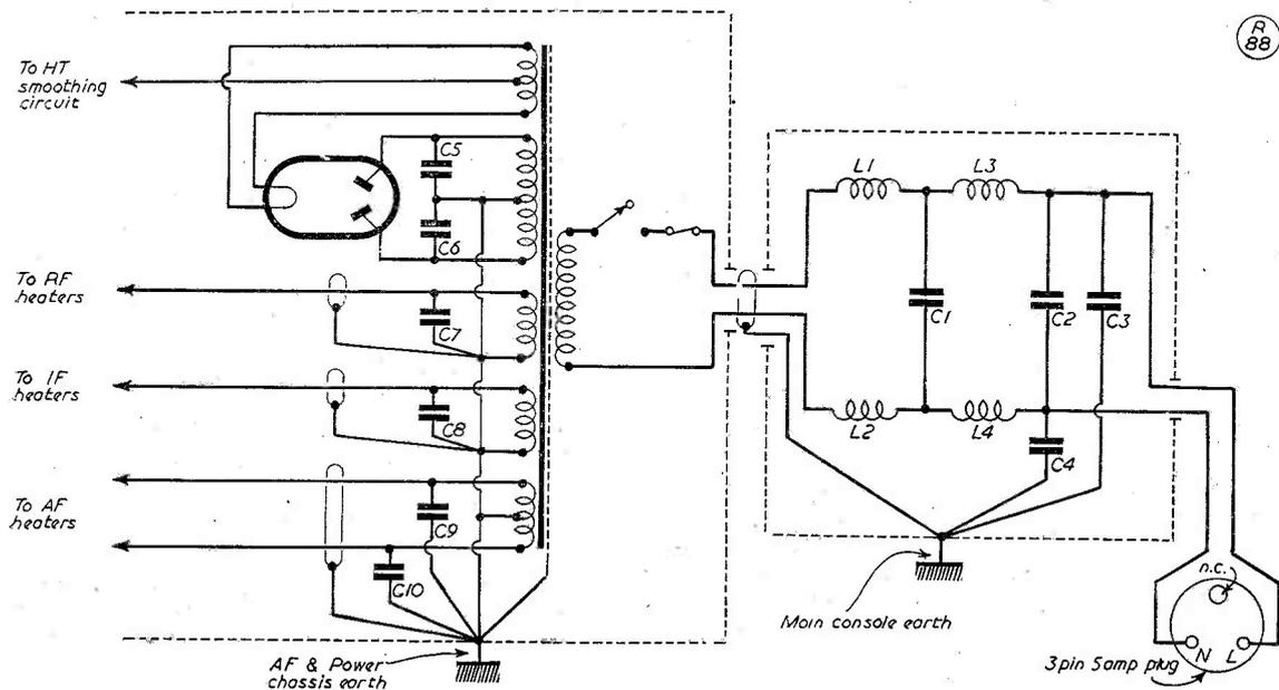
Fig. 5. Circuit of power pack and suitable mains supply filter for use with the idealised noise-free receiver.
