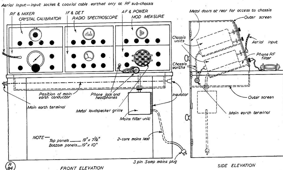
Fig. 1. Recommended layout plan for console-type receiver designed for noise-free operation. This is to show general arrangement only.
