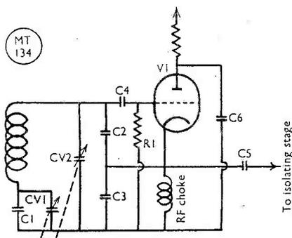
The circuit suggested by G2DCI to improve the performance of the Clapp over a wider band of output frequencies. CV1, CV2, are ganged to give constant capacity variation, and values are shown in the table.
