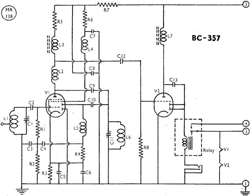
Circuit of the BC-357 before modification. All controls and connections are brought out to the front panel, and the whole unit measures 5½-in. × 5½-in. × 3¼-in. only
