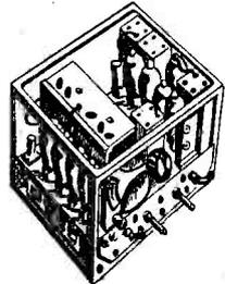
**RECEIVER TYPE 21.** These function as a superhet from 4.2-7.5 mc/s and as a double superhet from 18-31 mc/s. Complete with 9 2v valves, it may be used with its PU (previous item), directly from a 6v accumulator. With crash limiter and BFO. **ONLY 35/-, complete with circuit.**
