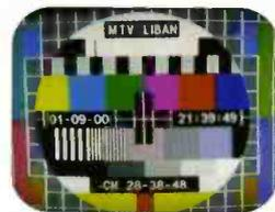
**Part of the Lebanese digital package on *Arabsat 3A*, a PM5534 test card.**
