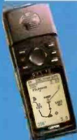
Ideal for walking or driving. With 12-channel reception it locks up very fast. And with the built-in antenna it is totally shower proof. Offers accurate positioning with selection of grids including British National Grid. Gives forward speed, compass direction, altitude, sunset/sunrise, ETA, waypoints and routes, zoom map display (user programmes points), and very accurate positioning to around 50ft. Requires 4 x AA cells (not supplied). Made by the top name in GPS, this is an absolute bargain!
