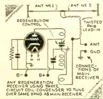
ceiver. It not only increases volume, but sharpens tuning as well. The regenerative receiver should be tuned to the frequency of the desired station and its regeneration control advanced to a point just below oscillation. Even with the power cut off from the regenerative receiver, the improvement in signal strength and sharpness is remarkably noticeable.
