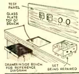
bench is usually littered with tools, solder, etc., and the large service manual would be in the way. Therefore, I have cut a slot in the front of my bench about 1/2" below the top. Instead of a drawer, I put in here two sheets (Continued on page 633)
