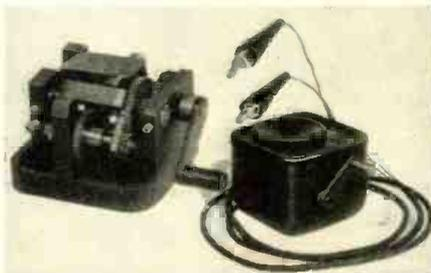
which vibrates an armature in the field of a permanent magnet, generating alternating current. Calling current is generated by revolving two discs of magnetic material, the teeth of which cut the field of the phone magnet. Photo courtesy Western Electric Co.
