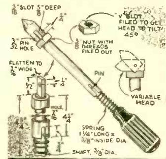
iron and the end of the shaft flattened and drilled to take a small metal pin. A spring is slipped over the shaft, then a piece of metal tubing over that, and finally a nut in which a V slot has been filed. The head is then pivoted to the end of the shaft. As the illustration shows, it may be turned to a number of convenient angles.—Thomas Horridge.
