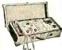
Here is the instrument every Radio expert needs and wants—an All-Wave. All-Purpose. Set Servicing Instrument. It contains everything necessary to measure A.C. and D.C. voltages and current; to test tubes, resistance; adjust and align any set, old or new. It satisfies your needs for professional servicing after you graduate—can help you make extra money fixing sets while training.
