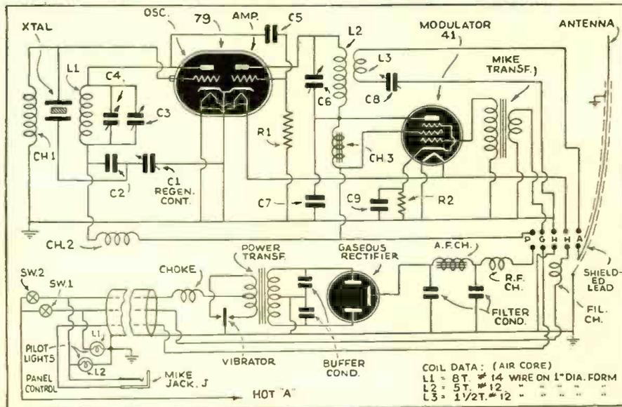
voltage only when desired. Voice currents are fed via the same cable to the modulator. Lights indicate the condition of the switch-operated circuits.
