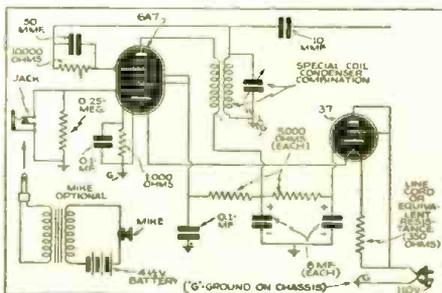
The pick-up is plugged into the jack provided for it and the radio tuned to the low-frequency end of the dial (around 600 kc.) where no station is heard and the turntable is then started. The condenser is varied by turning the adjusting screw until the record is heard through the loud-speaker with the volume control well up.
