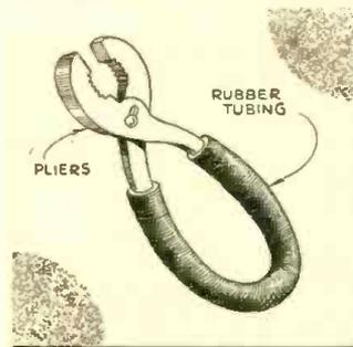
ing around live wires and also when a number of small parts must be picked up in rapid succession, or when the pliers must be opened and closed frequently, as when screwing a nut tight in a cramped space.—David Lloyd.
