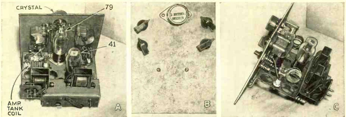
The Inside Story: Left, back view; Center, the panel, showing controls and crystal; Right, side view.
