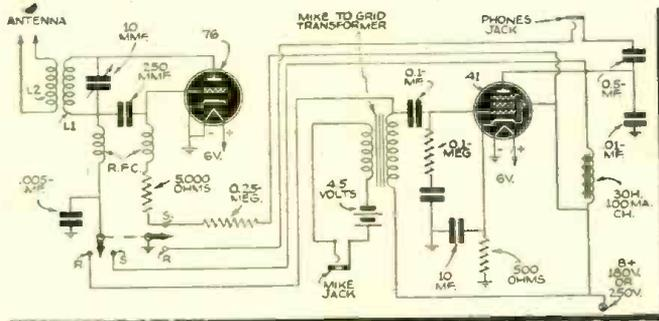
Circuit for 2½ meter Transceiver. No. 1168.
