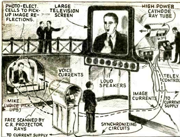
The new Telefunken television amplifier system—the scanning light illuminates the face of the subject and photo-electric cells pick up the reflected light rays, which are amplified and passed into the cathode tube behind the large image screen.
