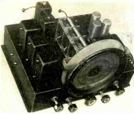
General view of the 6-tube superhet, with its calibrated dial. (No. 657).
