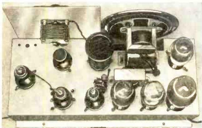
Top view of the 5-T receiver as built complete for broadcast, ordinary short-wave bands and 5-meter band reception—8 tubes in all.
