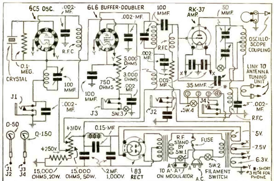
Diagram of crystal oscillator, buffer-doubler and amplifier, together with plate supply.
