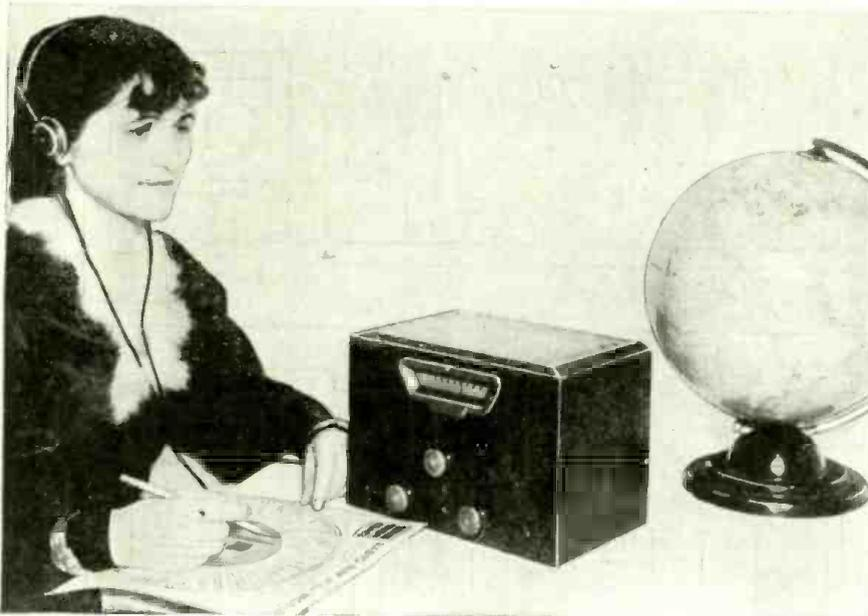
This 3-tube receiver is to be operated from a 110 volt A.C. circuit. A 58 tube is used as a detector as it is very reliable for this purpose. The detector output is fed into a 56 audio amplifier. The third tube is a rectifier. Plug-in coils are used to change the wave bands.
