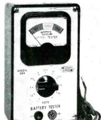
Battery tester (kit or factory-wired) for checking portable radio and hearing-aid batteries under operating conditions. Uses rotary selector switch which inserts proper dropping and shunt resistors in meter circuit to reduce terminal voltage. For 1.5 to 90 v. (Model 584; Electronic Instrument Co., Inc., 84 Withers St., Brooklyn 11, N. Y.)
