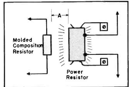
Fig. 6. Drawing illustrating need for keeping molded resistors far enough away from heat-producing components to hold ambient temperature of molded resistor below surrounding temperature, thus preventing overload.
