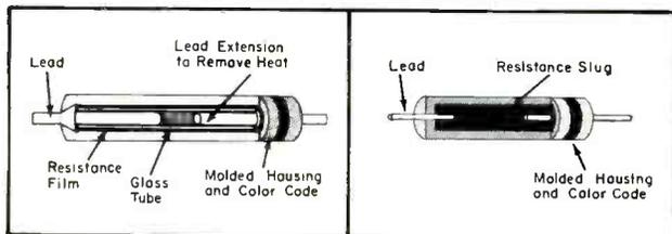
IN GENERAL, there are two types of molded-composition resistors in use today. One uses a film of resistance material applied to the outside of a glass tube for its resistance element and the other uses a solid body of resistance material. A cutaway section of these types, indicating their construction is shown in Fig. 4.
