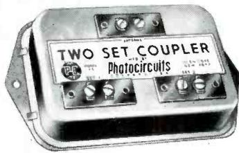
Two-set pc coupler, using wound sections of copper ribbon wire on a fiberglass support, connected to match 300-ohm signal input. (Photocircuits Corp., Glen Cove, N. Y.)
