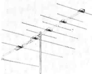
Wide band directive arrays for fringe and sub-fringe areas. Colinear phasing sections employed in both driven and parasitic elements. All aluminum construction; quick-rig assembly. (Thunder Bird series; Telrex.)
