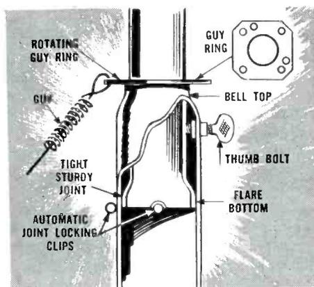
Comes complete with optional base—rotating guy rings for 3 or 4 guy points. MB-1 Standard Base for mounting on flat, vertical, sloping, or peak roofs.
