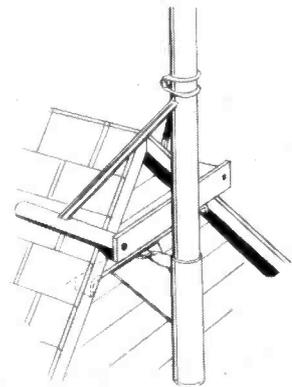
Gable mount designed for gable roofs. Accommodates tubing up to 1 1/2" in diameter. (Rohn Manufacturing Co., 116 Limestone, Bellevue, Peoria, Ill.)
