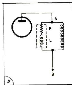
Fig. 5 (below). Gain control in video ii circuit: if R is replaced with a wire-wound resistor, circuit AB shown in (a) is changed and characteristics of circuit are radically altered as noted in (b) above. (See Fig. 8 for schematic of this portion of circuit in a typical TV chassis; Coronado 15TV4.)
