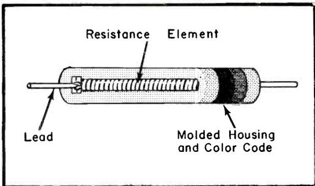
Fig. 1. Molded wire-wound resistor construction.
