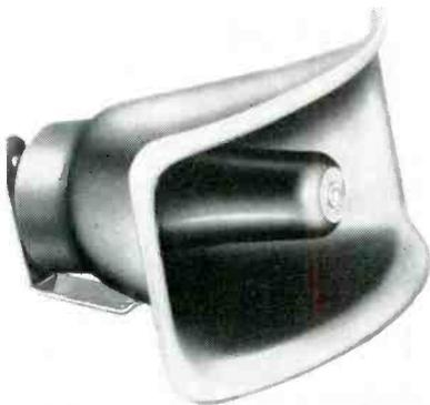
Five-watt cobra-jector speaker said to provide wide angle of dispersion in areas of high noise level, adverse wind conditions, etc. Main flare has fiberglass construction. Can be used for paging, talk-back, intercomm, industrial, marine and mobile applications. (Model CI-14. Atlas Sound Corp., 145 39 St., Brooklyn 18, N. Y.)
