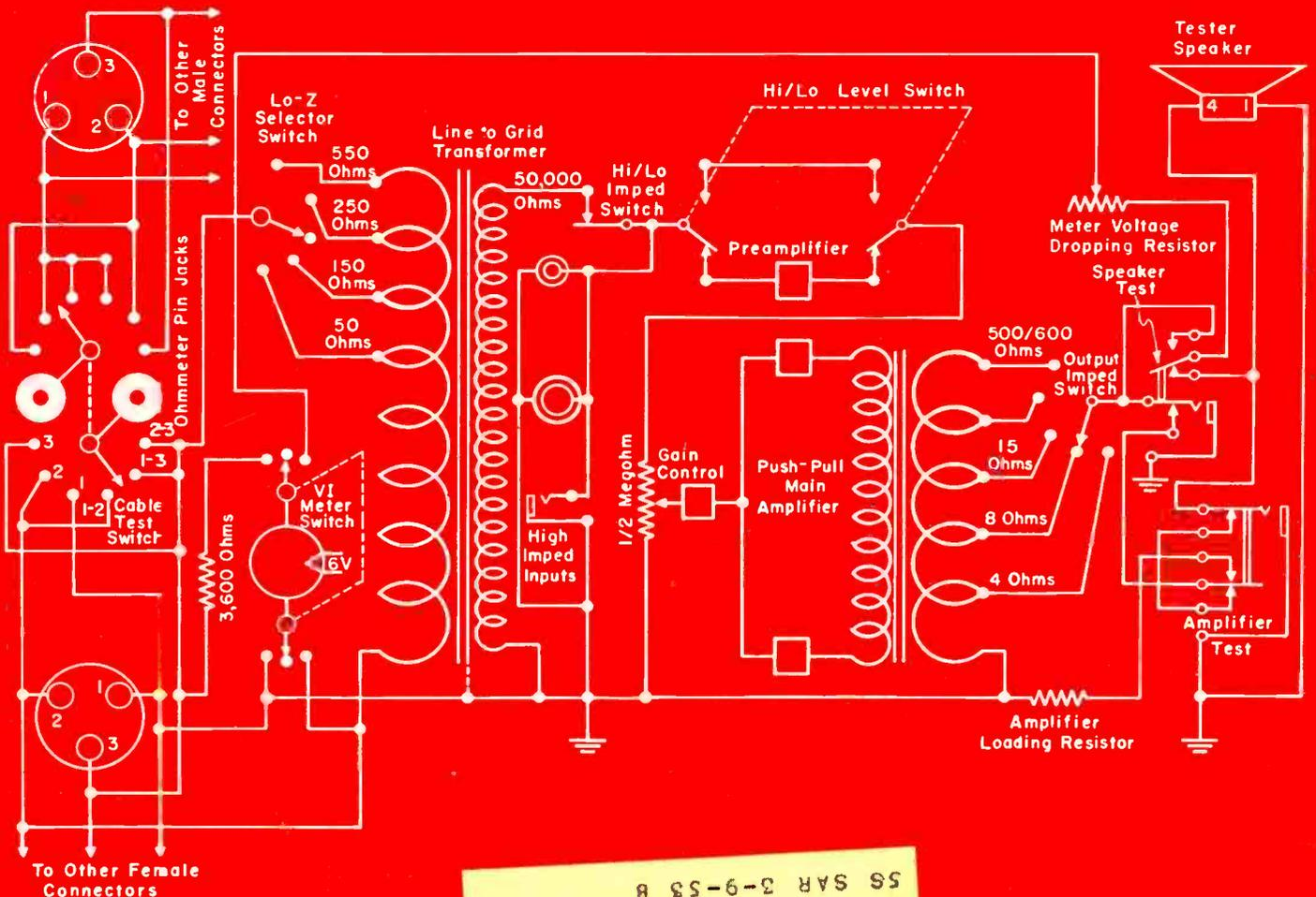
Audio test instrument designed to check operation of microphones, pickups, amplifiers and speakers. [See circuit analysis, this issue]
