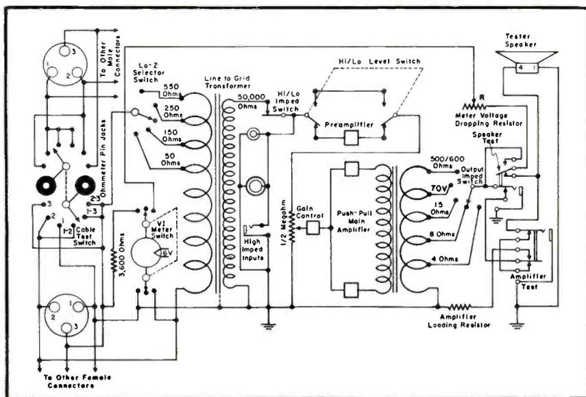
†In the model built, Cannon connectors were employed on the mike cables; Amphenol connectors on speaker cables.
