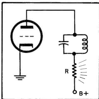
Fig. 2. Circuit illustrating point that one should never use resistors above voltage even though actual wattage is not exceeded. R (load) = .1 w and resistor rating = 1 w, but voltage across R = 350 v and voltage rating of R = 250 v; hence resistor R will break down to over-voltage.
