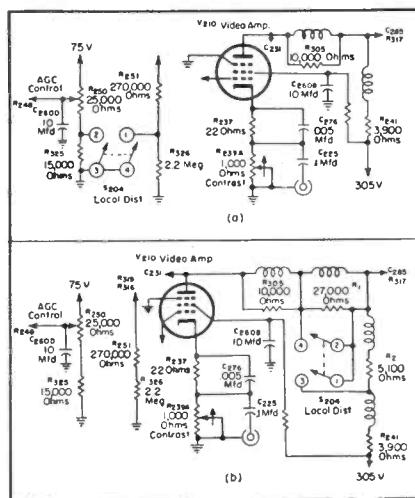
Fig. 2. Present (above) and modified video amp circuit (below) in DuMont RA-112A, RA-113 and RA-117, which provides more gain in fringe areas.
