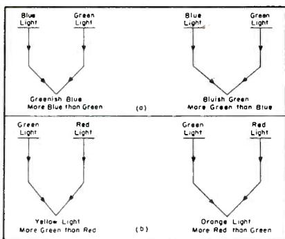
Fig. 3. How colors between primary colors can be created by mixing the right proportions of base colors.
