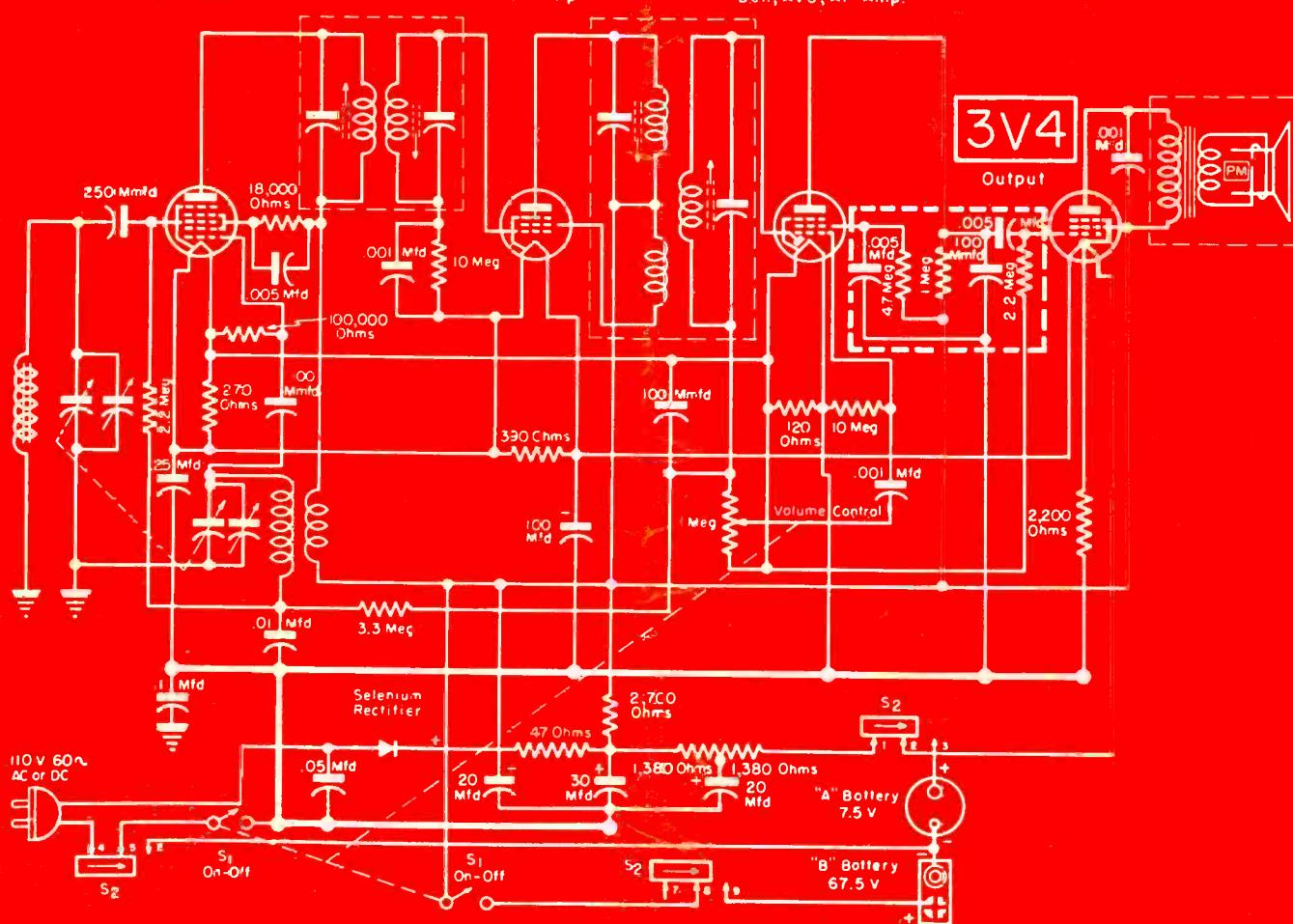
Four-tube ac-dc-battery portable featuring a printed-circuit audio-coupling assembly.
