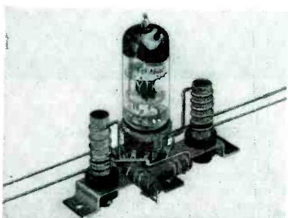
Vee-D-X single-channel outboard booster rf assembly.
