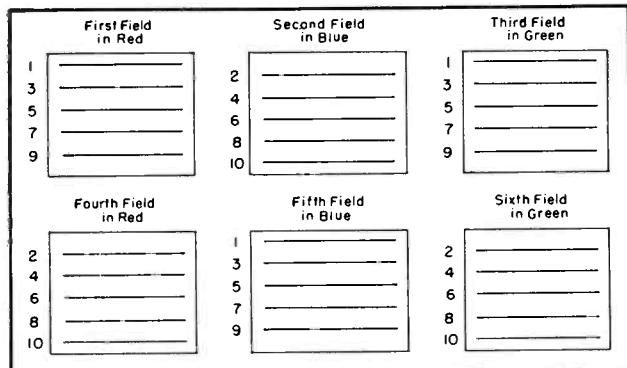
Fig. 5. Color sequence in the RCA system, letters representing sequence of color dots.
