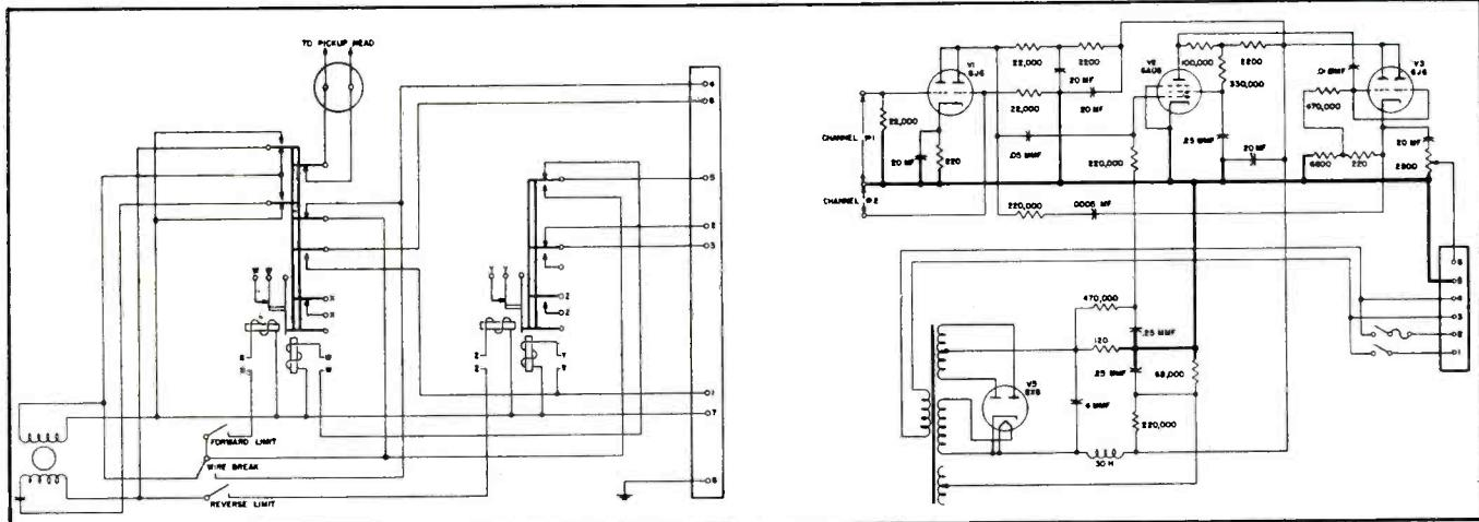
Fig. 2. Wire reproducer and preamp schematics.
