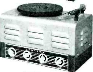
Model E-50: 50 watt performance leader in its price class. Multi-stage inverse feedback and push-pull parallel 6L6 tubes assure low distortion. Two mikes mixed, or one mike, one phone. Impedance selector simplifies speaker matching. With tubes and cover, retail . . .
