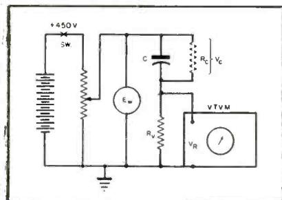
Fig. 2. Setup using a vacuum-tube voltmeter for the checking of leakage resistance of capacitors.  $C$  is a capacitor under test;  $R_c$ , leakage resistance of the capacitor in megohms;  $R_v$ , total resistance between the vtv terminals in megohms before the capacitor is placed into the circuit;  $V_c$ , voltage drop across  $R_c$ ;  $V_R$ , voltage drop across the vtv and  $E_w$ , working voltage for the capacitor being tested.
