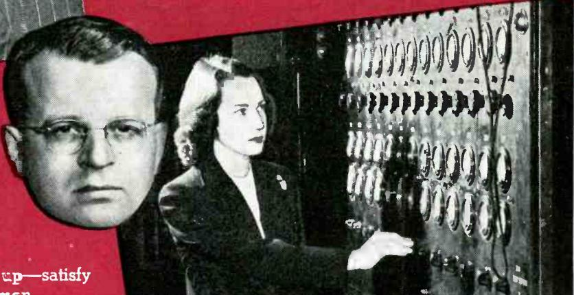
ROBERT HAGAN, Shop Foreman, Quality Laboratory, is in charge of the strict Life Test, above. It's typical of the numerous tests that Ken-Rad tubes must pass before leaving the plant.
