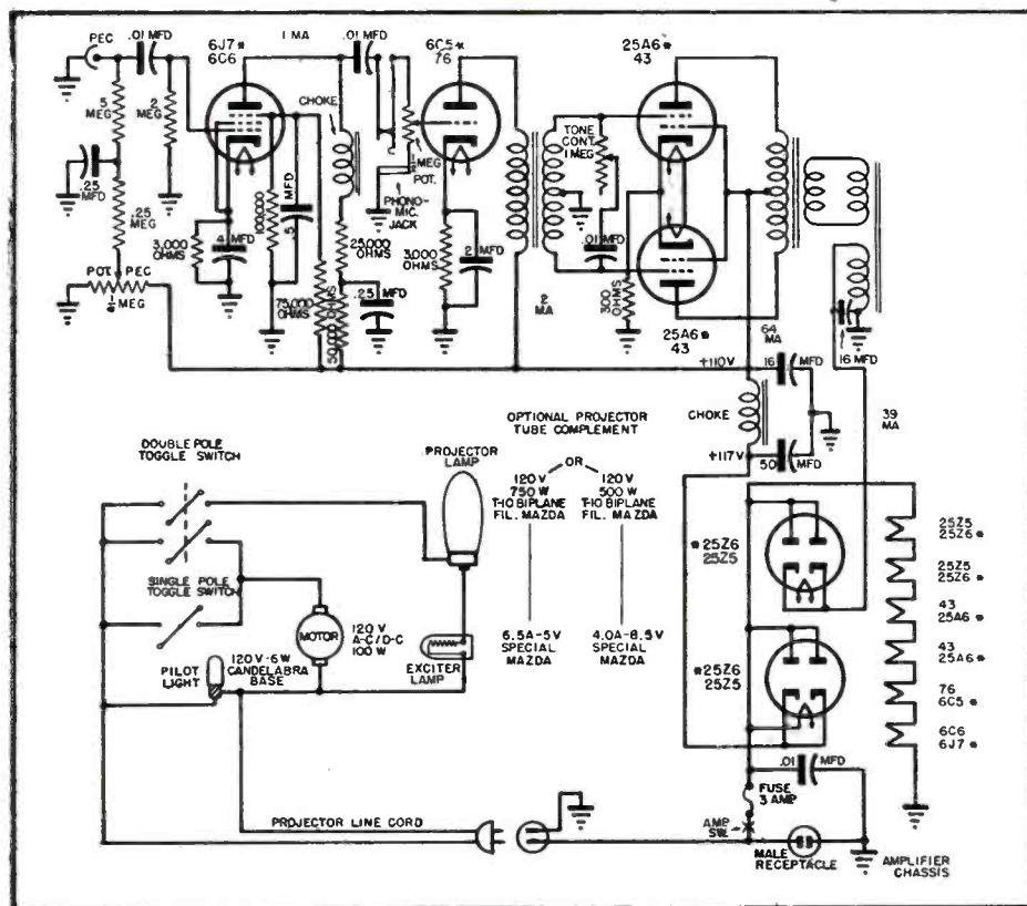
Fig. 1. Circuit of the projection and amplifier system of the Victor model 25 universal. Early models used the 6C6, 76, 43 and 2525; later models, 6J7, 6C5, 25A6 and 25Z6 tubes. Readings in ma were made at 115 v. a.c.
