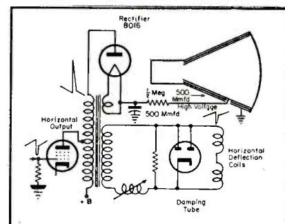
Fig. 5. A flyback high-voltage supply.
