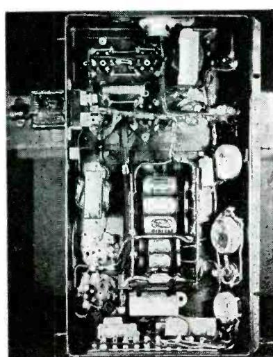
Fig. 4. Bottom view of amplifier showing the aluminum tubulars which replaced the electrolytics.
