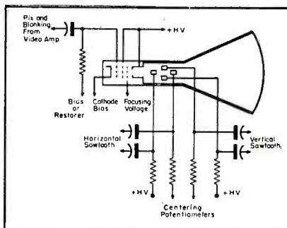
Fig. 4. A picture tube circuit for electrostatic deflection and focusing.
