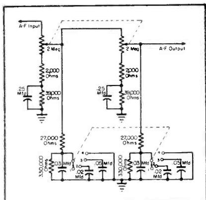
Fig. 3. A dual volume-control circuit used to obtain the desired bass-boost characteristics over a wide range of output levels. Circuit is similar to that used in the G.E. model 41.
