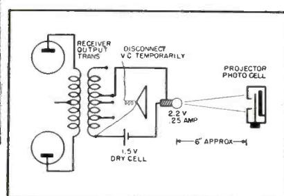
Fig. 3. Projector amplifier test circuit using a sound-to-light conversion with a receiver.
