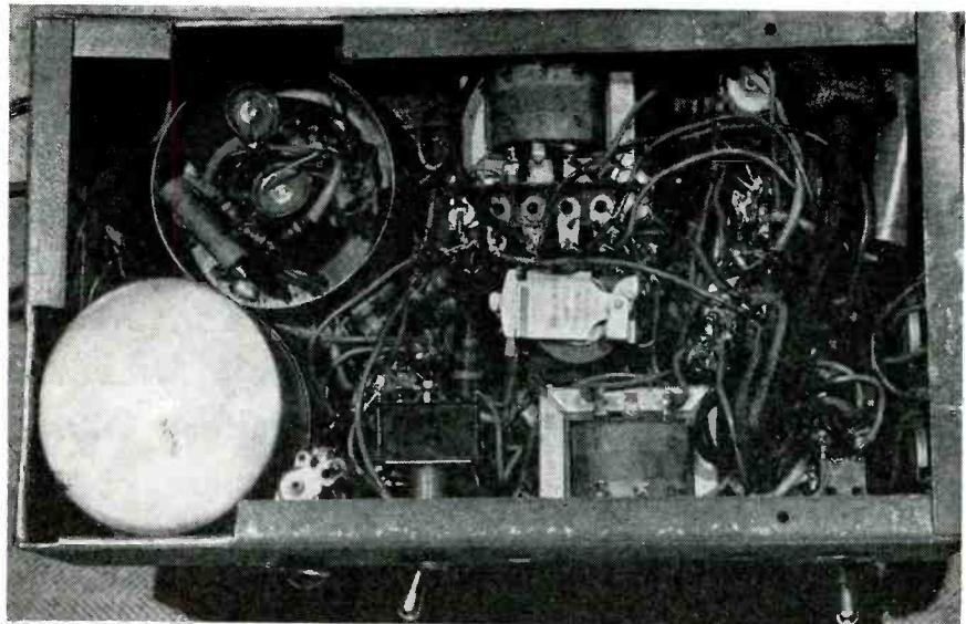
**Bottom view of chassis with cover of high gain stage of one channel removed. Switch at lower left is the listening switch. Relay in center is E relay.**
