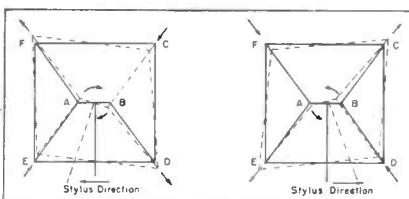
Fig. 1. Action of harness on crystal for rotational motion.
