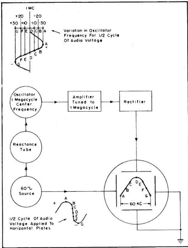
Fig. 3. Simplified visual alignment circuit.
