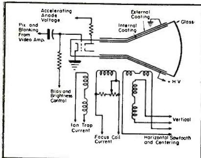
Fig. 3. Picture tube circuit for magnetic deflection and focusing.
