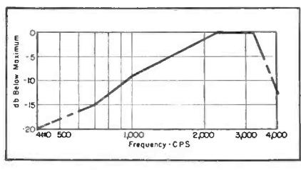
Fig. 1. Overall acoustic response, from microphone input to horn output, of typical electric megaphones.
