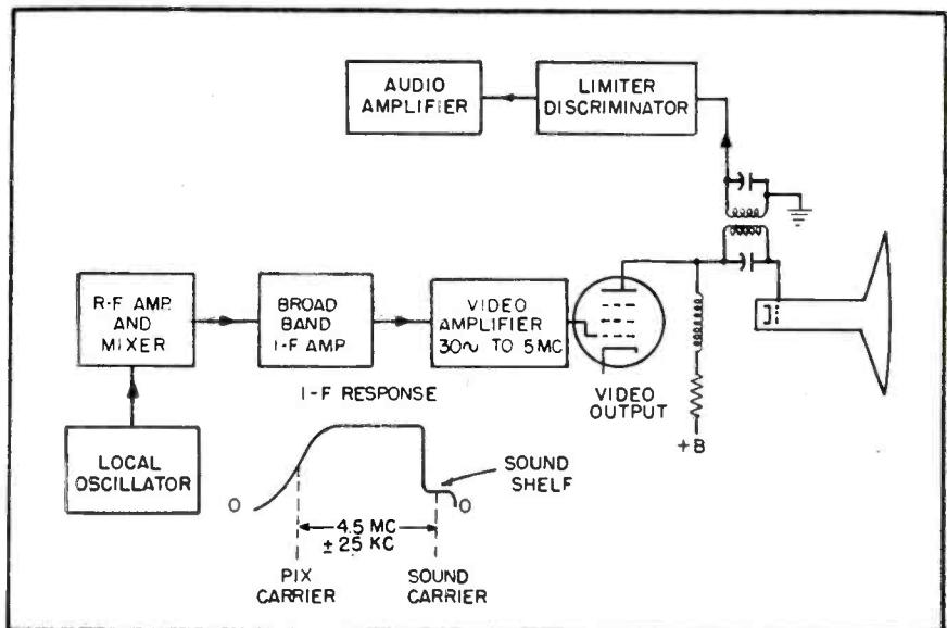
been developed by G.E. In this system, Fig. 2, the picture and the sound are carried through the picture i-f and video amplifiers up to the grid of the picture tube. Only one i-f system is necessary. The sound is taken off a tuned-circuit located between the video output and the grid of the picture tube which is tuned to 4.5 mc. The sound is then passed to a conventional limiter-discriminator and audio system.
