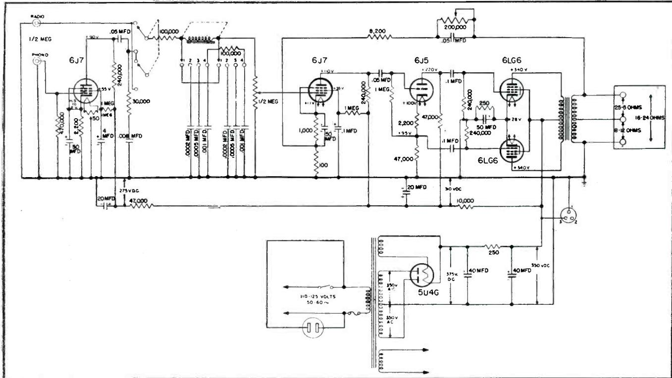
Fig. 4. Circuit of the Altec Lansing amplifier kit.
