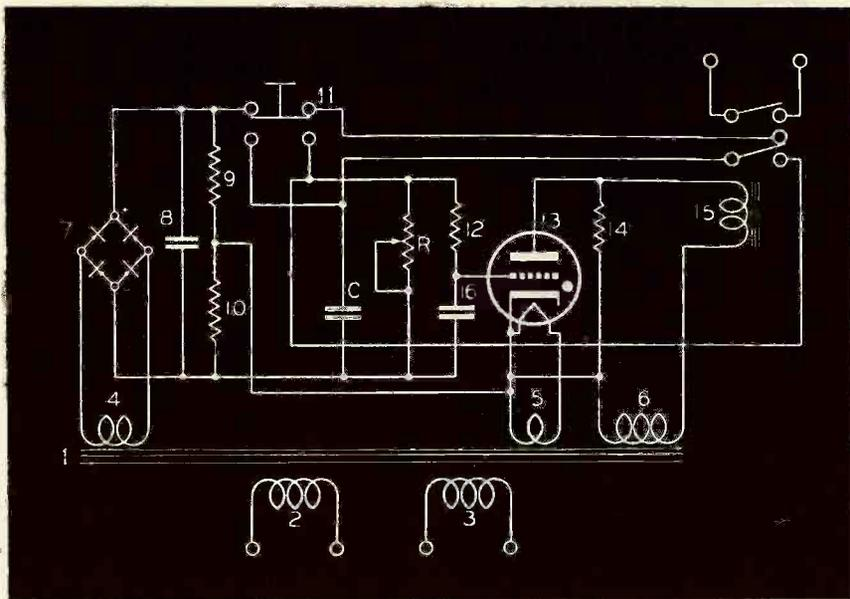
Fig. 4. Fundamental timing circuit using thyatron tube.
