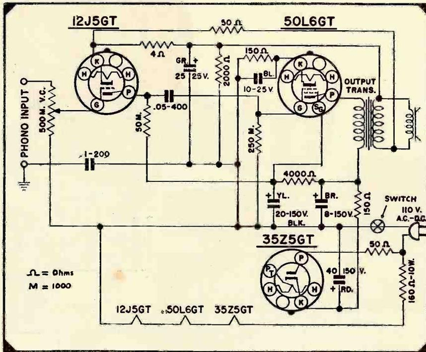
Fig. 3. A 3-tube amplifier with degeneration. A 50-ohm resistor determines the amount of feedback applied.
