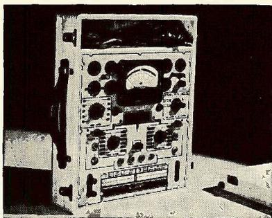
load for various voltage ratings of batteries. The d-c voltmeter ranges are from 0-25-10-50-250-1000-5000; a-c voltmeter ranges from 0-10-50-250-1000-5000; output voltmeter ranges are 0-10-50-250-1000-5000; d-c milliammeter ranges: 0-.5-2.5-10-50-250-1000; d-c ammeter range, 0-10 amperes.
