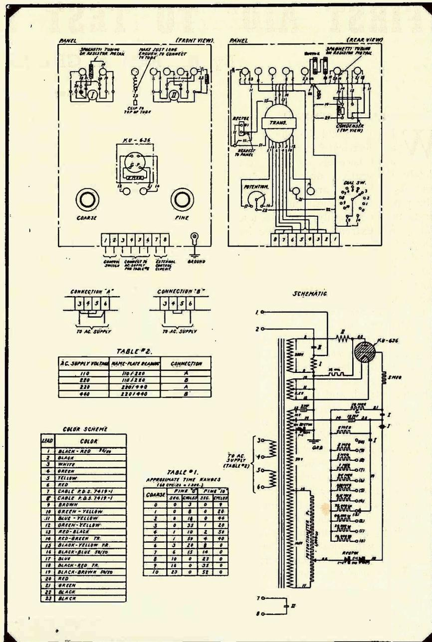
Fig. 6. Diagrams of a typical timing unit with circuit characteristics.
