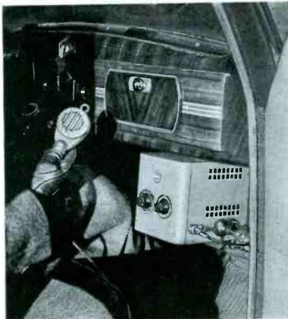
highly efficient marine type speaker may be mounted under the hood as shown, or on the outside of the car if preferred.
