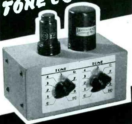
A simple circuit gives you an effective tone compensating system to boost or attenuate the bass and treble frequencies independently of each other. It may be incorporated in your present amplifier or receiver.
