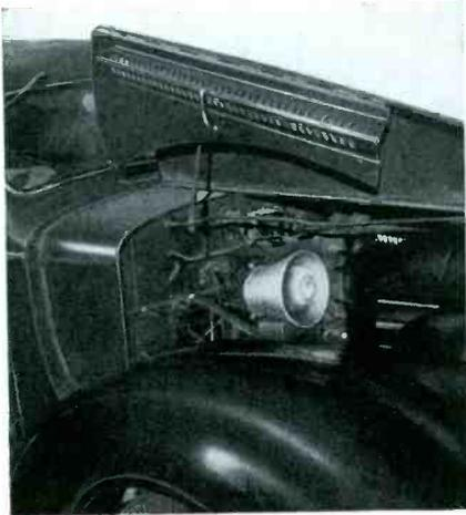
Fig. 2. Any automobile can be converted as a sound car with equipment that is no more cumbersome or conspicuous than the ordinary auto-radio receiver. The miniature marine type speaker is mounted under the hood, but can be mounted on the outside of the car if desired.
