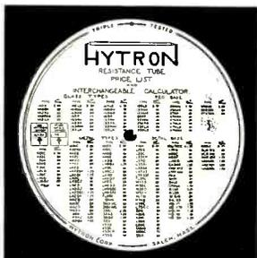
appears the special type number, in the other slot appears the Hytron type number to use having the same electrical and wiring characteristics.
