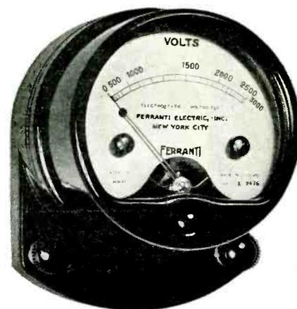
scale reading of 3,000 volts and a (full-scale) capacitance of only 8 mmfd can be connected across r-f circuits up to 1,500 kc. Ten different full-scale readings of from 150 to 3,500 volts are available. Three models can be obtained: portable, projecting or flush, in 2½ in., 3¼ in. or 4 in. dials.
