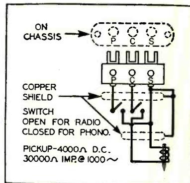
Fig. 4. Phonograph pickup connections.
