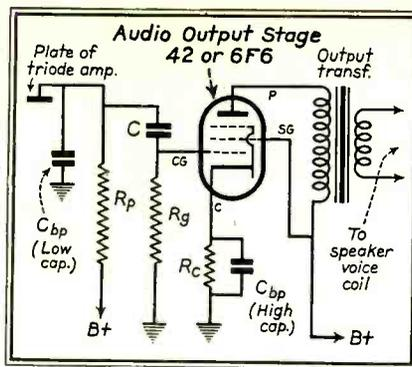
Fig. 5. Typical output stage.
