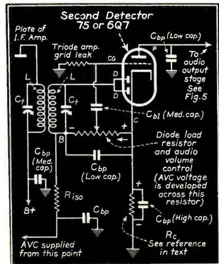
Fig. 4. A simple second detector stage.
