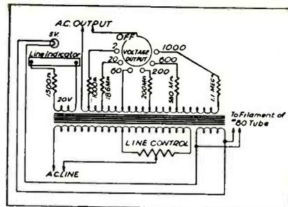
Fig. 3. Transformer circuit Triplet 1240.
