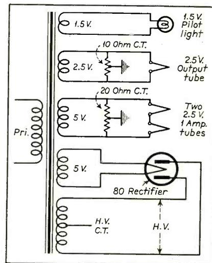
5-volt winding originally designed for the 71A's, will not overload that winding. If this 5-volt winding is center-tapped, one tube can be connected across each half of the winding. The other 5-volt winding together with the high-voltage winding is used to operate a type 80 tube to supply plate power for the amplifier.
