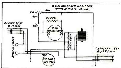
Fig. 2. Capacity test circuit.
