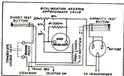
Fig. 1. Breakdown test circuit.
