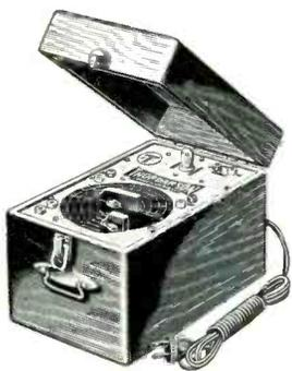
case, an etched and drilled metal panel with a scale calibrated in microfarads, matched panel mounting screws, and complete instructions and assembly plans for a condenser capacity-leakage tester.
