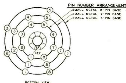
Fig. 2. Base and socket pin-numbering arrangements for the new metal tubes. See Table III on this page.
