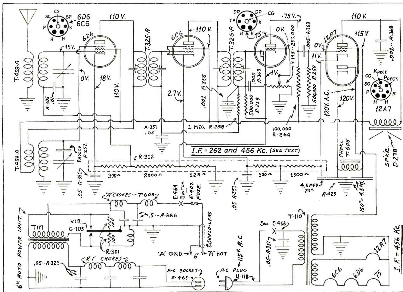
Circuit of International Model 90, together with circuit of attachment for 6- or 32-volt operation.
