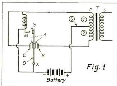
Circuit of typical full-wave shunt vibrator.
