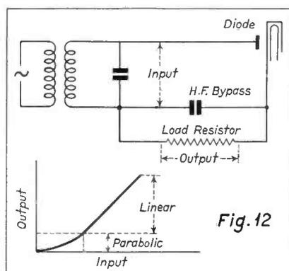
Input-output characteristic of diode, illustrating parabolic and linear portions of curve.
