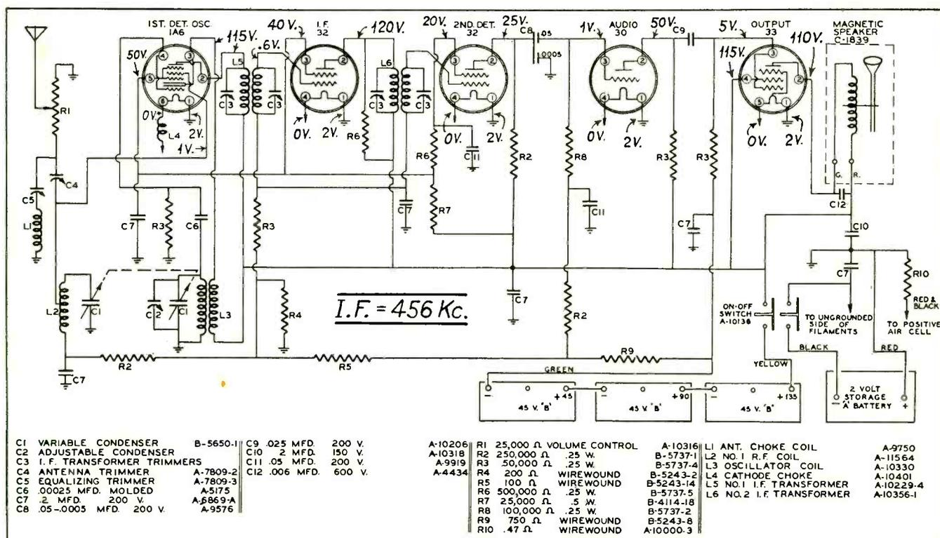
Circuit of Sparton Model 58, with socket voltages and parts values.
