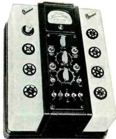
incorporates a fundamental advance in testing tubes on the basis of total emission, in that three separate loads, one for general purpose tubes, one for battery types and one for diodes, are available as required at the throw of a switch. Thus, total emission tests for each type of tube may be obtained on a specific load basis, and without possibility of damage to the tube structure itself.
