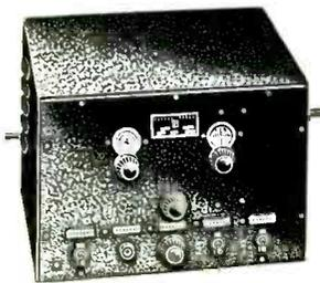
except that it has a second modulated oscillator that wobbles the output of the first oscillator plus and minus 15 kc when it is desired to use with a cathode-ray oscilloscope. With the wobble circuit switched off, the Model OM may be used as a standard 400-cycle modulated oscillator for output meter indications.
