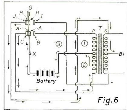
Second action of the full-wave synchronous vibrator.
