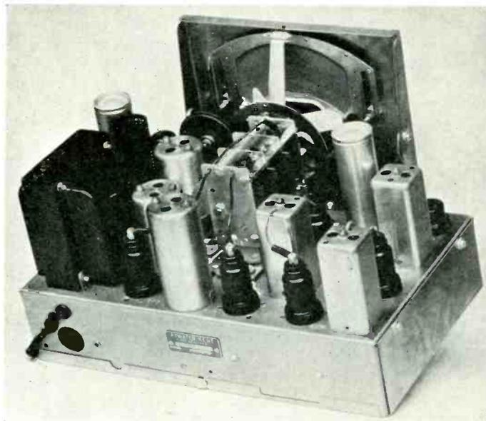
One of the new 1935-6 Atwater Kent metal-tube chassis—9 tubes in all, including a 6H6 twin diode.
