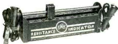
scales, 0 to 10,000 ohms and 10,000 to 100,000 ohms, permit accurate readings from 100 to 100,000 ohms. This range may be extended indefinitely by the addition of fixed IRC Metallized Resistors in series. A ball-bearing, spring-cushioned slider running along a rod at the top makes it possible to tap off any desired resistance value or voltage.
