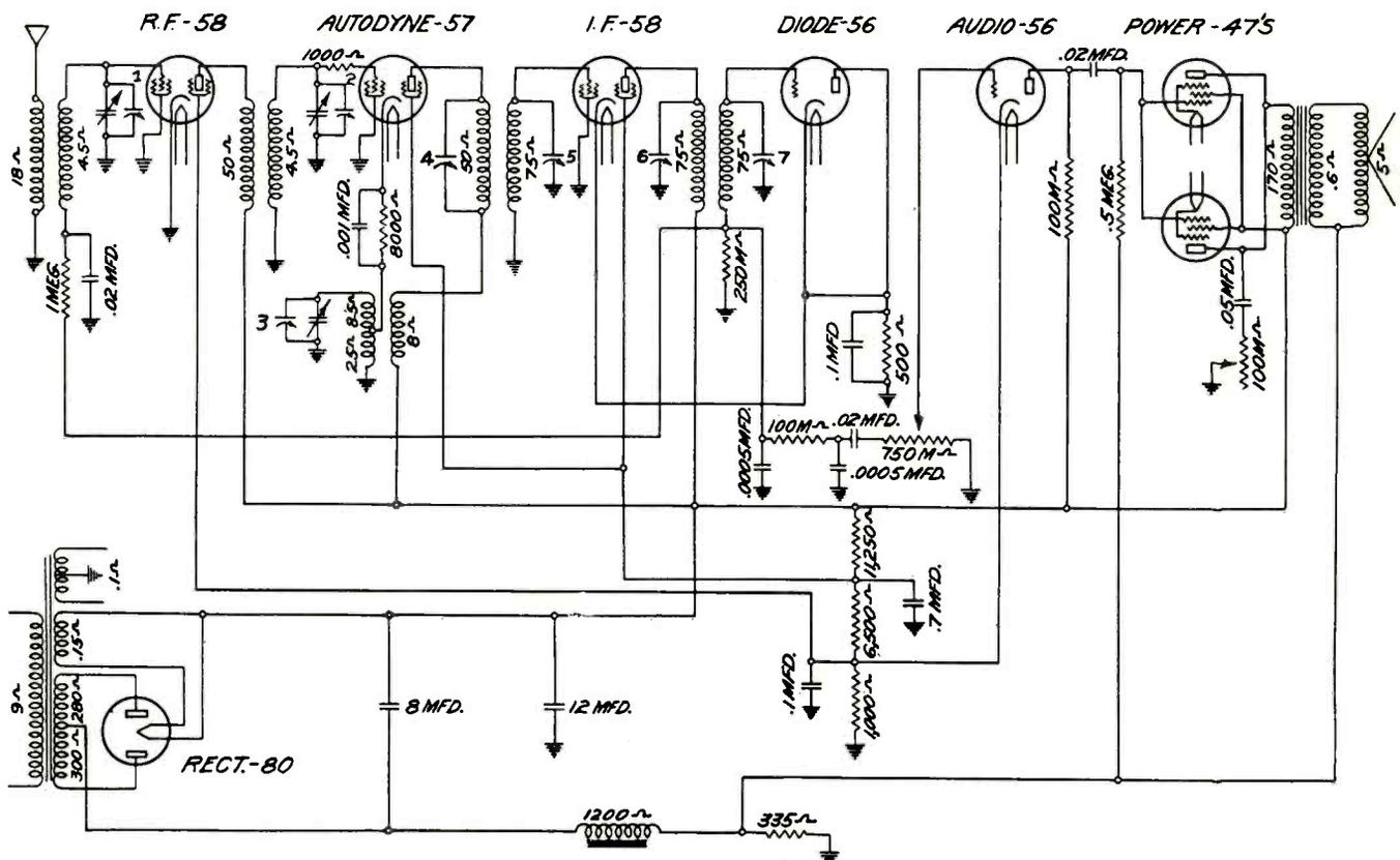
Circuit diagram of the Clarion Model 340 Super, with two 47 tubes in parallel. Test data is on the opposite page
