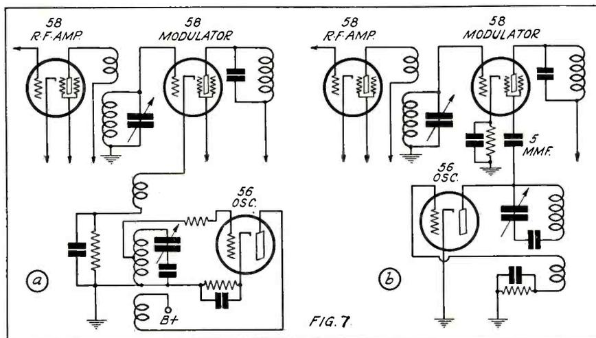
Illustrating inductive and capacity coupling between oscillator and modulator tubes. These are the forms of coupling most commonly employed
