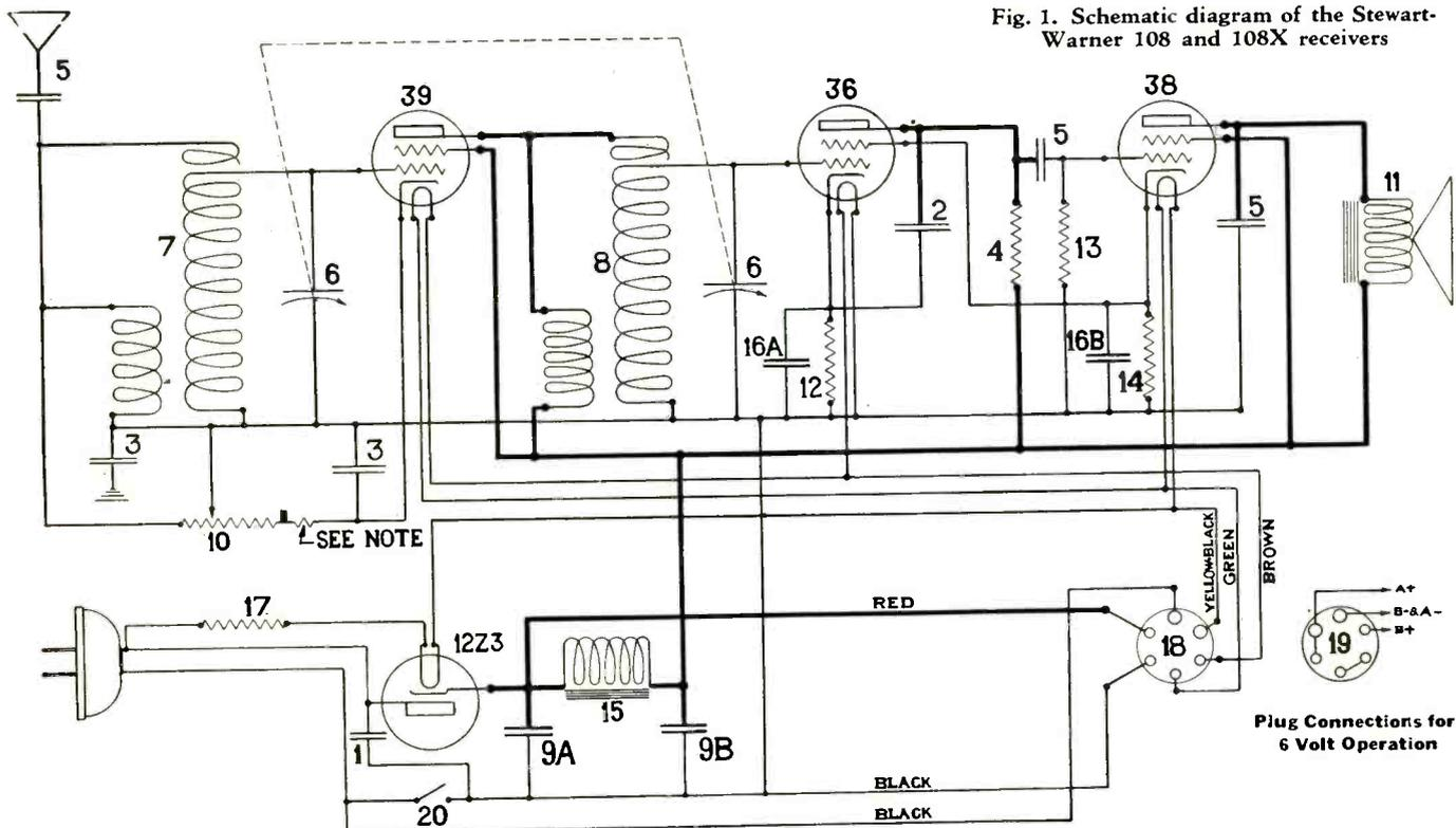
NOTE: In some receivers, a 140 ohm, 1/4 watt carbon resistor, part 81646 is connected in series with the volume control; in other sets this resistor is built into the volume control.
