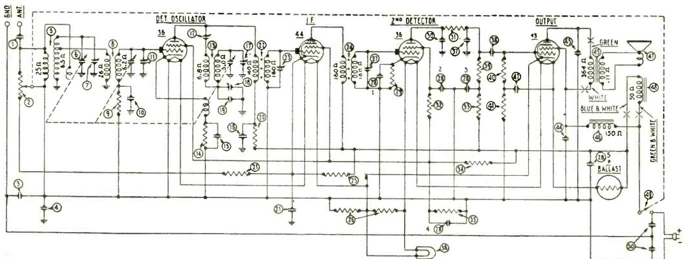
Circuit diagram of the Philco Model 48 D-C. receiver using series heater connection which includes the field of the dynamic speaker
