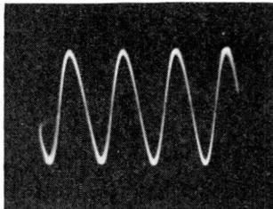
Fig. 1. The a-f. output of a set that is correctly tuned to a carrier
