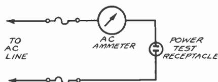
This simple layout will enable you to check the power consumption of a-c. receivers.
