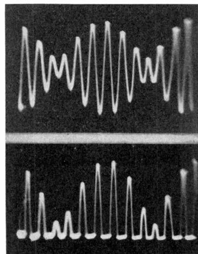
Fig. 4, above. A modulated voltage wave as applied to the rectifier of Fig. 1. Fig. 5. The modulated current wave in the load resistor, after passing through the half-wave rectifier.
