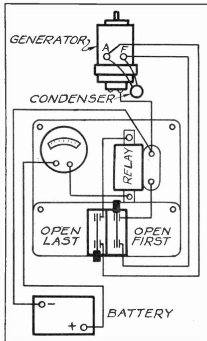
How switches are connected in the Wincharger circuit to prevent burnout.
