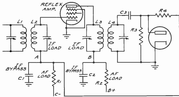
Fig. 3, left. The same tube here amplifies both i-f. and a-f. Figs. 4, 5, 6, below, are oscillograms of modulated signal, detector output, and a combination of the two.
