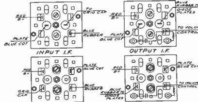
The two upper sketches show connections for the General Mfg. Co. transformers and the lower pair are those of the Meissner Mfg. Co., both types being used in Series A, B, and C.
