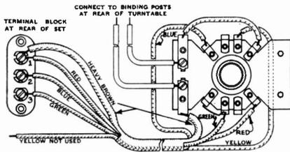
Fig. 1. Switch connections for phonograph.
