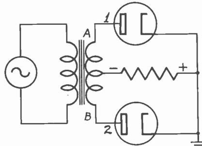
Fig. 6. Basic circuit of a full-wave rectifier.
