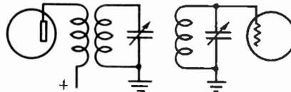
Fig. 3. An example of a pre-selector stage, using a three-winding transformer, two of the windings being tuned.
