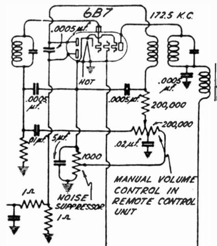
Fig. 6. An example of reflexing in the second detector of a superheterodyne, where the 6B7 is also an i-f. amplifier and controls the a.v.c.
