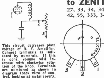
Due to the considerable current which this type of control must carry, a dual unit providing double wattage capacity is recommended.
