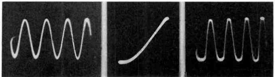
The sine wave of Fig. 11 was put through amplifier, whose operating characteristic is shown in Fig. 12. The wave of the output voltage is shown in Fig. 13. Compare with Fig. 11 and notice the distortion
