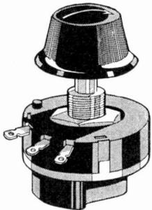
Centralab smoothness results from the action of the non-rubbing contact where-by a strip of polished metal rocks on the resistor ... and the only rubbing action is between an oilless wood bearing and the polished metal.
