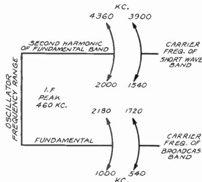
Fig. 4. The second harmonic of the oscillator frequency is used for heterodyning on the s-w. band in certain RCA receivers.
