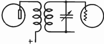
Fig. 1. A conventional r-f. transformer with tuned secondary that is used in TRF receivers.
