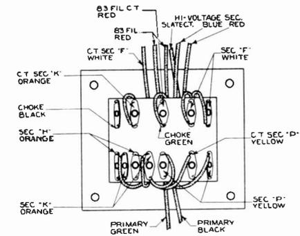
Connections to the new power transformer used in the Silvertone 1640
