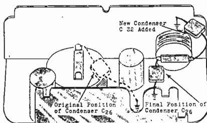
Schematic, Fig. 1, shows changes in Wells-Gardner 6R to eliminate motor noise. Fig. 2, below, shows new parts positions
