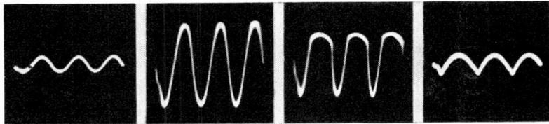
Figs. 2A, 2B, 2C and 2D, left to right. These oscillograms correspond with the four points designated along the horizontal axis of Fig. 1, and represent the demodulator output for a receiver not equipped with avc. The distorted output shown in Figs. 2C and 2D is due to overload and represents input in excess of S<sub>2</sub> in Fig. 1.
