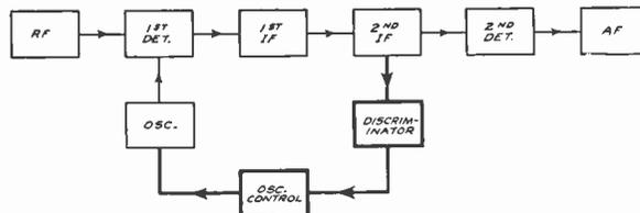
Fig. 3. The block diagram on the right shows how the discriminator and oscillator control tubes are incorporated in a superheterodyne receiver to obtain a.f.c. action
