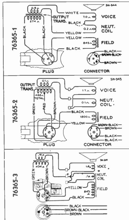
Color coding and connections of plugs and connectors for three RCA speakers.
