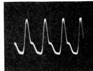
Fig. 2. When a set is incorrectly tuned, the a-f. output assumes this appearance
