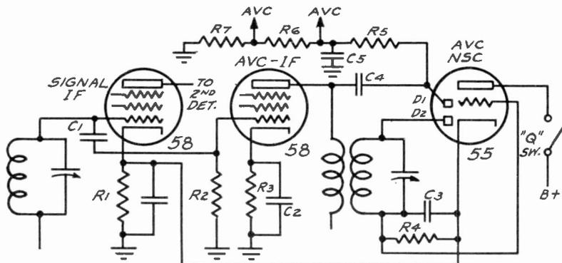
Fig. 4. A noise suppression circuit which operates to block the i-f. amplifier. This is accomplished by the automatic control of the drop across R1 as explained in the text.
