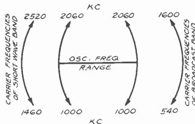
Fig. 3. The same range of oscillator frequencies is used for both the broadcast and s-w. bands in some Stewart Warner sets.
