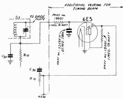
How the 6E5 tube is connected in the Pilot models mentioned in the text
