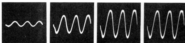
Figs. 3A, 3B, 3C and 3D, left to right. These oscillograms show the output corresponding to the avc curve in Fig. 1. Note the absence of distortion and that after a certain input is applied there is practically no change in the output level.
