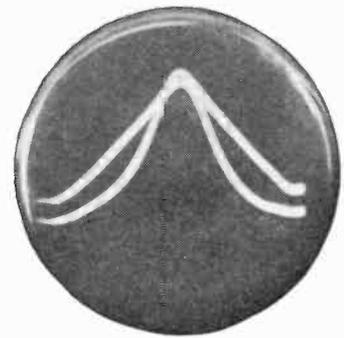
This i-f amplifier was aligned with output meter. Oscillograph shows distortion
