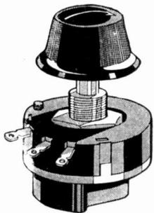
Centralab smoothness results from the action of the non-rubbing contact where-by a strip of polished metal rocks on the resistor . . . and the only rubbing action is between an oilless wood bearing and the polished metal.
