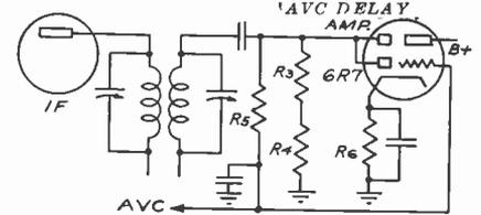
Fig. 10. The diode section of the 6R7 is used as the avc rectifier and the control voltage is fed to the delay amplifier through R5.
