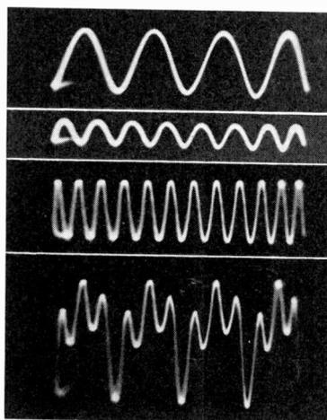
Fig. 10. A 1000-cycle sine wave and its second and third harmonics were combined, giving the wave shown at the bottom. Note the lack of mirror symmetry in the resultant wave.
