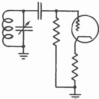
Fig. 7. The additional resistor connected between ground and the grid supplies the correct bias to this element of the tube.
