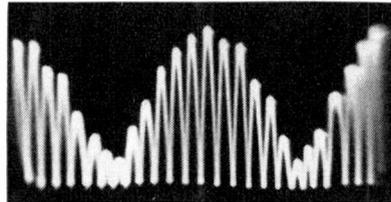
Fig. 7. A rectified modulated current wave flowing in resistor of Fig. 6.
