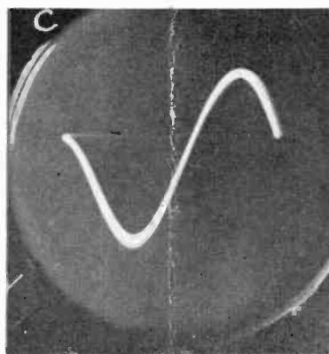
By partially darkening the room, undesirable reflections from the tube surface (see corners above) can be avoided and a greater contrast obtained
