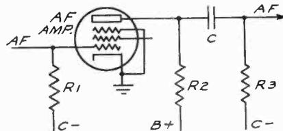
Fig. 2. A tube of the same type as that in Fig. 1, is here used as an a-f. amplifier.
