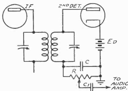
Fig. 1. A simple a.v.c. circuit wherein the second detector is blocked when the input falls below a certain level.
