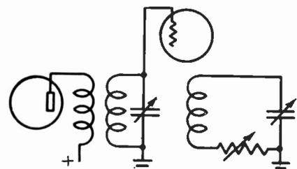
Fig. 5. One type of selectivity control is to have a variable resistor in series with the third winding of the i-f. transformer.
