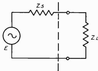
Fig. 1.  $E$  is the a-c. voltage source and  $Z_s$  represents its impedance.  $Z_L$  represents the impedance of the load.
