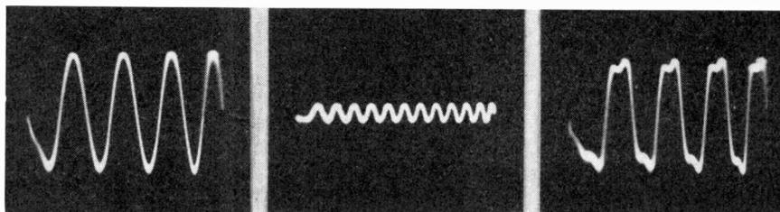
The 1000-cycle sine wave, Fig. 7, left, and the 3000-cycle wave Fig. 8, were combined, giving the wave of Fig. 9. Note the "mirror symmetry" of the latter, due to the presence of the third harmonic and compare with Fig. 6
