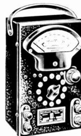
A low cost set analyzer and all-purpose component tester with a big, easy-to-read 5-inch fan-type meter. Ranges: 0-15-150-750 v d.c. and a.c., 0-1.5-15-150 ma d.c., and ohms scales 0-100, 0-20,000, and 0-2 meg. Low ohms range is new shunt type with maximum battery drain only 2.5 ma. Hand calibrated in the C-B Standardization Laboratory. Write for new bulletin.
