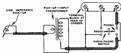
Fig. 2. Setup used when turntable is used at some distance from the receiver.
