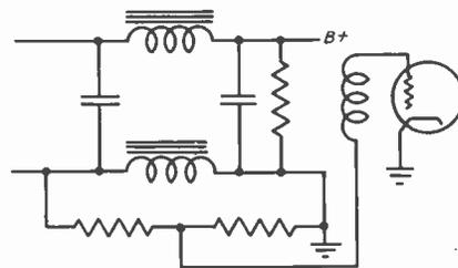
Fig. 8. An example of the grid bias for an a-f. tube being taken off a resistor shunted across a choke in the negative leg of a power unit filter, thus making the grid negative with respect to ground.
