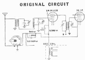
Due to the obsolete system of control used in the Stewart-Warner 102-A, B and E Receivers, it has hitherto been impossible to obtain satisfactory volume control operation. By utilizing the specially-designed 2107 control and making several circuit modifications as shown below, all difficulties can be eliminated and entirely satisfactory operation assured.
