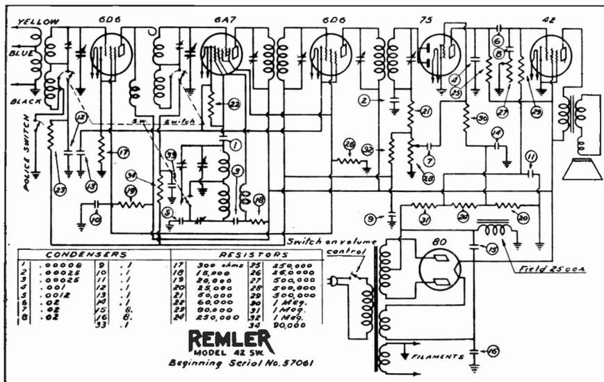
Remler Model 42 short wave receiver has been revised starting with serial number 57061. Compare this schematic diagram with that for the early chassis.
