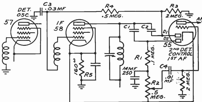
Fig. 9. The type 55 tube performs the triple function of second detector, first a-f. amplifier, and delayed avc control. The d-c. voltage for control purposes is developed across the resistor  $R_3$ .
