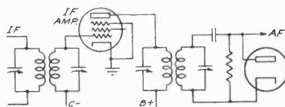
Fig. 1. A conventional i-f. stage coupled to a diode detector.
