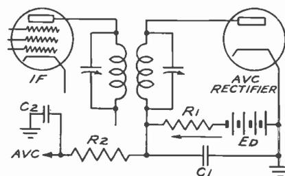
Fig. 5. The essential elements of a circuit commonly used in receivers having delayed avc is here shown. Note the battery for introducing the negative bias on the diode plate.
