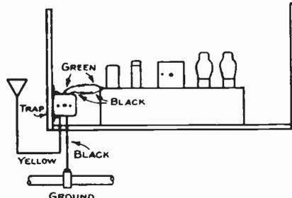
Installation of wave-trap in various Silvertone chassis
