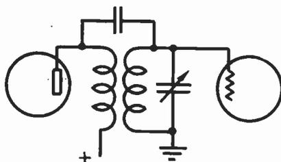
Fig. 2. An r-f. transformer which has both inductive and capacitive coupling.
