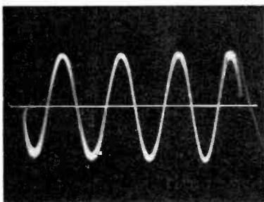
Fig. 1. An example of a pure sine wave. The horizontal reference line was added after the oscillogram was made
