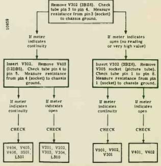
Figure 46. Simplified Test Procedure for Locating an Open Circuit Heater Tube in Sets With Son-R Remote Tuning.
