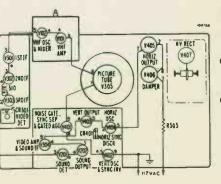
TUBE LOCATIONS AND HEATER CIRCUIT †25CD6GB in chassis Run 10 thru 22; 12DQ6A
