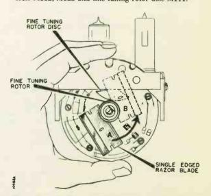
Figure 58. Front View of VHF Tuner Showing Method of Inserting Fine Tuning Disc and Fine Tuning Rotor.
