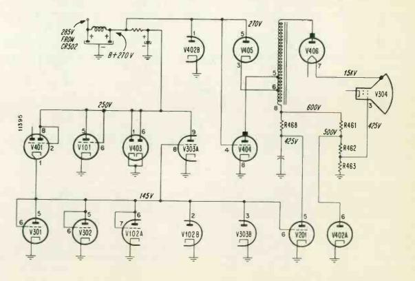
Figure 54. Simplified B+ Distribution Diagram. TV Chassis 15D1B.
