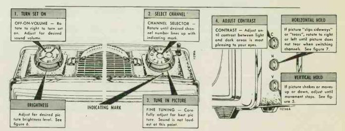
Figure 27. Top Oblique View of Models using TV Chassis 15D1B. Location of controls shown.
