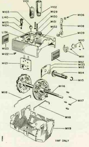
Figure 57. Exploded View of VHF Tuners 94E144-13, -19, -24, and -26.
