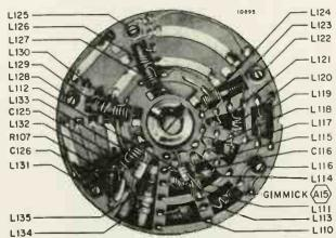
Figure 29. View of Oscillator-Mixer Rotor Disc in VHF Tuners 94E144-9, -22, -27 and -30.
