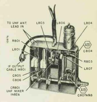
Figure 60. View of UHF Tuners 94D112-5 and 94D155-3, Cover Plate Removed.
