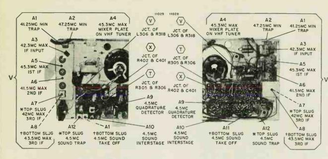
Figure 24. Component View of Printed Wiring Board Showing Test Point Locations and IF Alignment Data.
