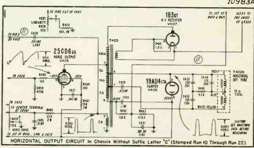
Figure 67. Horizontal Output Circuit in Chassis Without Suffix Letter "C" (Stamped Run 10 through Run 22). See Schematic Diagrams for Horizontal Output Circuit in Chassis with Suffix Letter "C" (Stamped Run 23 or Higher).
