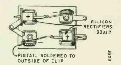
Figure 66. View of Fuse Holder Showing Position of Pigtail Type Selenium Rectifiers.
