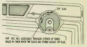
Figure 11. Front View of VHF Tuner In Table Models.
