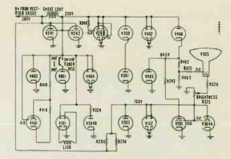
Figure 43. Simplified B+ Distribution Diagram for VHF-UHF
