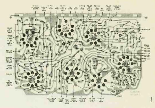
Figure 49. View of Wiring Side of Printed Wiring Board A5780-1 Used in All Chassis Except 16U1C, 16AU1C, 16W1C, and 16AW1C. Gray area represents printed wiring; black symbols and lines represent components and connections on opposite side.
