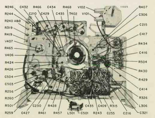
Figure 54. Wiring Side of Chassis With Push-Pull Sound Amplifier.
