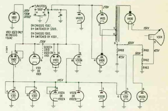
Figure 53. Simplified B+ Distribution Diagram. TV Chassis 15A2, 15A2C, 15B2, 15B3 and 15UA2.
