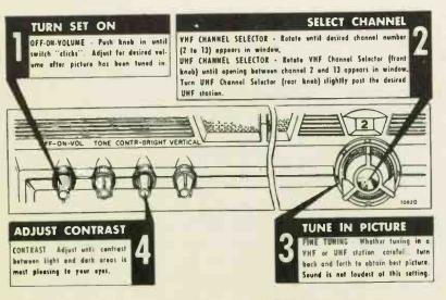
Figure 2. Operating Instructions for VHF-UHF Sets with Tone Control. Figures at Right Show Control Locations in Other Models.
