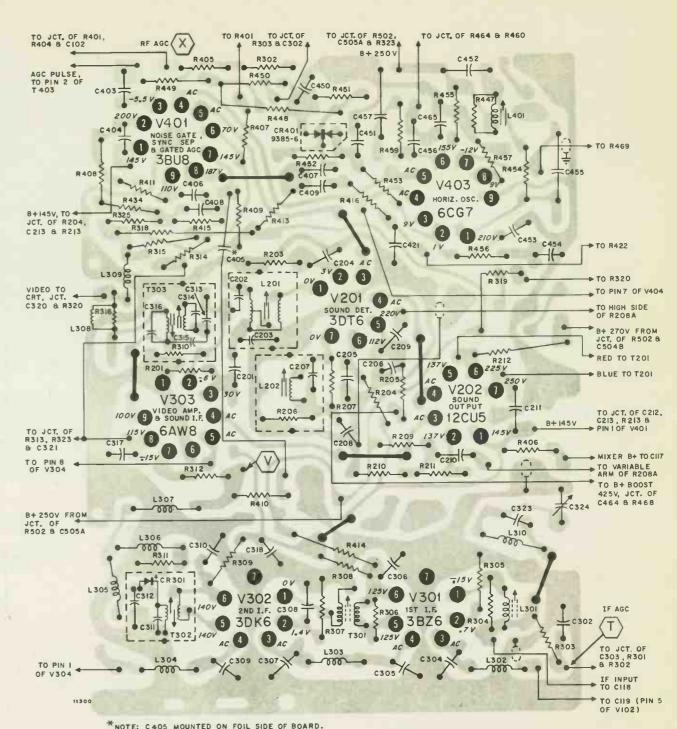
Figure 56. View of Etched Wiring Side of ETCHED CIRCUIT BOARD A7585-1. Gray area represents etched wiring; black symbols and lines represent components and connections on opposite side. A7585-1 is used with TV chassis 15D1B.
