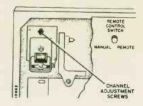
Figure 15. Rear View of San-R Models Showing Channel Selection Screw Location.
