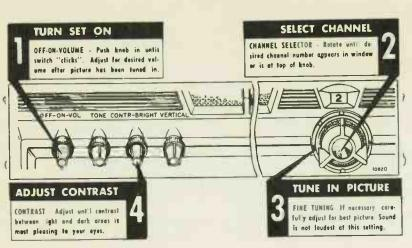
Figure 1. Operating Instructions for VHF Sets With Tone Control. Figures at Right Show Control Locations in Other Models.
