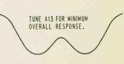
Figure 39. 41MC IF Trap Adjustment.
