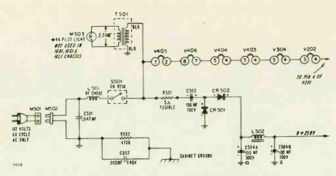
Figure 64. Heater Circuit in 16 and 17 Tube Sets Stamped Run 10 through Run 22. See Complete Schematics for Heater Circuit in Sets Stamped Run 23 or Higher (with suffix letter "C" added to chassis number).
