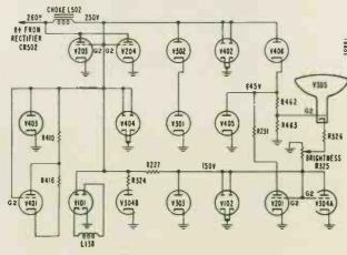
Figure 42. Simplified B+ Distribution Diagram for VHF Receivers With Push-Pull Sound Amplifier.
