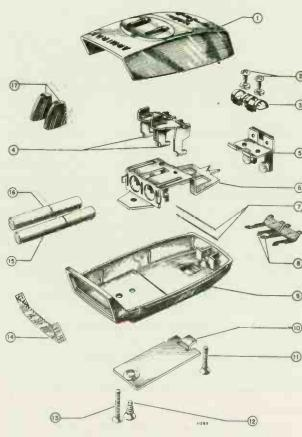
Figure 58. Exploded View of Son-r Tuner S21A. See Parts List for part numbers and descriptions.
