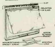
Figure 18. Illustration of Picture Window Mounting.
