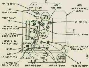
Figure 33. Top View of VHF Tuners 94E144-9, -22, -27, -30 and UHF Tuner 94D112-5 or 94D155-3 Showing Adjustment Locations.
