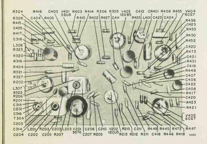
Figure 75. View of Component Side of Printed Wiring Board A5780-5 used in 16R1C, 16AR1C, 16S1C and 16AS1C Chassis. See Service Manual No. ST597-2 for other Printed Wiring Views.
