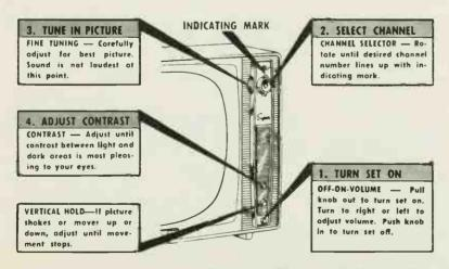
Figure 23. Tuning Instructions for Models using TV Chassis 15A2 and 15A2C.
