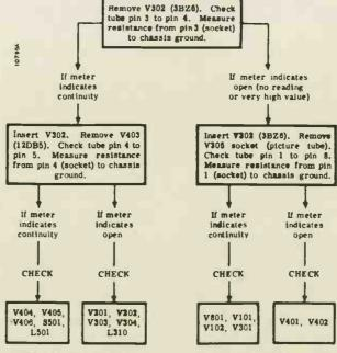
Figure 44. Simplified Test Procedure for Locating an Open Circuit Heater Tube in Sets With Single Ended Sound Amplifier. Note V801 in VHF-UHF Sets Only.
