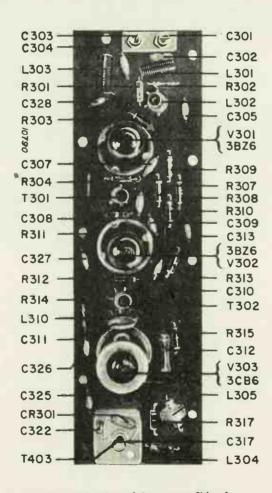
Figure 48. View of Component Side of Printed Wiring IF Board A5775-1.
