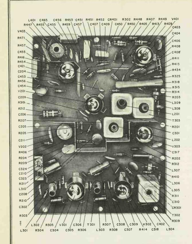
Figure 55. View of Component Side of Etched Circuit Board A7585-1. A7585-1 is used with TV chassis 15D1B.
