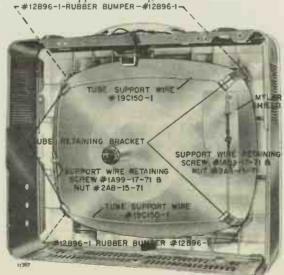
Figure 34. Rear View of Models using Chassis 15D1B with Chassis Removed. Method of picture tube mounting shown.
