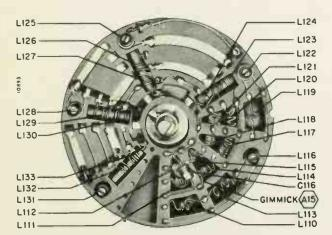
Figure 28. View of Oscillator-Mixer Rotor Disc in VHF Tuners 94E144-13, -19, -24 and -26.
