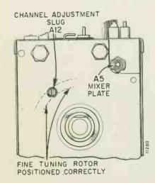
Figure 42. Front View of 94E163-1 and -2 Tuners.
