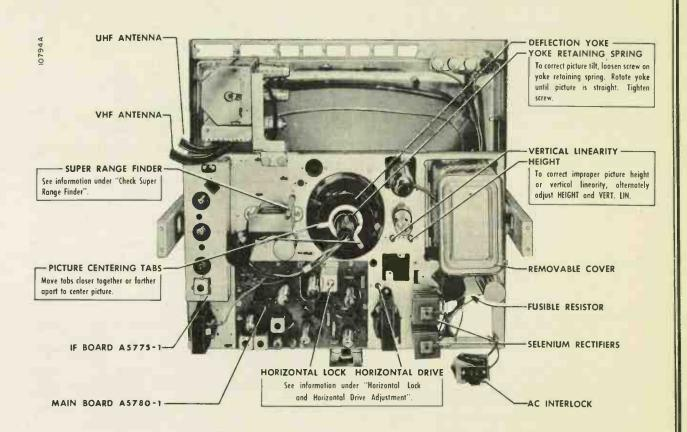
Figure 6. Rear View of Chassis Showing Adjustment Locations.
