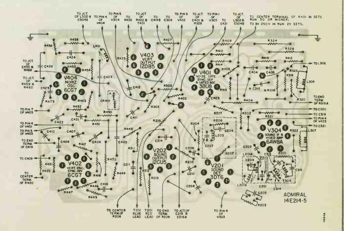
Figure 74. View of Printed Wiring Board AS780-S used in 16R1, 16AR1, 16S1, 16AS1 Chassis. Note: Noise Gate Circuit in Chassis Stamped Run 30 or Higher. Gray Area Represents Printed Wiring; Black Symbols and Lines Represent Components and Connections on Opposite Side. See Service Manual No. STS97-2 for Other Printed Wiring Views.
