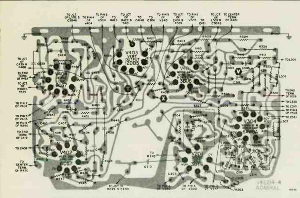
Figure 51. View of Printed Wiring Side of Main Board A5780-4 Used in 16U1C, 16AU1C, 16W1C and 16AW1C Chassis. Gray area represents printed wiring; black symbols and lines represent components and connections on opposite side.
