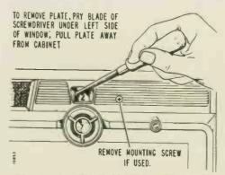
Figure 9. Method of Removing Snap-in Plate Without Mounting Screw.
