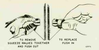
Figure 55. Method of Removing and Replacing Nylon Insulating Inserts.
