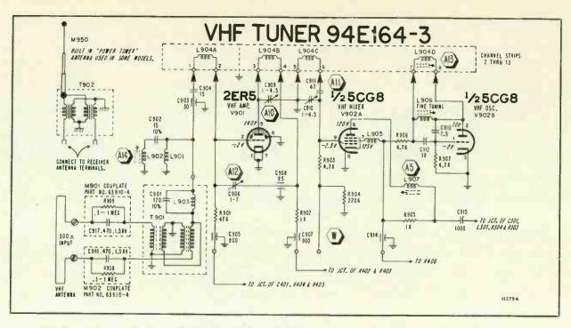
Figure 62A. VHF Tuner 94D164-3 used with Television Chassis 15A2C. Except for Tuner, Chassis 15A2C is the same as Chassis 15A2.
