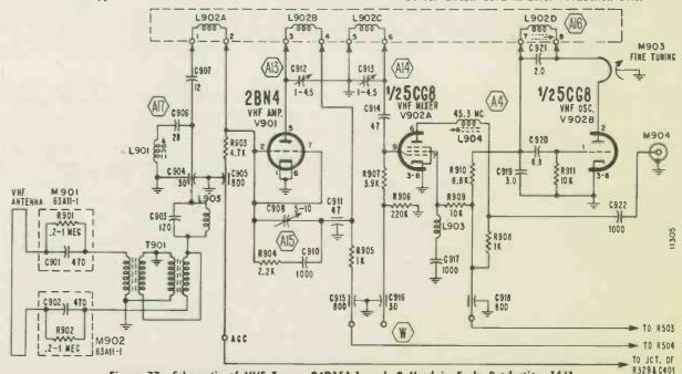
Figure 77. Schematic of VHF Tuners 94D151-1 and -2 Used in Early Production 16J1, 16K1, 16R1CB and 16S1CB Chassis. See Figures 81 and 83 for VHF Tuners 94D151-5 and -6 Used in Later Production Chassis.
