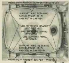
Figure 33. Rear View of Models using Chassis 15A2, 15A2C, 15B2, 15B3 and 15UA2 with Chassis Removed.
