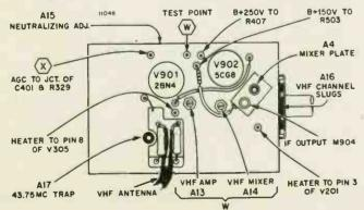
Figure 37. Top View of VHF Tuners 94D151-1 and -2 Showing Adjustment Locations.
