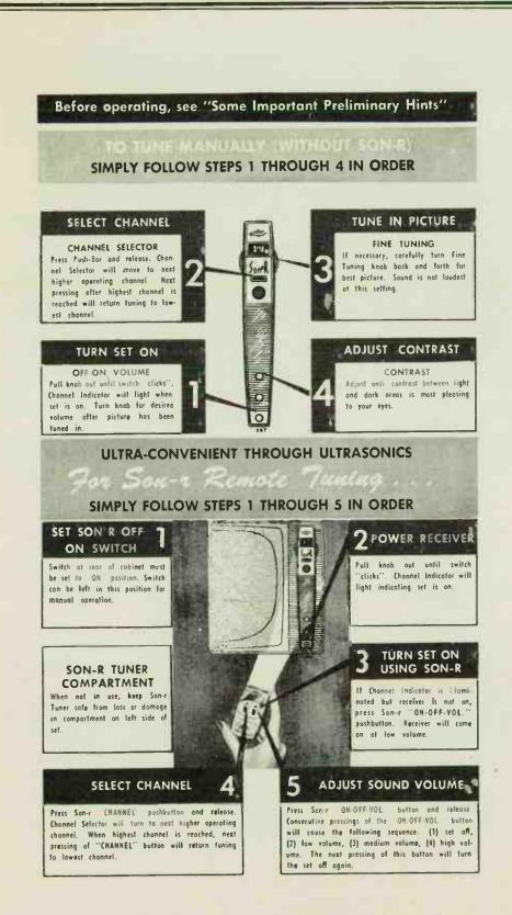
Figure 25. Tuning Instructions for Models using TV Chassis 15B3.
