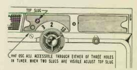
Figure 12. Front View of VHF Tuner In Console Models
