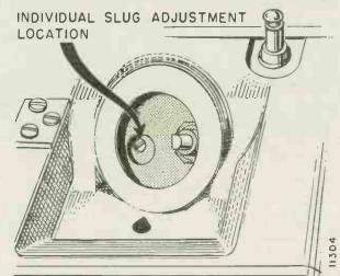
Figure 32. Partial Top View of Models using Chassis 15D1B Showing Channel Adjustment Slug Locations.
