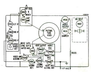
TUBE LOCATIONS AND HEATER CIRCUIT
