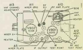
Figure 45. Top View of VHF Tuner 94D164-3
