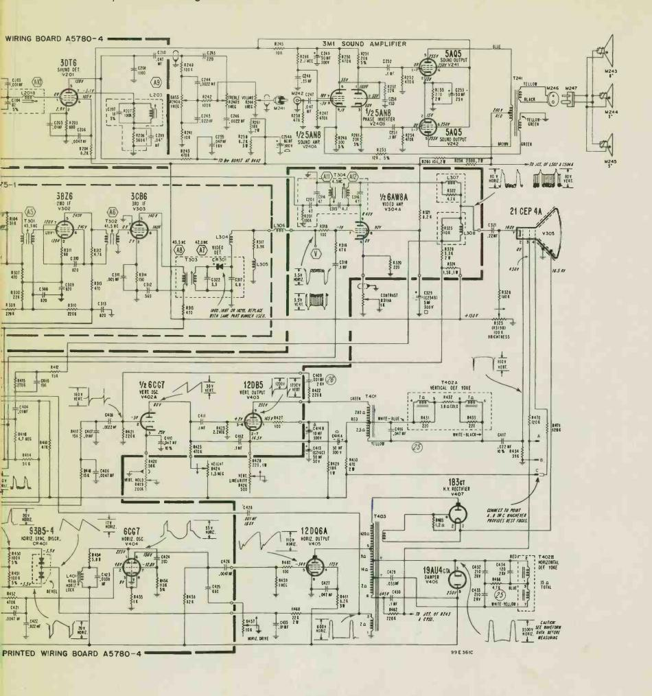
Figure 72. Schematic for 16J1, 16J1C, 16K1, and 16K1C Television Chassis Stamped Run 15 Throughber. See Figure 57 for Horizontal Output Circuit in Sets V
