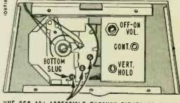
VHF OSC. ADJ. ACCESSIBLE THROUGH EITHER OF THREE HOLES. WHEN TWO SLUGS ARE VISIBLE ADJUST BOTTOM SLUG
