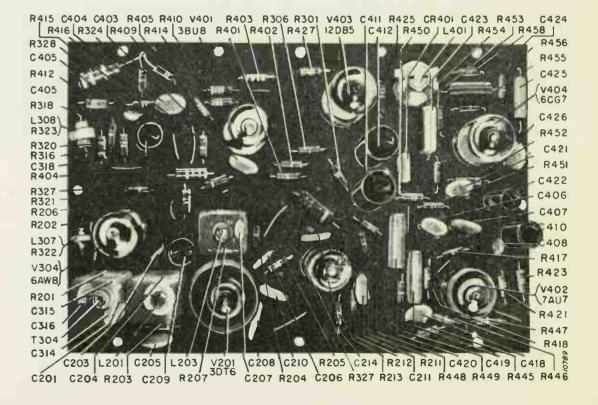
Figure 50. View of Component Side of Printed Wiring Board A5780-1 Used in All Chassis
