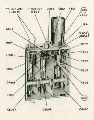
Figure 61. Side View of UHF Tuner 94D162-3 with Cover Removed, Location of components and adjustments shown.
