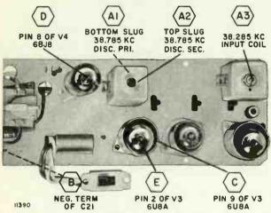
Figure 50, Partial Top View of Remote Amplifier Chassis 4G3 Showing Alignment Points and Adjustment Locations.
