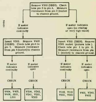
Figure 45. Simplified Test Procedures for Locating an Open Circuit Heater Tube in Sets With Push-Pull Sound Amplifier. Note V801 in VHF-UHF Sets Only.
