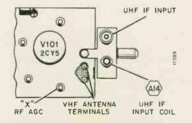
Figure 48. Top Rear Partial View of VHF Tuner 94E163-2 Showing UHF IF Input and UHF IF Input Coil Adjustment, A14.
