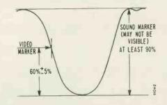
Figure 47. Ideal Overall VHF and IF Response Curve.
