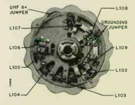
Figure 27. View of Antenna Rotor Disc in VHF Tuners 94E144-9, -22, -27 and -30.
