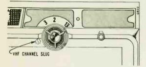
Figure 13. Front View of VHF Tuner in Console Models With Son-R Tuning. Escutcheon Plate Removed.
