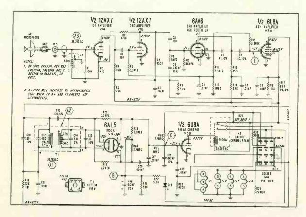
Figure 62B. Schematic for 4H3 Remote Control Amplifier Chassis. NOTE: Chassis 4H3 used with television chassis 15B2.
