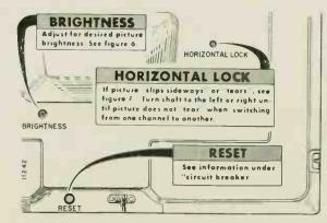
Figure 29. Auxiliary Controls; Chassis 15A2, 15A2C, 15B2, 15B3 and 15UA2.
