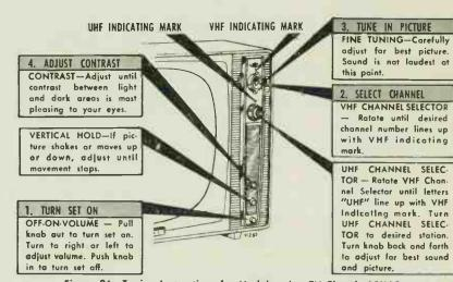
Figure 26. Tuning Instructions for Models using TV Chassis 15UA2.
