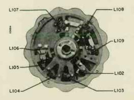
Figure 26. View of Antenna Rotor Disc in VHF Tuners 94E144-13, -19, -24 and -26.
