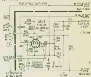
Figure 76. Sync Separator and Gated AGC Circuit Used in 16R1, 16AR1, 16S1 and 16AS1 Chassis Stamped Run 29. See Figure 81 for Circuit Used in Later Production Sets.
