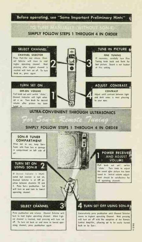
Figure 24. Tuning Instructions for Models using TV Chassis 15B2.
