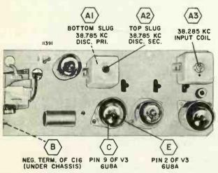
Figure 51. Partial Top View of Remote Amplifier Chassis 4H3 Showing Alignment Points and Adjustment Locations
