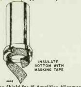
Figure 35. Special Tube Shield for IF Amplifier Alignment and IF Response Curve Check.
