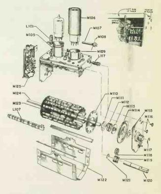
Figure 59. Exploded View of VHF Tuners 94E163-1 and -2. Partial illustration shows placement of detent spring and detent roller.
