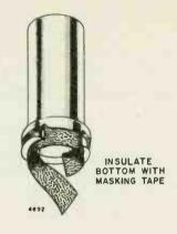
Figure 19. Special Tube Shield for IF Alignment and IF Response Curve Check.
