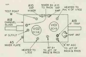
Figure 44. Top View of VHF Tuners 94E163-1 and -2 Showing Alignment Points and Adjustment Locations.
