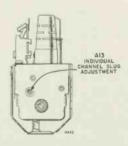
Figure 43. Front View of 94D164-3 Tuner.
