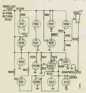
Figure 40. Simplified B+ Distribution Diagram for VHF
