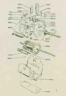
Figure 79. Exploded View of VHF Tuners 94D151-5 and -6 Used in Later 16J1, 16K1, 16R1CB and 16S1CB Chassis.
