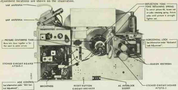
Figure 30. Rear View of Chassis 15UA2 Showing Adjustment Locations.
