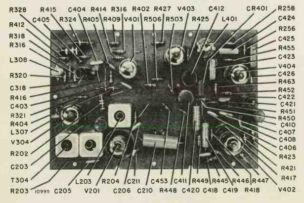
Figure 52. View of Component Side of Printed Wiring Board A5780-4 Used in 16U1C, 16W1C, and 16AW1C Chassis.
