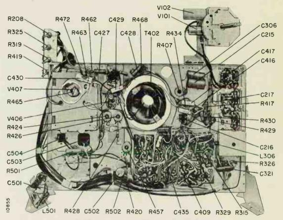
Figure 53. Wiring Side of Chassis With Single Ended Sound Amplifier.
