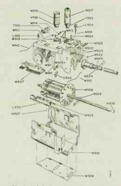
Figure 78. Exploded View of VHF Tuners 94D151-1 and -2 used in early 16J1, 16K1, 16R1CB and 1651CB Chassis.
