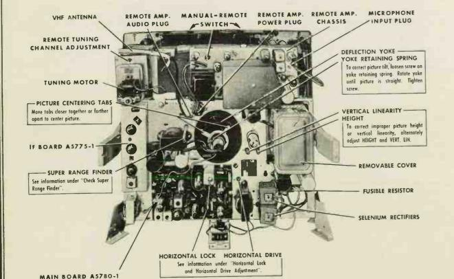
Figure 8. Rear View of 16J1 and 16K1 Chassis Showing Adjustment Locations.
