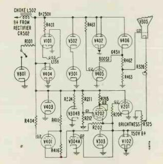
Figure 41. Simplified B+ Distribution Diagram for VHF-UHF Receivers With Single Ended Sound Amplifier.
