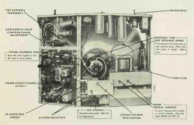
Figure 31. Rear View of Chassis 15D1B Showing Adjustment Locations.
