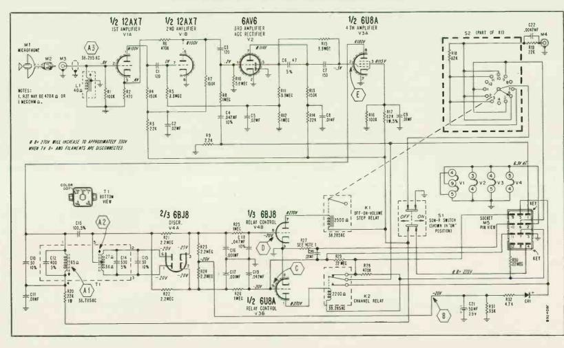
Figure 63. Schematic for 4G3 Remote Control Amplifier Chassis. NOTE: Chassis 4G3 used with television chassis 15B3.
