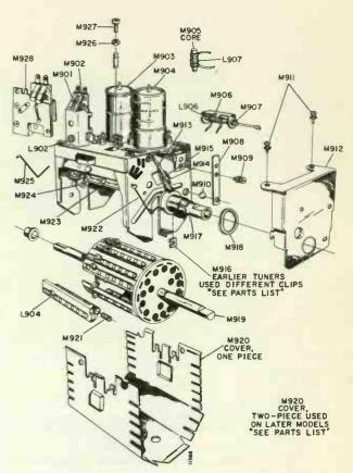
Figure 60. Exploded View of VHF Tuner 94D164-3.
