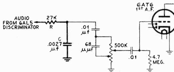
FIG. 4.—The RC de-emphasis circuit of Montgomery Ward Model 74 WG-2505A.
