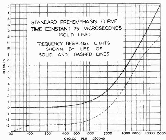
FIG. 1.—Pre-emphasis characteristic curve established by the FCC.
