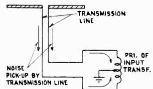
cancel each other. Hence, the total noise voltage induced in the secondary of the input transformer is effectively zero.
