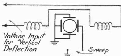
voltage, if such is used, to the horizontal deflecting plates and use a combination of magnetic and electrostatic deflection. Note that the free vertical plate is grounded. The sweep voltage connections to the horizontal plates may be made externally, if an external sweep voltage is used, or may be made internally, if an internal sweep voltage is used. In the latter event, ignore the connections shown to the horizontal plates.
