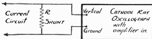
is shown in figure 152. The cathode-ray tube is arranged for independent voltages to the horizontal and vertical plates. The vertical
