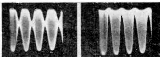
rect frequency adjustment, that is sweep frequency adjustment, results in a pattern such as that shown in figure 387. When the correct sweep frequency adjustment is reached, in this case being a sub-multiple equal
