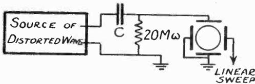
Fig. 201. Circuit for checking phase distortion.
