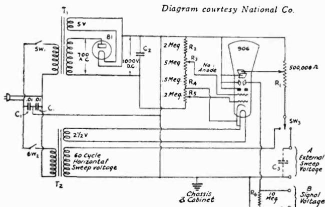
trols are mounted upon the front of the housing and upon the right side. The spot intensity and spot focusing controls are mounted upon the front panel; also the power supply switch. The horizontal and vertical deflection plate connection posts are mounted on the side; also the potentiometer controlling the amplitude of the voltage supplied to the horizontal plates. The unit is equipped with a 60-cycle
