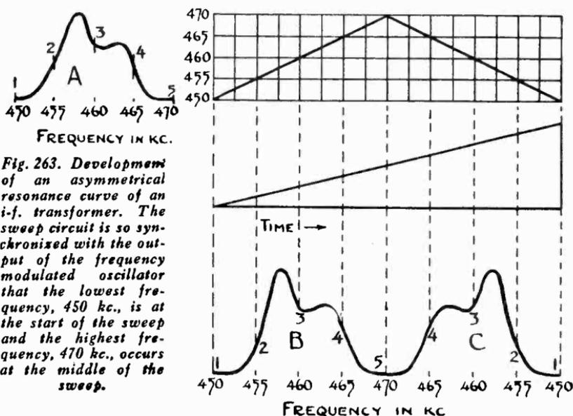
*Fig. 263. Development of an asymmetrical resonance curve of an i-f. transformer. The sweep circuit is so synchronized with the output of the frequency modulated oscillator that the lowest frequency, 450 kc., is at the start of the sweep and the highest frequency, 470 kc., occurs at the middle of the sweep.*
