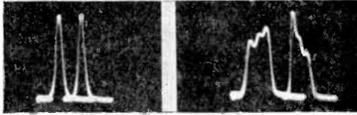
modulating unit, also is important. If the polarity is incorrect, the pattern is greatly distorted. Examples are shown in figures 316 and 317. The image shown in figure 316 is for correct polarity of the impulse generator signal and all other adjustments correct. The pattern shown in figure 317 is for the same signal under exactly the same conditions, except that the polarity of the signal obtained from the impulse generator has been reversed.
