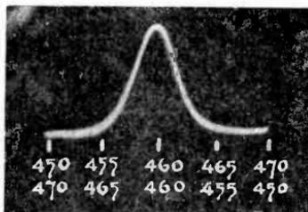
the curve. The variation in amplitude is the same both sides of the single resonant frequency, hence the spot positioning for corresponding frequencies of each pair is the same and a single line pattern appears.
