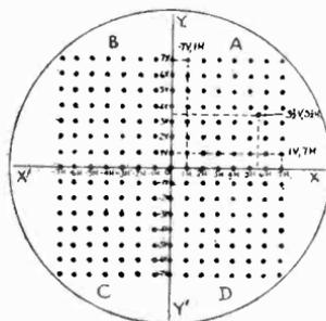
however, the voltage applied to the plates changed in very small increments, the spot would appear so close to the previous position that when recurrent at a rate, say 16 to 20 times per second, the entire active area would appear fluorescent.
