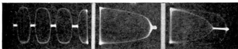
The wave envelope and trapezoid patterns are shown in Figs. 398 (left) and 399 (middle). Fig. 400 (right) shows the type of trapezoid pattern secured when the audio voltage for the horizontal displacement is secured from the input to the speech amplifier, instead of from the modulator, as in Fig. 399.
