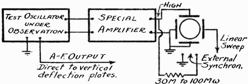
Fig. 224. Circuit used for checking the modulated and unmodulated carrier outputs and the a-f. output of a test oscillator.
