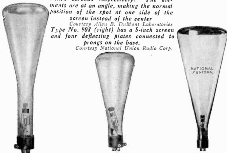
cerned, but differs in that the electron emitter, the cathode, is not heated and the electrons are drawn from the cathode by a nearby element (anode), to which has been applied a voltage of from 10,000 to 20,000 volts, which is positive with respect to the cathode. In the hot-cathode type of tube, the emitter emits electrons freely.
