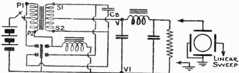
*Fig. 367. Schematic diagram of full-wave synchronous vibrator.*
