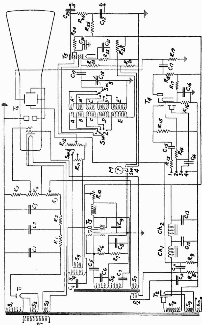
Fig. 279. Schematic diagram of the Egert Model VRO oscilloscope.
