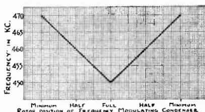
Obviously, the correct setting of the frequency modulating condenser for the correct mean frequency is about half capacity. The increase from half to maximum capacity serves to produce the change in frequency from the mean figure to the lowest frequency. The decrease from half capacity to minimum capacity serves to produce the change in output frequency from the mean frequency to the highest frequency.
