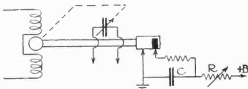
cal connection with the stationary contact during 180 degrees of the 360-degree arc made by the rotating condenser rotor. A high d-c. voltage is fed to condenser C through resistor R, charging the condenser.
