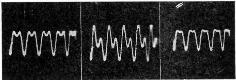
*Figs. 157, left, 158, middle, 159, right. The amplitude of the wave in Fig. 155 was reduced and caused the reduction of the dip in the composite wave of Fig. 157. Compare Fig. 156. By shifting the phase between the waves of Figs. 154 and 155, the composite wave of Fig. 158 was obtained. Fig. 159 was obtained by reducing the amplitude of the wave of Fig. 154 and making that of Fig. 155 about one-half its amplitude. Compare Figs. 156 and 157.*
