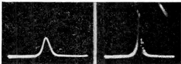
quency is indicated or spotted upon the pattern or image by the point where the two curves cross each other. A pattern of this type indicates that the response of the circuit is better to frequencies one side of the mean frequency than to frequencies on the other side of the mean frequency.
