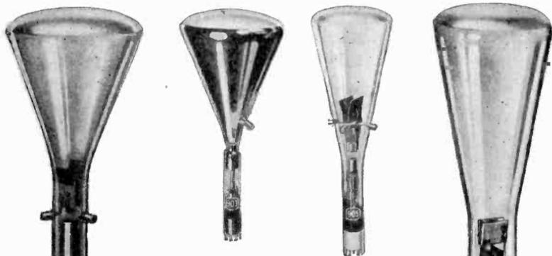
Type 903 has a 9-inch screen and is designed for electromagnetic deflection.
