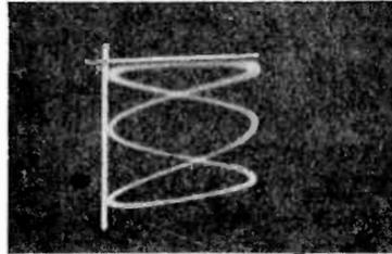
deflection plates must be three times the standard, or the frequency of the standard is to the unknown as 1 is to 3, and the frequency of the unknown is 9000 cycles.
