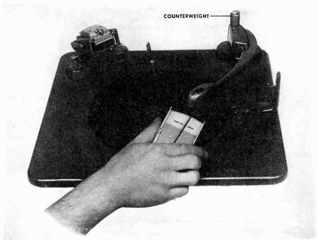
FIGURE 10. MEASURING HORIZONTAL FRICTION
