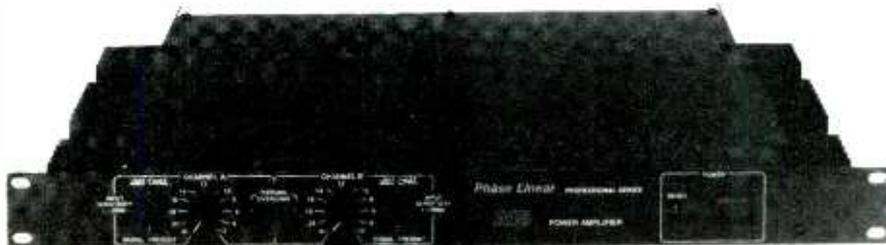
Housed in its compact, 1 1/4-inch high chassis, the amplifier is a modular, fully complementary device. Functional features include LED Fault, Signal Present and Thermal indicators; balanced/unbalanced inputs; and automatic mono input. Total harmonic distortion is quoted at less than 0.05% from 20 Hz to 20 kHz.
