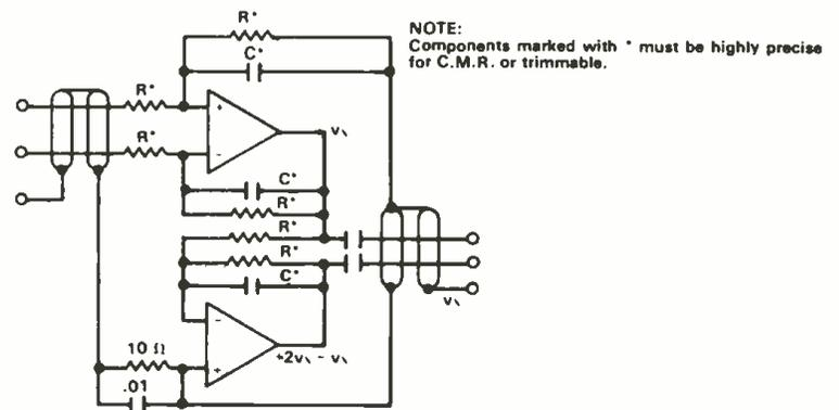
Figure 7 - An Electronic 6 dB Step-Up Output with Forward Referenced Isolation and Differential Input
