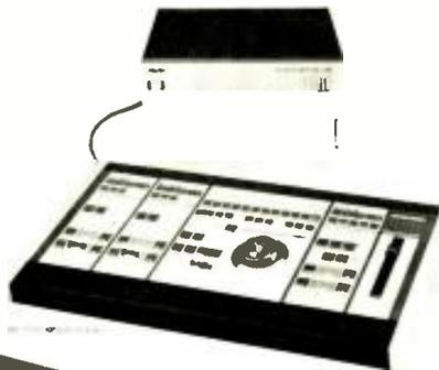
Sony broadcast U-matic videocassette recorders to store the digital information, the editor allows the sequencing and combination of varied material for a finished product with extremely accurate, undetectable edits. The preview function of the DAE-1100 makes editing fool-proof, and lighted buttons which flash in sequence show the order of operation.
