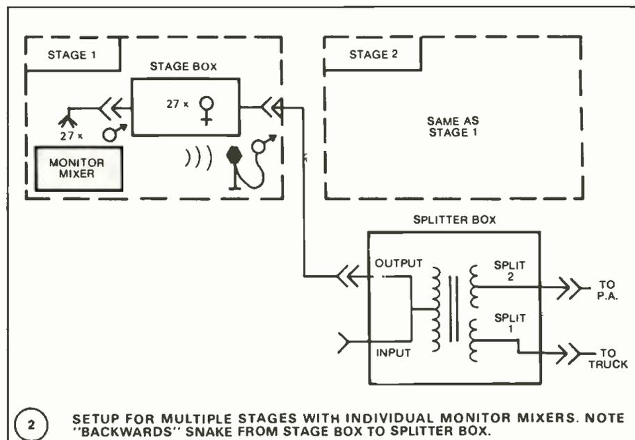
2 SETUP FOR MULTIPLE STAGES WITH INDIVIDUAL MONITOR MIXERS. NOTE "BACKWARDS" SNAKE FROM STAGE BOX TO SPLITTER BOX.
