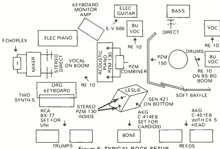
Figure 6: TYPICAL ROCK SETUP
