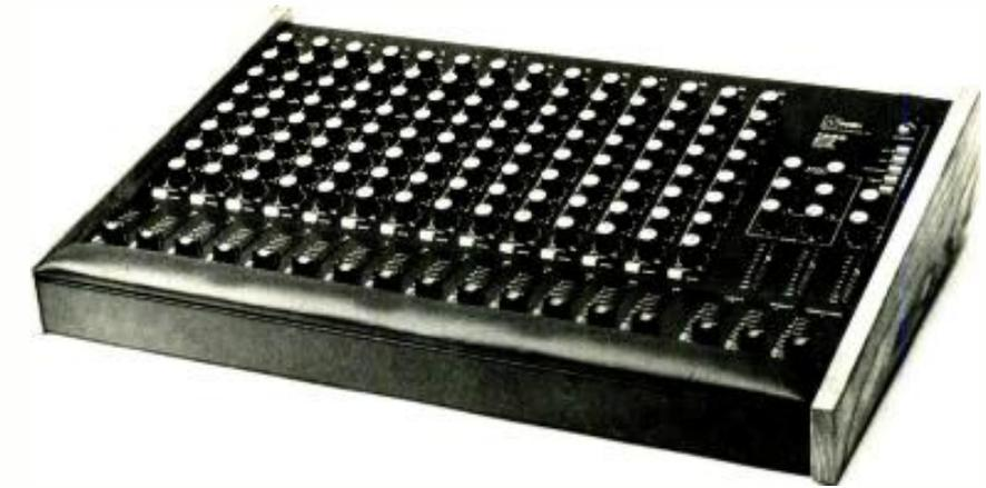
and functions include: extensive headphone monitoring system for solo and function monitoring with loud 5-watt headphone amp with gain control, balanced (D3M) and unbalanced (1/4" phone) line level outputs for left/right mains and monitor, slide-type master gain (left/right) and monitor master controls with LED VU level indicators, effects and auxiliary master sends and returns with hi or low level return jacks (effects return) and panning for both effects and auxiliary returns, plus much more.
