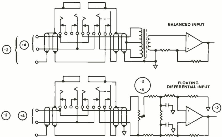
Figure 9 - Isolation Inputs with Bi-Level Patching
