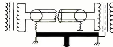
Figure 2A: BALANCED TO BALANCED COUPLING
