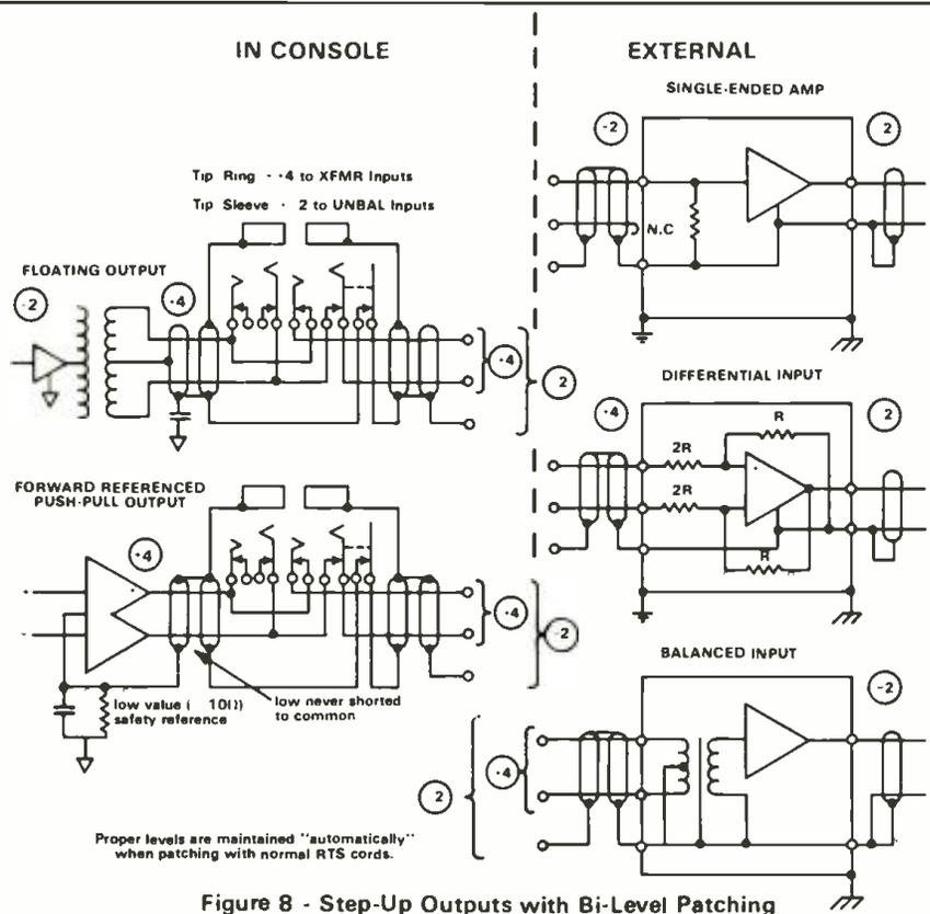
Figure 8 - Step-Up Outputs with Bi-Level Patching
