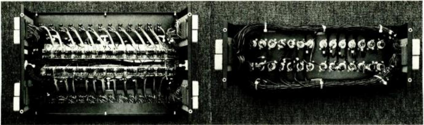
(Left) 27-pair Splitter Box built by McCune Sound. Note ground lift switches and transformer mounting rails. (Right) 27-pair Stage Box with "loopthrough" connections. Photographs courtesy of McCune Sound, San Francisco, California
