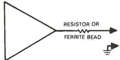
AMPLIFIER HOOK-UP SHOWING BUILT-OUT RESISTOR OR FERRITE BEAD
