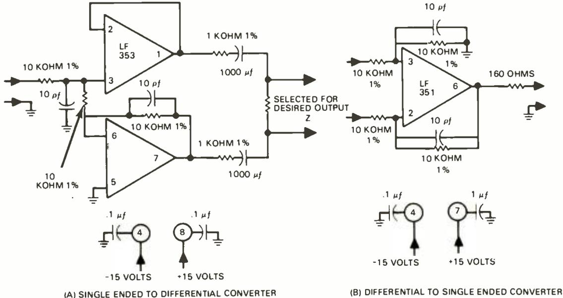
Figure 5: CIRCUITS FOR CONNECTING UNBALANCED TEST EQUIPMENT TO BALANCED DUT'S
