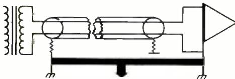
Figure 2B: BALANCED TO UNBALANCED COUPLING
