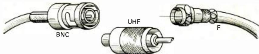
**CONNECTORS:** There are three basic connectors you will find in video applications: the BNC, the F, and UHF. The UHF connector is generally used with a composite video signal and is wired to coax type cable (RG-58, RG-59). The F type connectors and the BNC connectors are typical for interconnecting RF signals, carrying both modulated video and audio.
