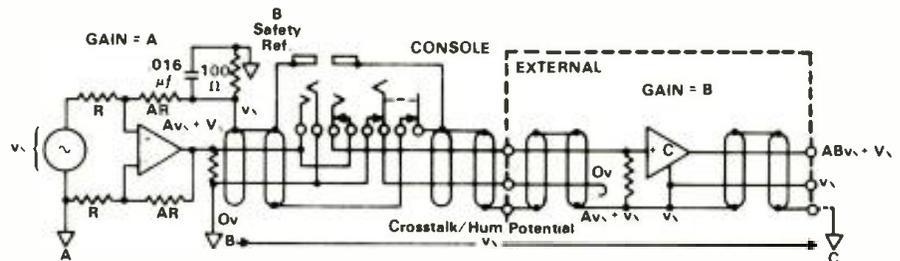
Figure 6 - Forward Referenced Amplifier
