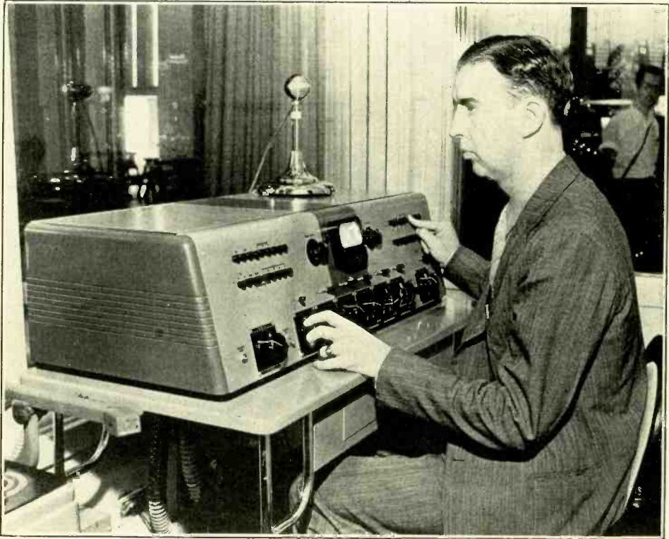
• This RCA "Consolette" control desk used in the Broadcast and Public Address Center at the New York World's Fair suggests a design for a de luxe medium-power amateur transmitter.
