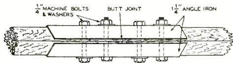
Here is a very neat method of joining 2 x 2 stock for antenna masts. It makes a very strong butt joint.
