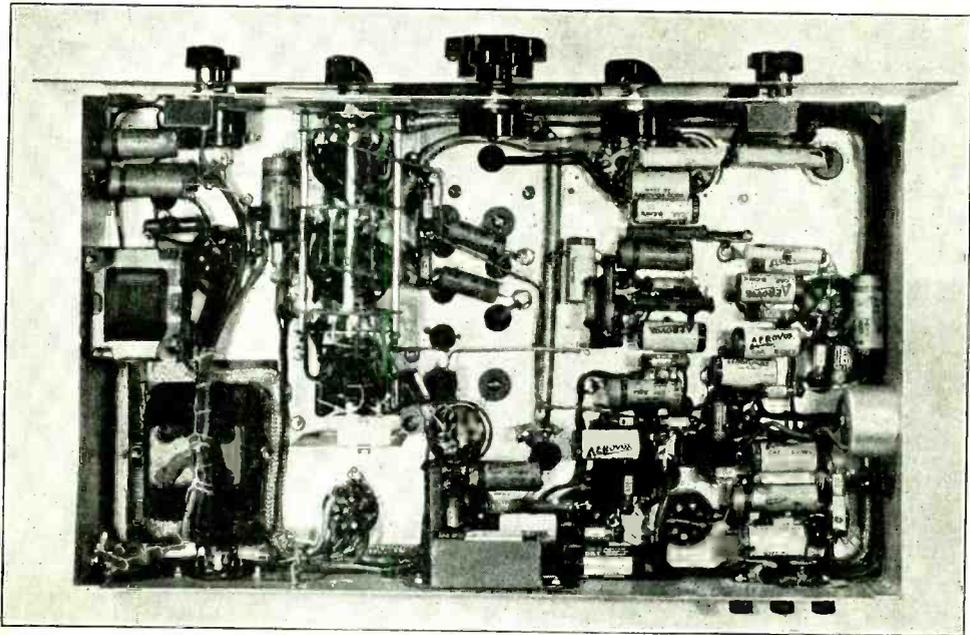
Under-Chassis View of the Completed Receiver
