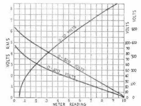
Fig. 6. Calibration Curve of Voltmeter
