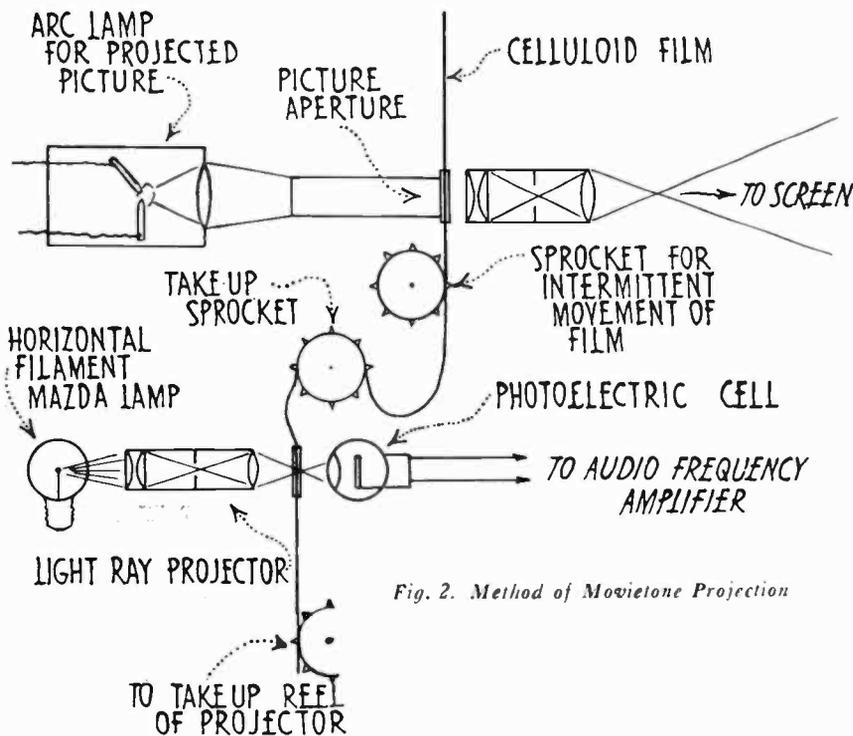
Fig. 2. Method of Movietone Projection
