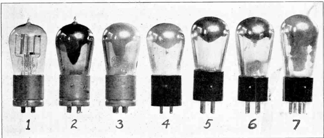
Fig. 1. Progressive Development of the "A" Tube
