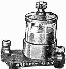
Used on the B-T Power Six, also Counterphase sets for balancing or neutralizing—a process much easier and certain when the precision condenser is used. Capacity adjustment is gradual and once set is permanent.
