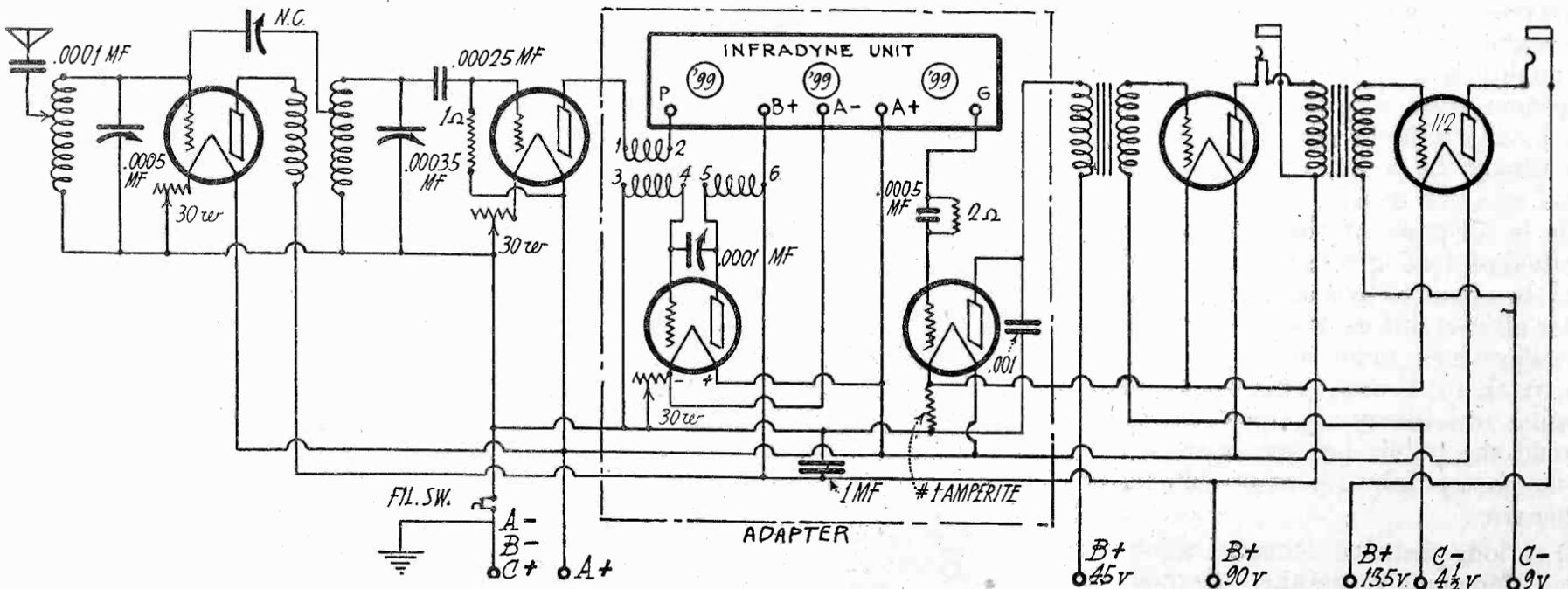
Browning-Drake Circuit With Infradyne Adapter Permanently Wired.
