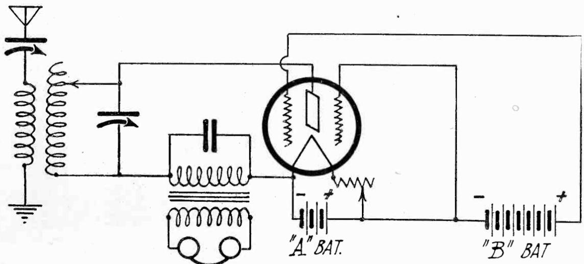
Fig. 2. Complete Four-Electrode Tube Circuit.
