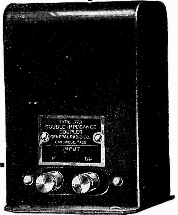
While the use of double impedances is not new in principle the General Radio Type 373 Double Impedance Coupler is unique in design and performance. To facilitate installation the complete unit, consisting of two impedances and a fixed condenser, is contained within a metal shell. It is connected in precisely the same manner in an audio amplifier circuit as a transformer.
