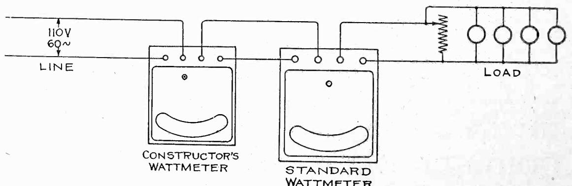
Fig. 8. Calibration Set-up.
