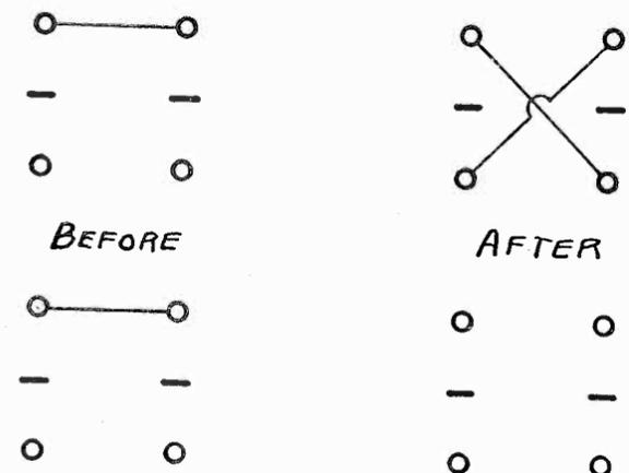
If the connections on the "OSCLR-DET" key switch on the tube control panel are changed as shown in the diagram, this switch may be used to reverse the tickler connections when on the "DET" position instead of cutting out and shorting the tickler coil as it does normally. Simply remove the two wires shown in Fig. 1 and connect the two shown in Fig. 2.
