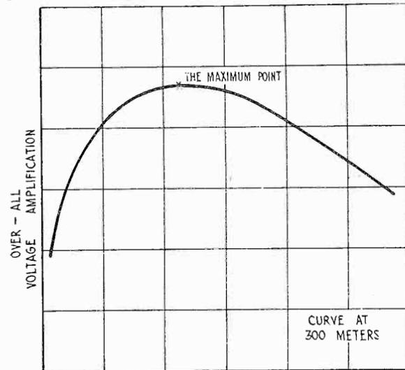
Fig. 2. Curve of Over-all Amplification with Primary Turns at Critical Regeneration. MAINTAINING CRITICAL REGENERATION WITH RESISTANCE CONTROL
