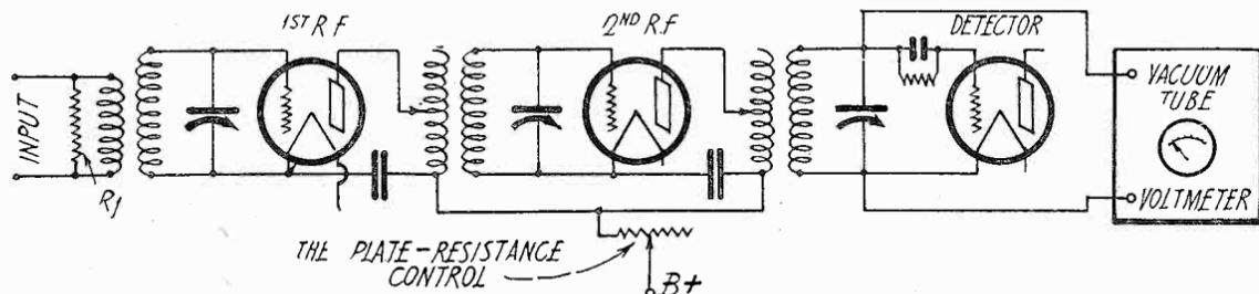
Fig. 1. Experimental Set-up for Determining Best Ratio of Plate Control to Size of Primary. The value of the output is measured by the vacuum-tube voltmeter. Output divided by input gives the relative amplification. A series of such readings at 300 meters for various primary taps and plate resistances may be plotted in a curve, Fig. 2, to indicate what size of coil gives maximum amplification.
