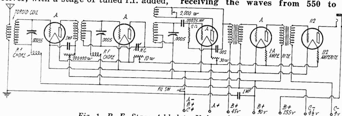
Fig. 1. R. F. Stage Added to Universal Receiver.
