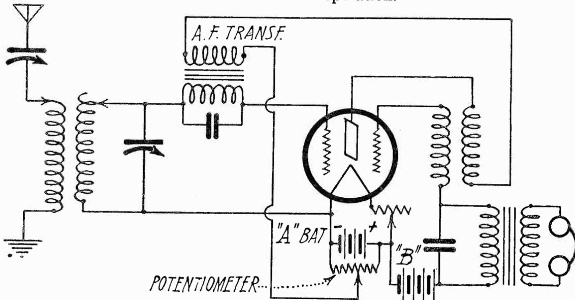
Fig. 4. R. F. Amplifier and Rectifier Circuit.
