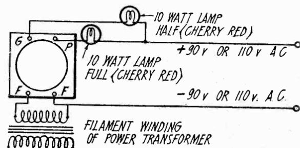
Circuit for Testing Rectifier Tube.
