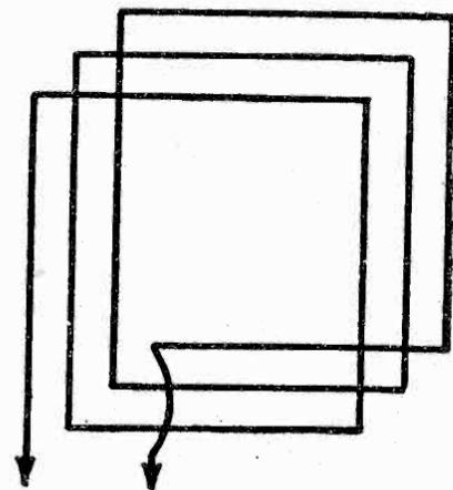
Fig. 2. Solenoid Loop.
