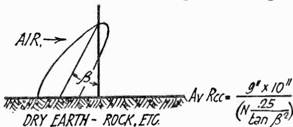
Fig. 2a. Propagation Over Imperfect Conductor.
