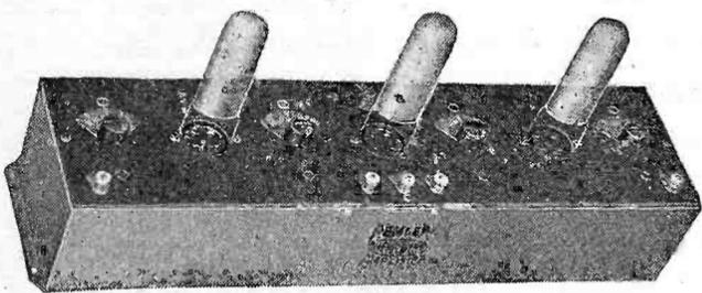
Front view, showing bakelite panel and copper case.
