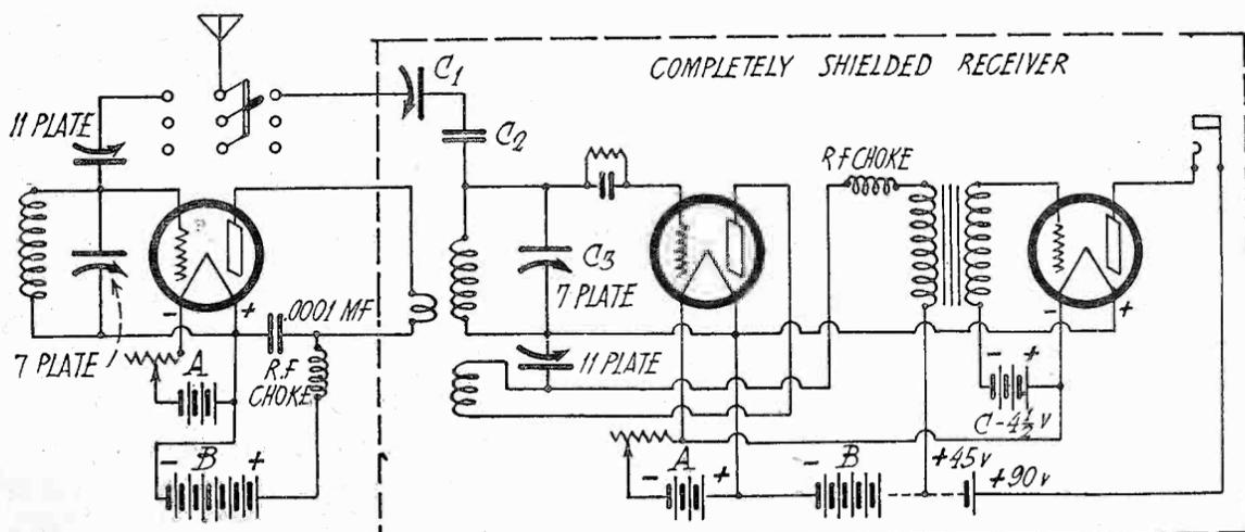
Circuit Diagram for Browning-Drake 30 Meter Receiver.
