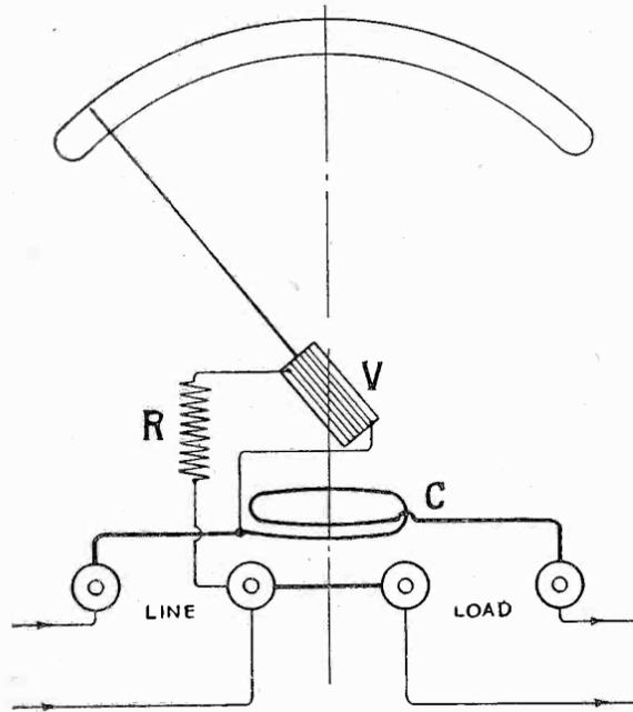
Fig. 3. Circuit Diagram of Wattmeter.
