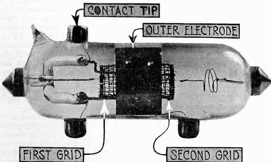
Fig. 1. The "MO" Four-Electrode Tube.
