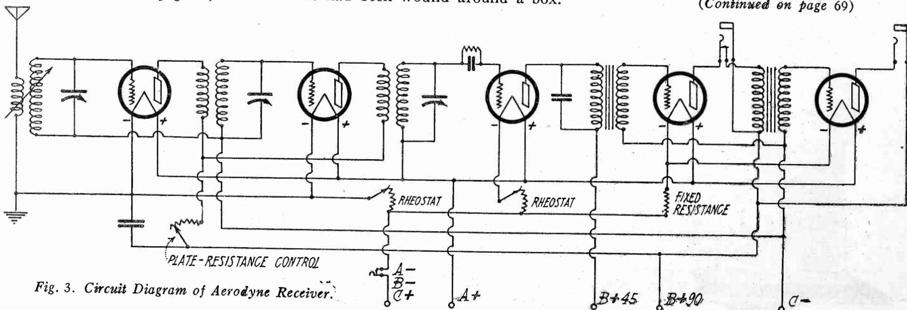
Fig. 3. Circuit Diagram of Aerodyne Receiver.
