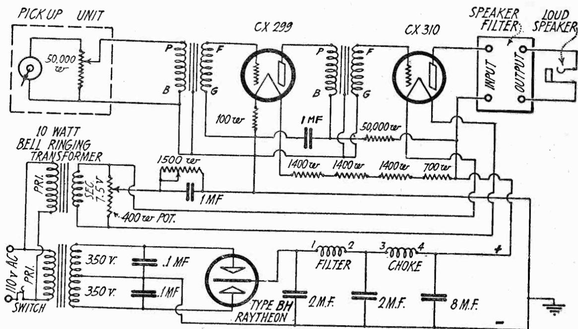
Fig. 1. Schematic Wiring Diagram of Electric Phonograph
