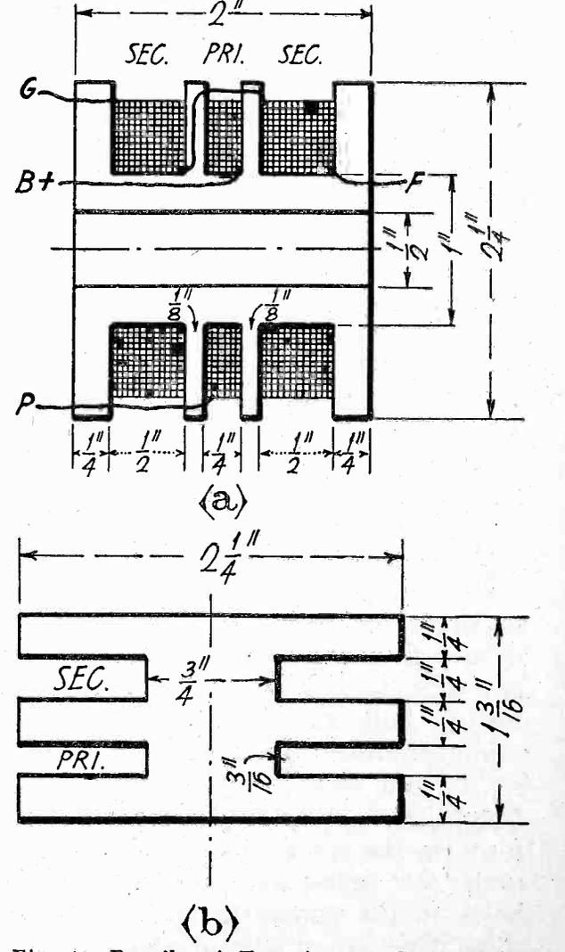
Fig. 4. Details of Transformer Construction. anical assembly of the wooden or bakelite spools for the intermediate frequency
