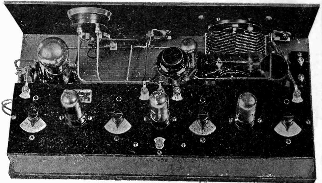
Separate Infradyne Adapter With Switch Control.
