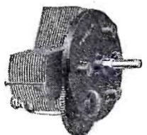
Remler Twin Rotor Condenser
