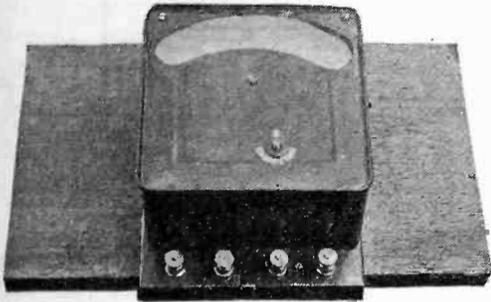
Fig. 1. Completed Wattmeter as Made by Author.
