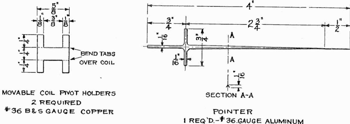
Fig. 4. Details of Pivot Holder and Pointer.
