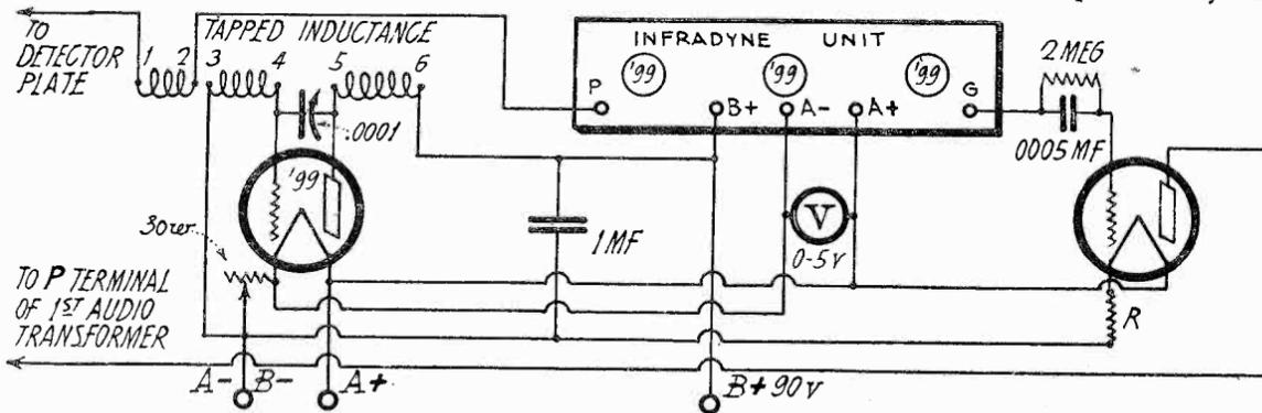
Circuit Diagram of Separate Infradyne Adapter.
