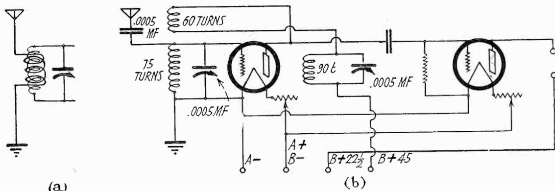
Fig. 1. Adaptation of Superdyne Circuit for Long Wave.
