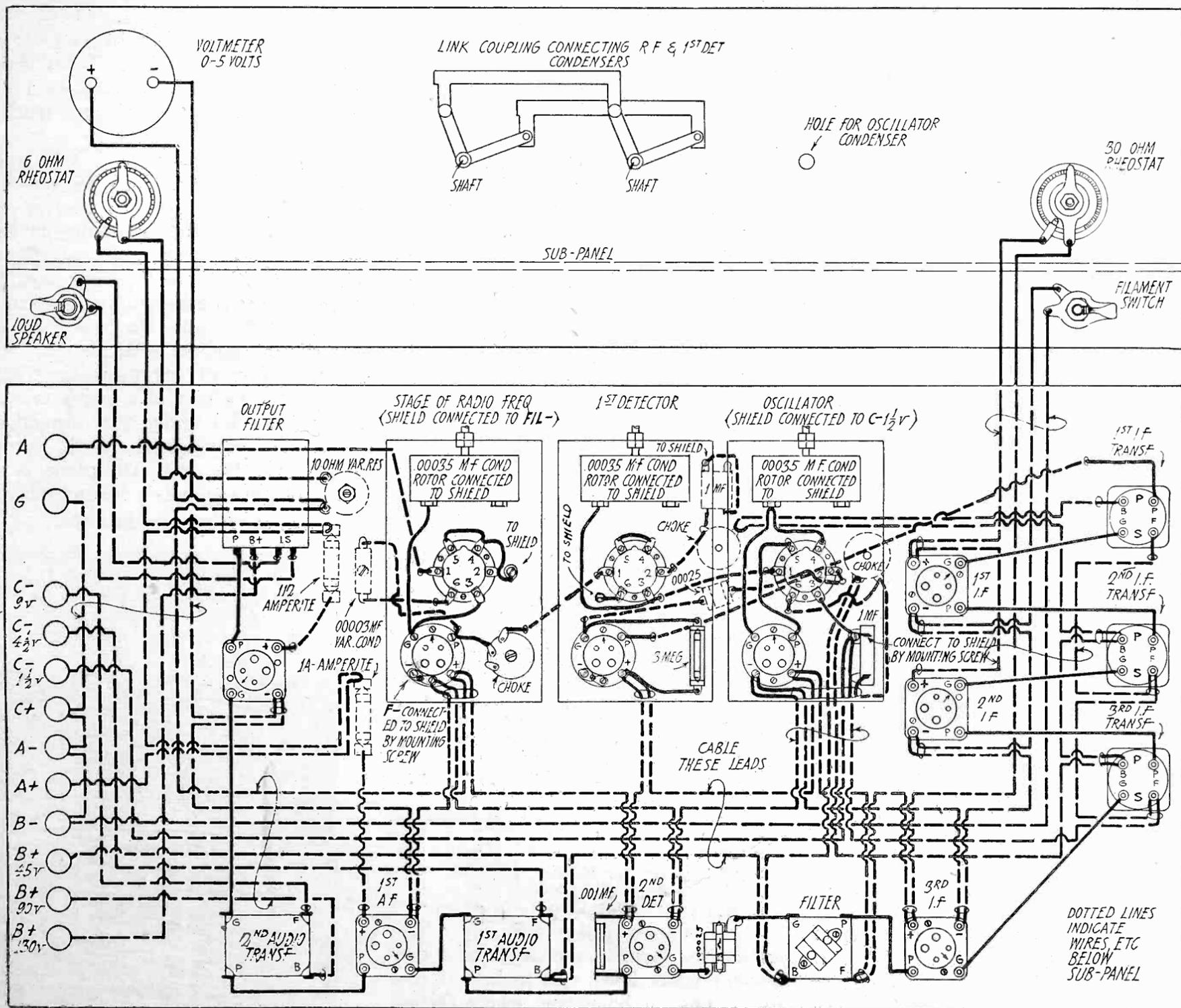
Fig. 3. Pictorial Wiring Diagram.
