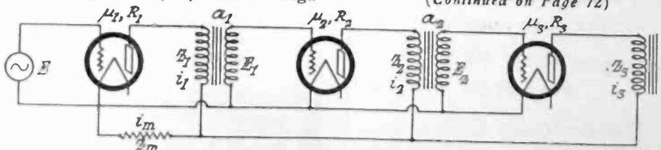
Fig. 4. Typical Audio Frequency Amplifier.
