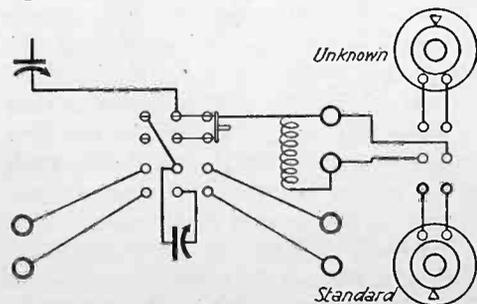
Fig. 1. Connections for Condenser Calibration.
