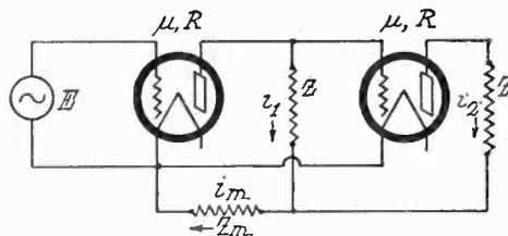
Fig. 1. Two-Stage Direct Coupled Amplifier.
