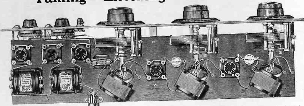
place on the dial. The selectivity of the circuit is accompanied by a remarkable volume, due to a big gain per each stage of radio frequency and to the employment of the powerful KARAS HARMONIK TRANSFORMERS for the two audio stages.
