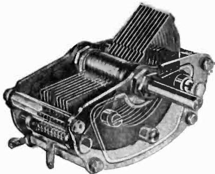
the capacity value nor the smoothness of operation. It is made with either aluminum or brass plate, as desired. The maximum capacity of the six sizes are 100, 150, 250, 300, 350 and 500 mmfd. respectively.
