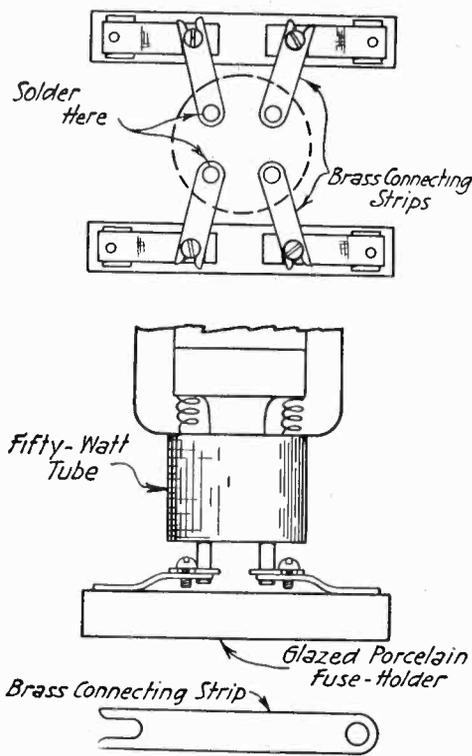
Fig. 1. Home-Made Socket for 50-Watt Tube.
