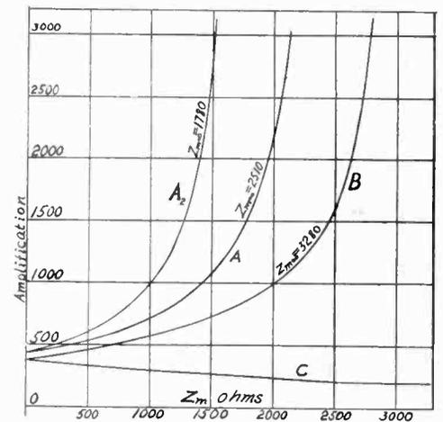
Amplification for Various Values of Common Impedance in Plate Circuit.
