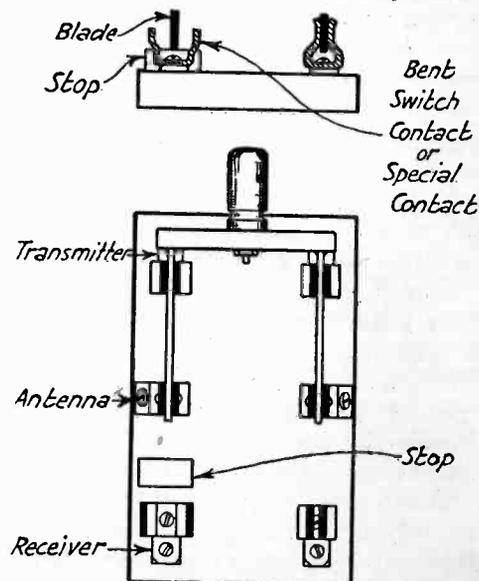
Fig. 2. Modification of Switch to Hold Service Condenser.
