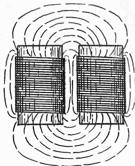
Fig. 2. *Electromagnetic Field of Astatic Pair.*
