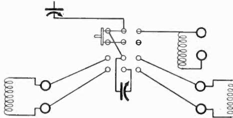
Fig. 3. Connections for Checking Coils.
