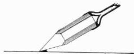
Fig. 2. Wrong Method of Applying Soldering Iron to Work.
