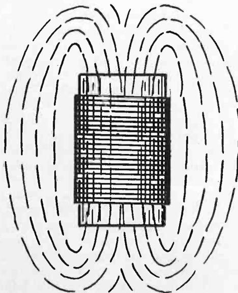
Fig. 1. *Electromagnetic Field of Solenoid.*
