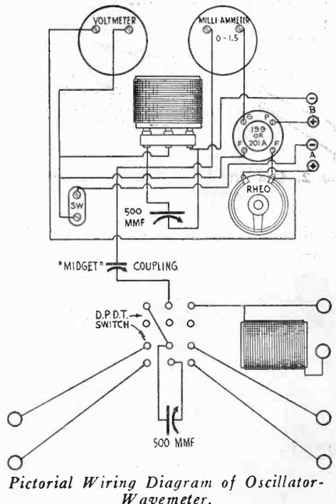
Pictorial Wiring Diagram of Oscillator-Wavemeter.
