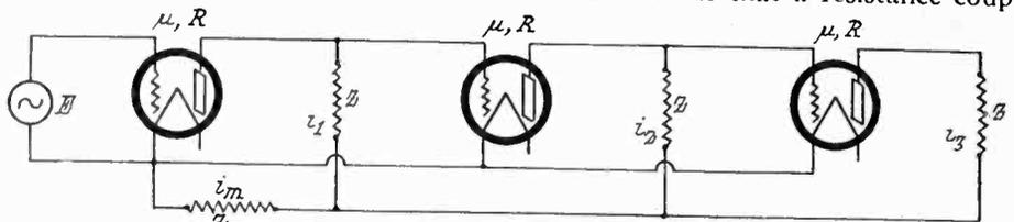
Fig. 2. Three-Stage Direct Coupled Amplifier.
