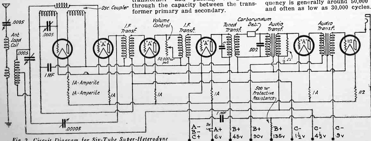
Fig. 2. Circuit Diagram for Six-Tube Super-Heterodyne With One Crystal Detector.
