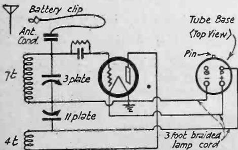
Circuit Diagram for Short Wave Adapter.
