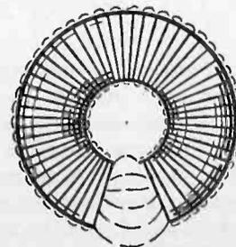
Fig. 3. *Electromagnetic Field of Toroidal Coil.*
