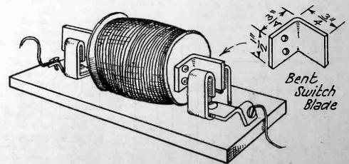
Fig. 2. Method of Mounting R.F. Choke.
