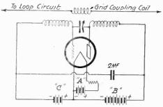
Fig. 3. Oscillator Used in Best Superheterodyne, with Series Condenser.
