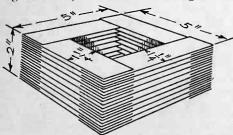
Fig. 2. Dimensions of Core for Battery Charger Transformer.
