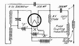
Fig. 5. Stabilized Oscillator, Using Tuned Grid Circuit.
