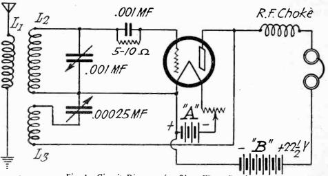
Fig. 1. Circuit Diagram for Short-Wave Receiver.
