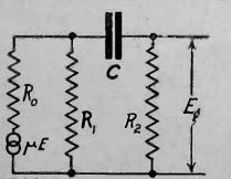
Fig. 1. Circuit Equivalent to Resistance Coupled Amplifier with Stopping Condenser.
