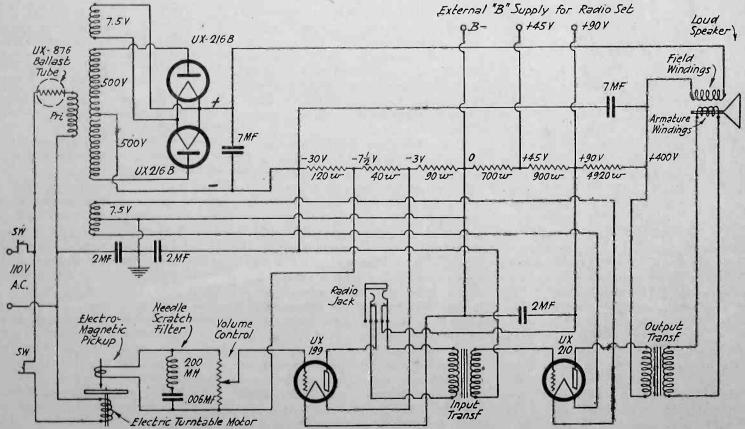
Fig. 1. Schematic Wiring Diagram of Panatrope.
