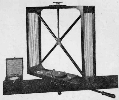
Kolster Loop Developed as Direction Finder for Radio Supervisor's Trucks
