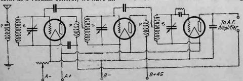
Fig. 2. Conventional Neutrodyne Circuit.
