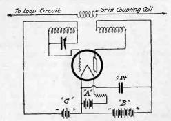
Fig. 2. Tuned Grid Oscillator, With Fixed Plate Coil.
