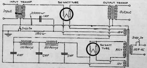
Fig. 4. Circuit for 50 Watt Power Amplifier.
