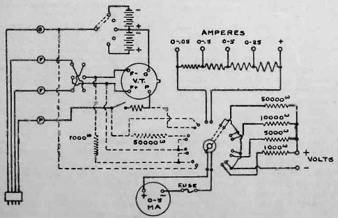
Fig. 2. Circuit Diagram of Testing Instrument.
