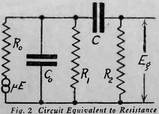
Fig. 2 Circuit Equivalent to Resistance Coupled Amplifier with By-Pass and Stopping Condensers.
