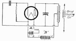
Fig. 4. Oscillator with Tuned Plate Circuit.
