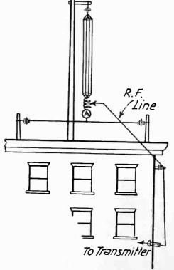
Fig. 2. Position of Antenna Receiver to Radio Frequency Feeder.
