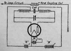
Fig. 1. Oscillator Circuit Most Frequently Used.
