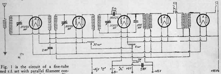
Fig. 1. Schematic Wiring Diagram of Five Tube Receiver for Battery Operation.
