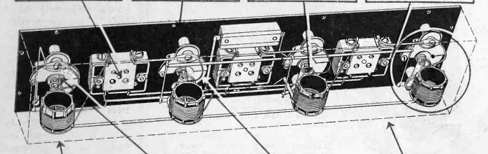
Moulded Bakelite coil forms ribbed to minimize dielectric losses. Coils designed for maximum efficiency and sharp tuning.
