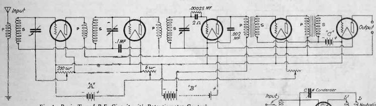
Fig. 1. Basic Tuned R.F. Circuit with Potentiometer Control.
