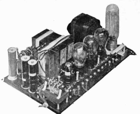
Fig. 2. Rectifier-Amplifier Assembly, Showing Constructional Details.
