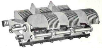
T HIS Continental special triple condenser was designed by Mr. E. M. Sargent for use in the Infra-Dyne Circuit.
