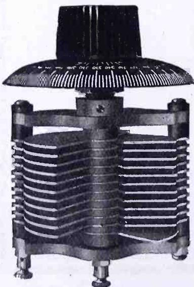
Losses have been reduced to a negligible quantity in the new Cruver condenser designed by G. M. Proudfoot. The stator plates are mounted on two instead of the usual three plates so as to give a loss of but .007 per cent at a capacity of .001 mfd. By means of two scales the coarse adjustment is made by turning the knob to the right on the large scale and the fine adjustment by turning to the left on the small scale. Body capacity effects are eliminated by grounding the rotor plates.
