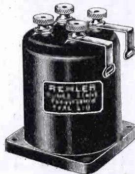
Remler Type 610 tuned stage transformer is designed to work between the last intermediate frequency stage and the detector tube of a super-heterodyne receiver. With a .00025 mfd. condenser it gives maximum amplification at 45,000 cycles and fairly uniform amplification over a range of 3000 cycles on either side thereof. It is made with an air core and primary impedance to match that of a standard dry battery tube.
