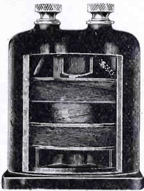
Remler Type 600 intermediate transformer is designed to give maximum amplification per stage at 45,000 cycles with minimum amplification of frequencies on either side of the 40,000-50,000 cycle bend. It is claimed to have no tendency to oscillate and to be free from distortion. It is made with an iron core and compactly mounted coils housed in a bakelite case.
