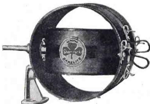
The Shamrock variometer employs pigtail connections from the rotor to the stator coil to eliminate noises and leakage; separate Fahnestock connections for rotor and stator leads permit use as a straight or split variometer; a floating stop allows full 360 degree turn of rotor within stator, thus giving maximum inductive efficiency; guaranteed to tune above 600 meters.
