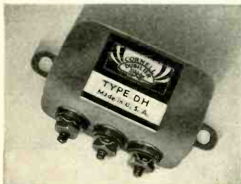
Condenser tested in boiling water
