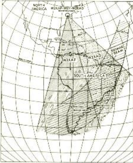
Map illustration of how two powerful beams from the United States will lay down strong signals in South America and Central America.
