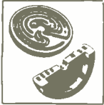
Cross-section shows where the acoustical labyrinth is located. Upper illustration shows the channels in the mould that comprise half the labyrinth. Approved by Radio World Laboratories.
