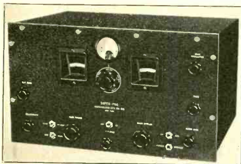
Front view of the receiver in its shield cabinet, and an exposition of the tuning controls. The central shaft operates the coil switch, the left-hand shaft the main condenser gang, and the right-hand shaft the bandspread condenser, which spreads over 20 divisions the band covered by one division of the other.
