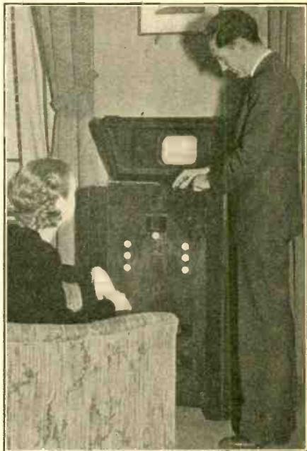
The RCA experimental television receiver, which uses the Kinescope, or reassembler of optical images. The picture is viewed in the opening inside the hinged cover of the console. Both sight and sound are reproduced. Part of speaker grille is seen at bottom.
